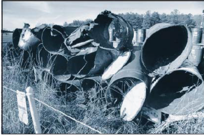
“Figure 1: Empty drums used for storing waste await treatment and disposal at Oak Ridge. These drums corroded prematurely when a 1987 waste-stabilization project failed to follow guidelines for combining waste sludge with cement. K-1417 Drum Storage Yards, Pond Waste Management Project, Oak Ridge, Tennessee. January 10, 1994”
