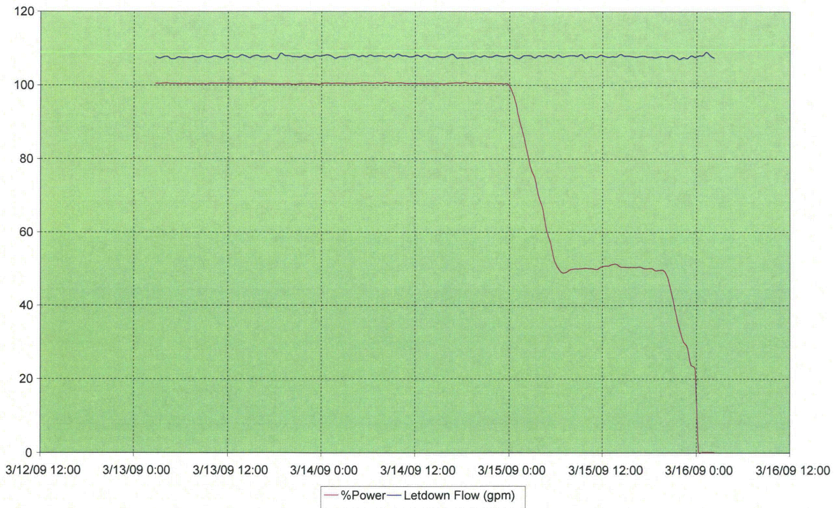
Reactor Power and Clean-up Flow Rate Prior to Turkey Point Unit 3 Iodine (I-131) Spike on 3/16/09
