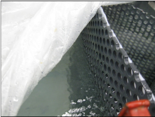
Head of water expected through pre-filter
