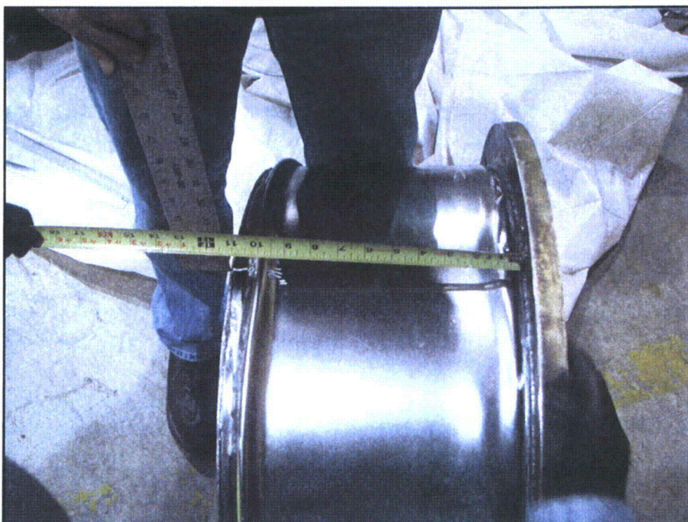
Figure 60 – Foam Crush and Skin Deformation Inspection of End Impact Limiter #2
