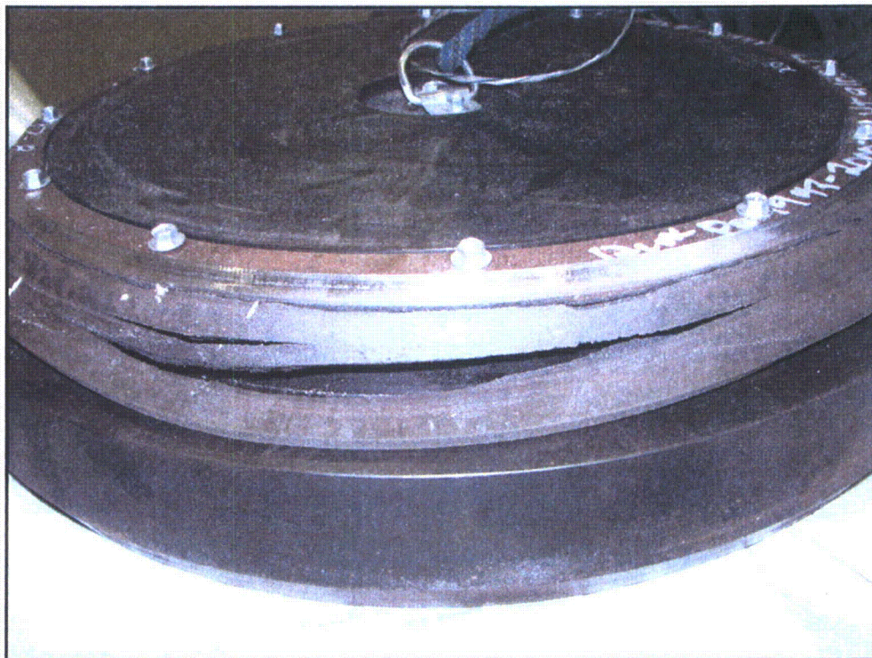
Figure 50 – Bottom End Cap Gasket (with circumferential tear)
