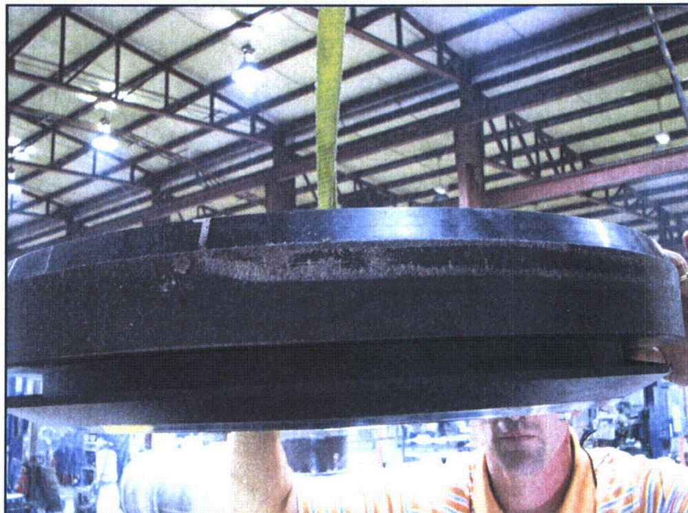
Figure 74 – NS30 #2 Top End Cap with Sand Adhered or Embedded to Outside Diameter
