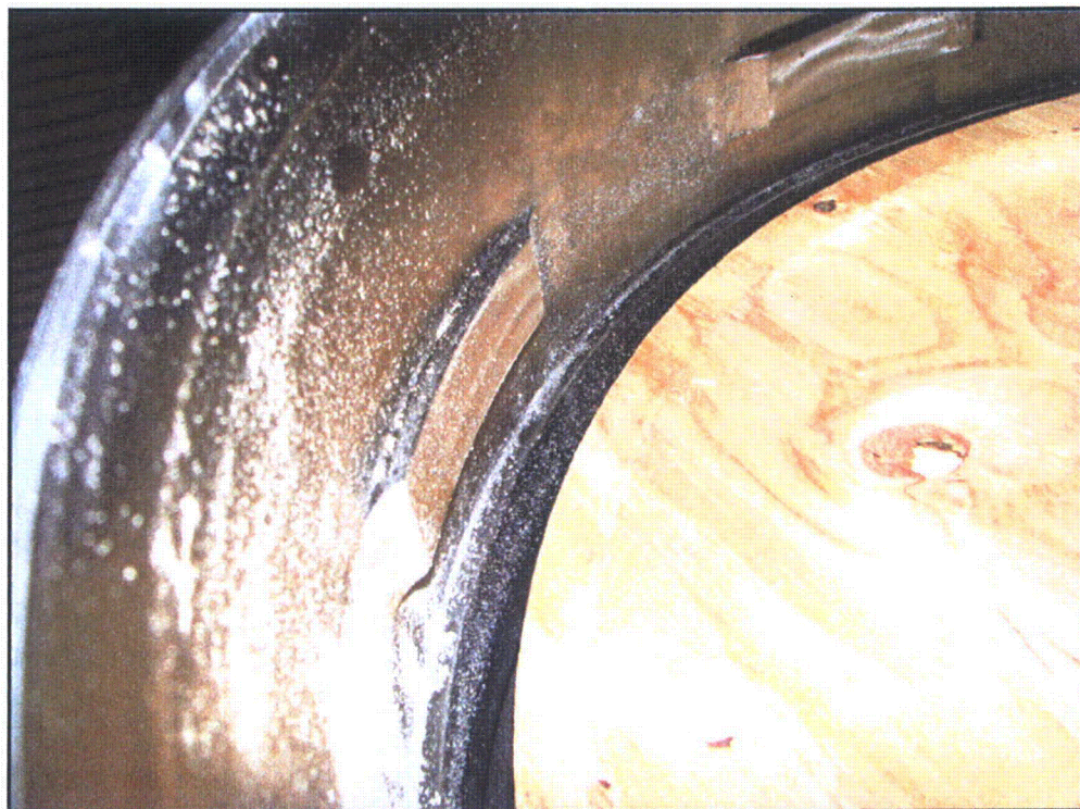
Figure 72 – NS30 #2 Canister Body Flange with Sand Particles Adhered to Lubricant
