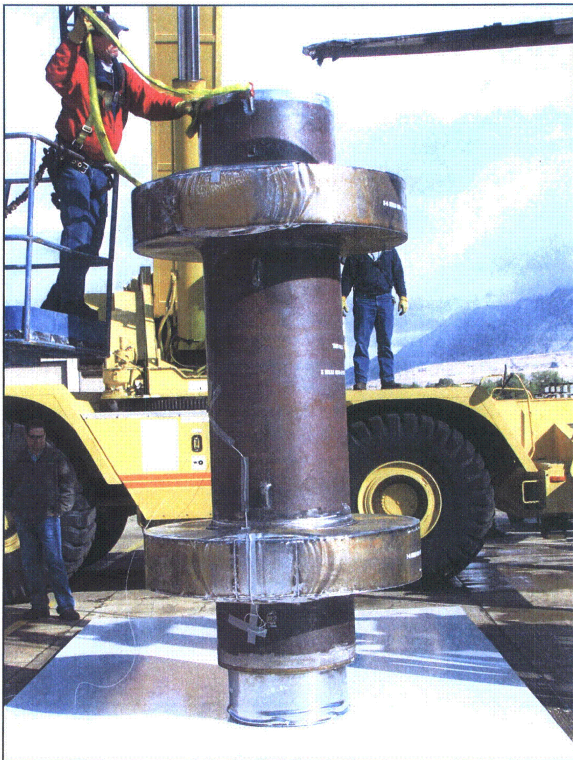
Figure 56 – NS30 #2 Hot End Drop After Impact
