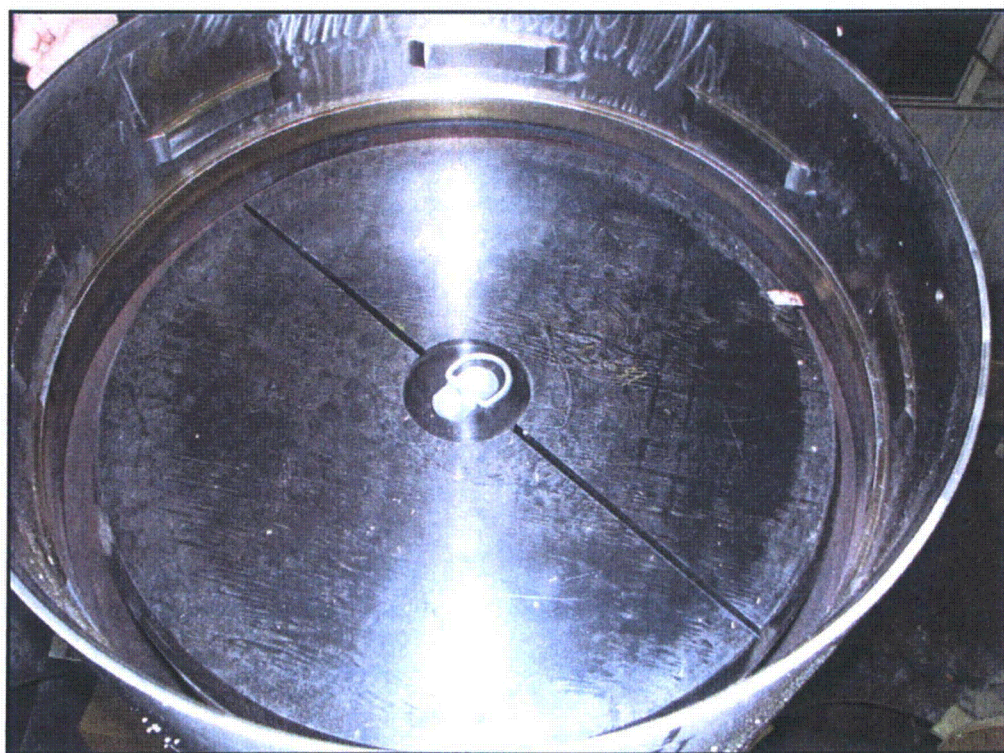
Figure 40 – Undamaged NS30 #1 Top End Cap (containing routed 1/4" deep v-groove defect)
