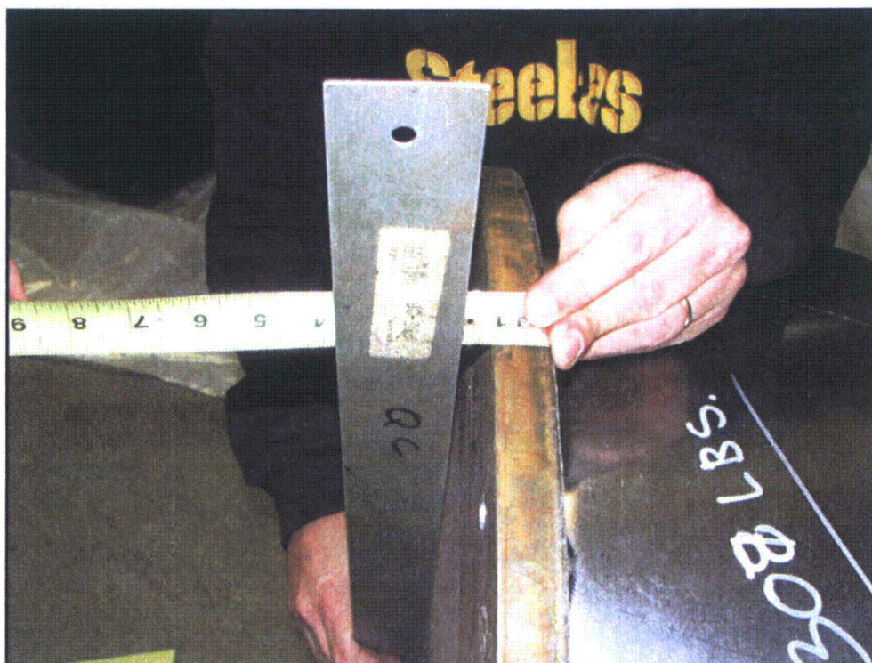
Figure 59 – Measurement of Plastic Deformation of Base Plate on End Impact Limiter #2
