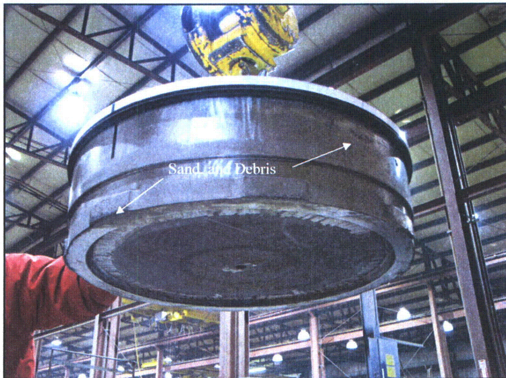
Figure 71 – NS30 #2 Canister Lid with Sand Particles Adhered to Lubricant
