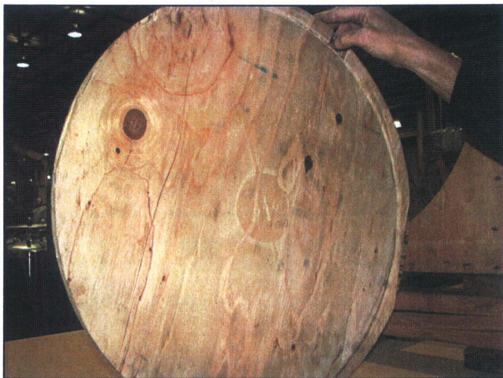
Figure 39 – Deformation of NS30 #1 Plywood Spacer (shield top end cap interface side)
