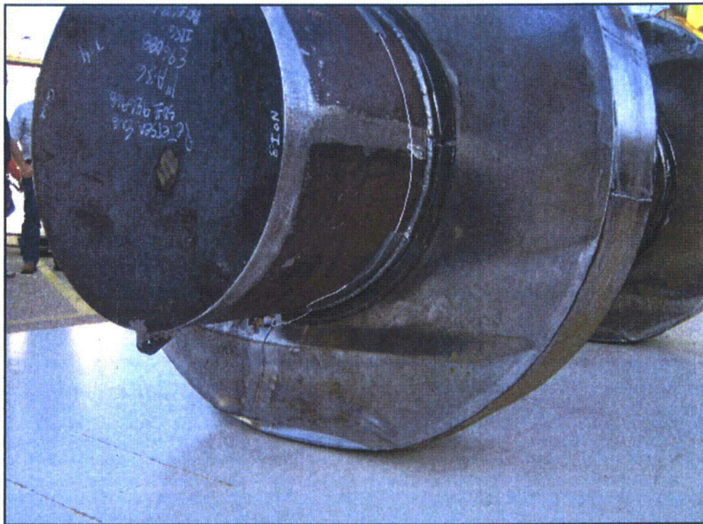
Figure 64 – Left Side (associated with bottom end of NS30 #2) Impact Limiter Deformation
