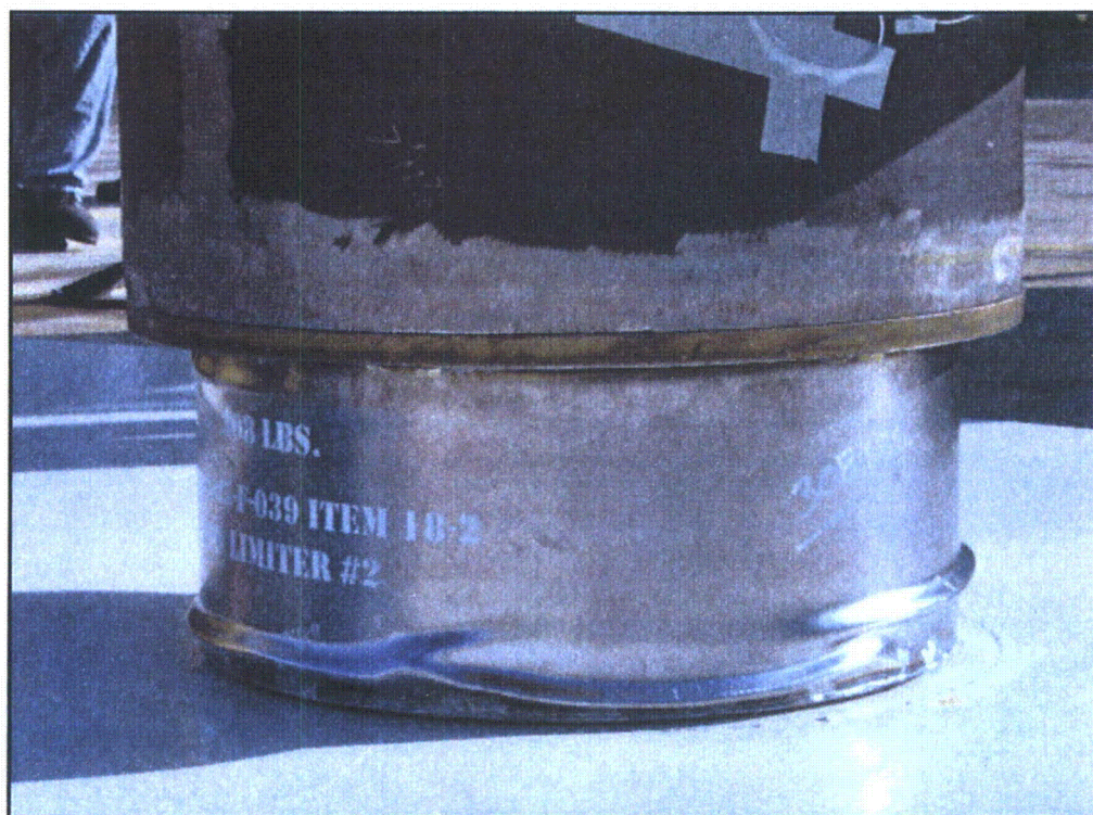
Figure 58 – NS30 #2 Hot End Drop After Impact (close-up #2 of end impact limiter)
