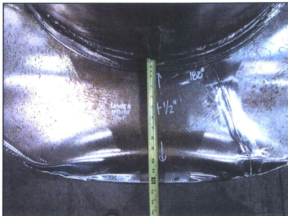
Figure 65 – Measurement of Hot Side Drop Impact Limiter Deformation
