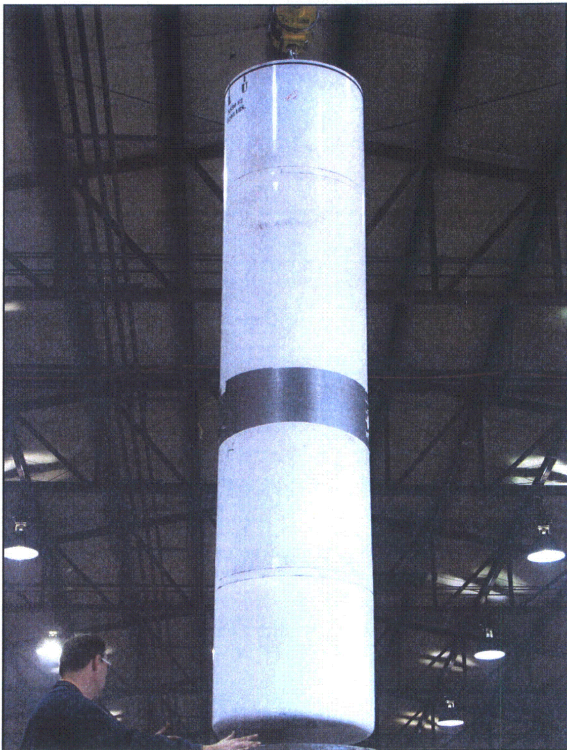
Figure 68 – Removal of NS30 #2 from Test Fixture Following Hot Side Drop Test
