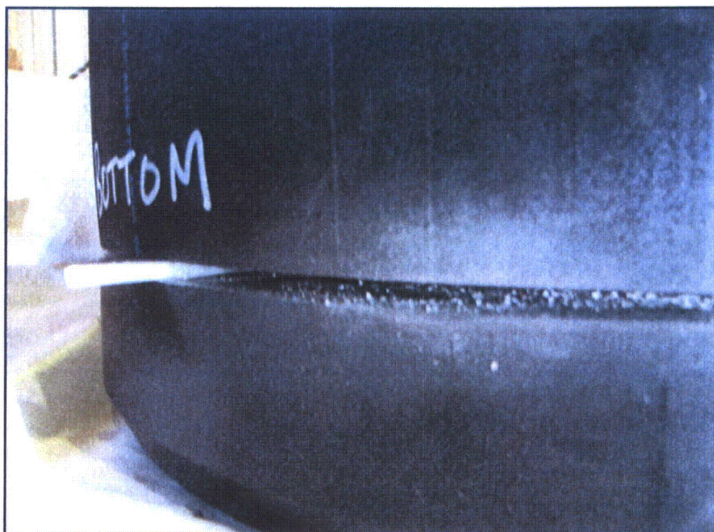
Figure 82 – NS30 #2 Bottom End Cap and Body Pipe Interface (separated by shims to facilitate removal of payload debris that bypassed gasket)
