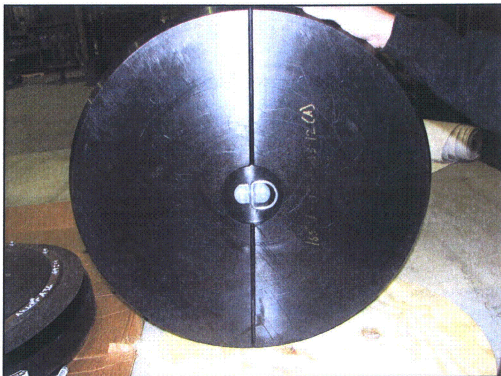
Figure 52 – NS30 #1 Top End Cap Exterior with No Propagation of V-groove Defect
