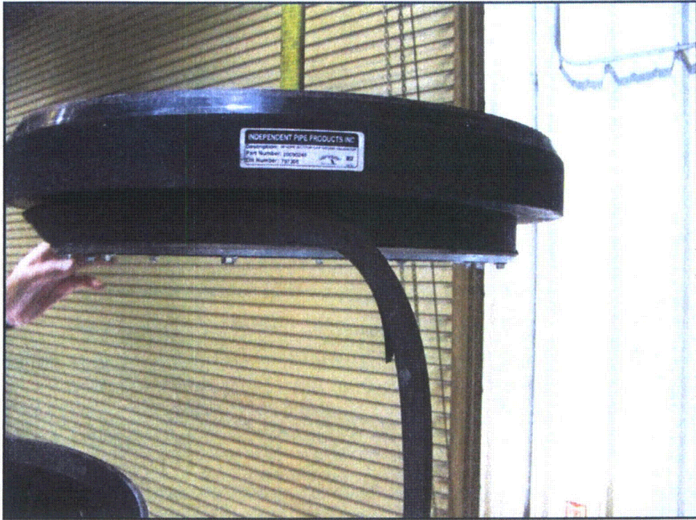
Figure 41 – Removal of NS30 #1 Top End Cap Revealing (gasket tear)
