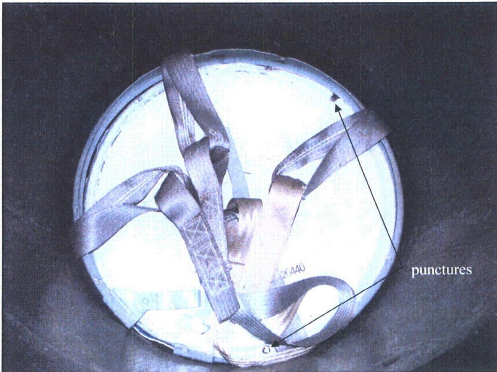
Figure 42 – NS30 #1 Top Payload Drum Inside Shield Body (punctured lid due to interaction with End Cap gasket retainer screws)
