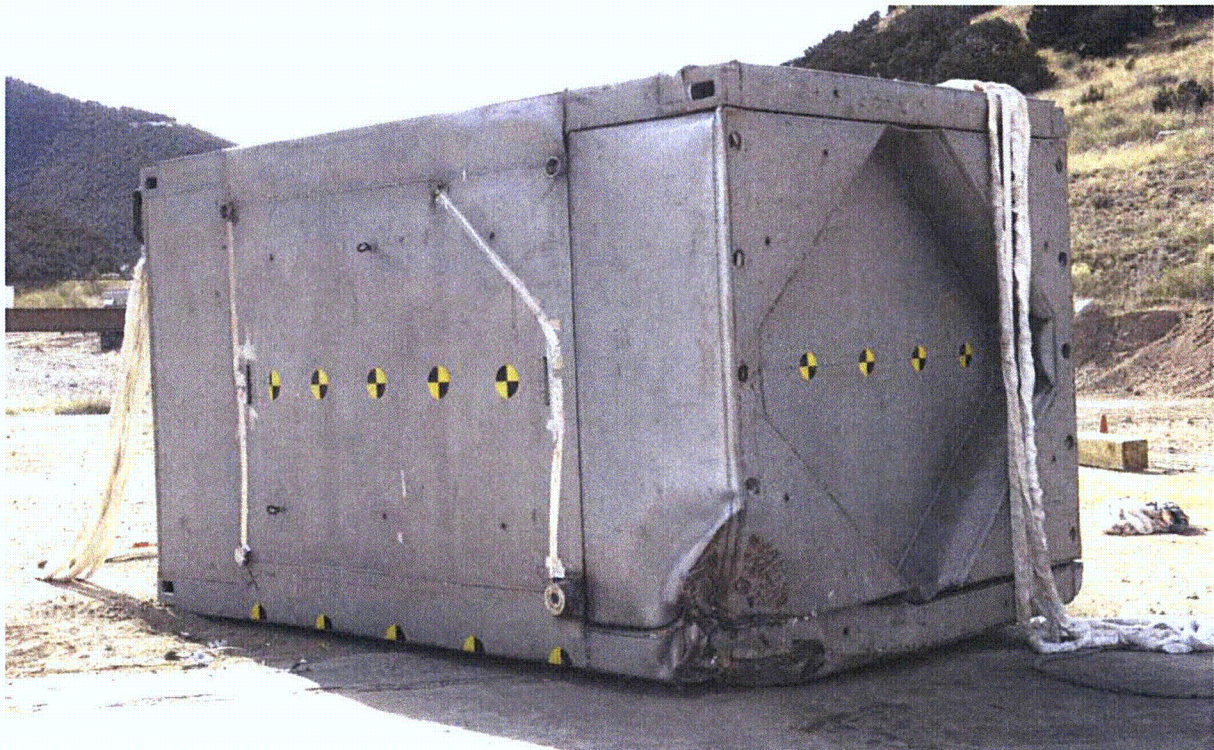
Figure 2.12.3-19 – Test LD4, Typical Deformations
