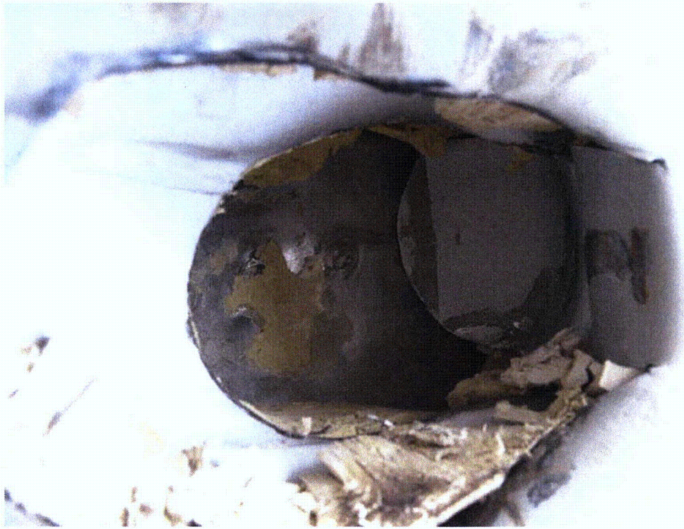
Figure 2.12.3-26 – Test LP1, Close-up of Damage. Bottom of Hole is CSA Outer Structural Sheet
