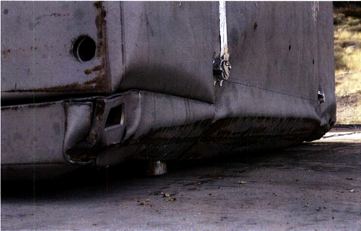
Figure 2.12.3-16 – Test LD5, Typical Deformation
