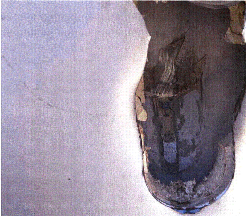
Figure 2.12.3-28 – Test LP2, Close-up of Damage. Bottom of Hole is Puncture-Resistant Plate
