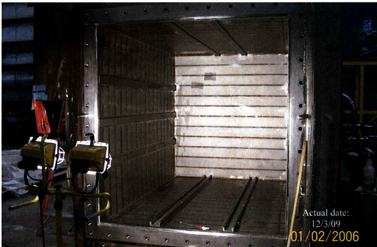
Figure 2.12.6-20 – Payload Cavity with All Contents Removed
