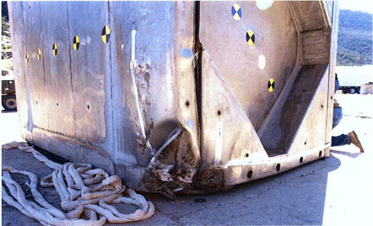
Figure 2.12.6-11 – Test LD91, CG-Over-Corner Free Drop Damage
