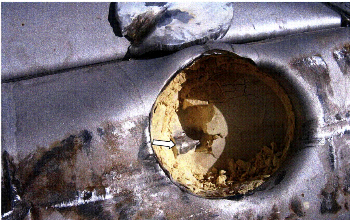
Figure 2.12.3-23 – Test LP4, Close-up of Damage. Note Corner of 16-mm Thick Insulation Protection Box Inside Hole
