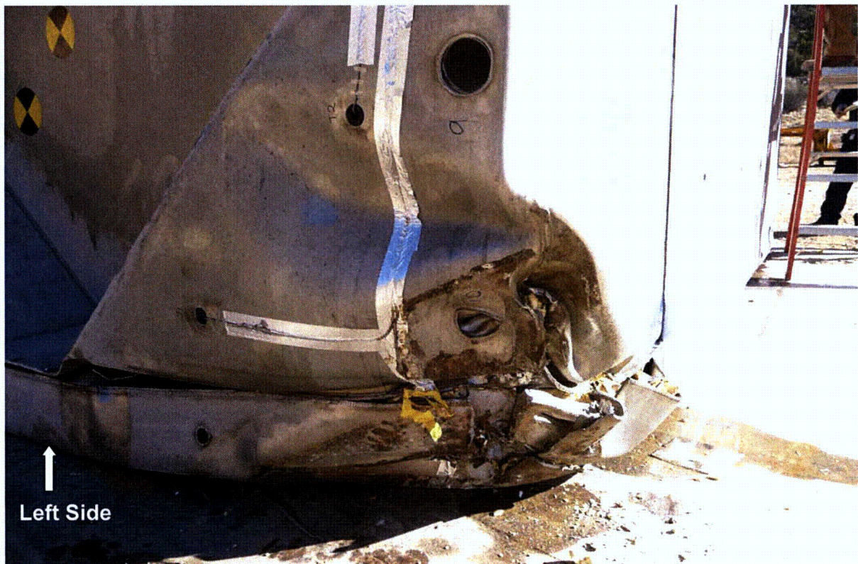
Figure 2.12.6-12 – Test LD91, CG-Over-Corner Free Drop Damage, Detail
