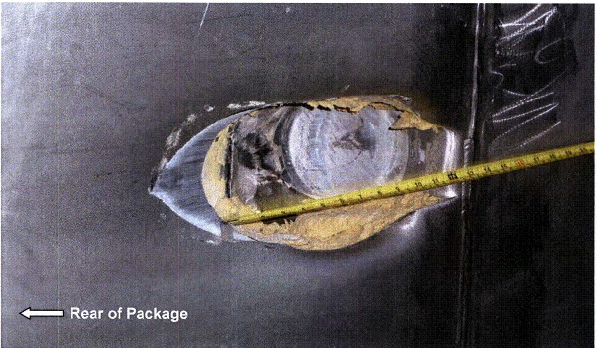
Figure 2.12.6-14 – Test LP92, Puncture on Bottom Wall Damage
