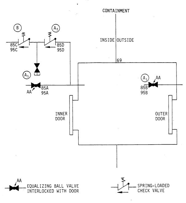
ITEM 69 PERSONNEL AIR LOCK (2) ENTIRE SYSTEM SHOWN IS SEISMIC CLASS I DESIGN
