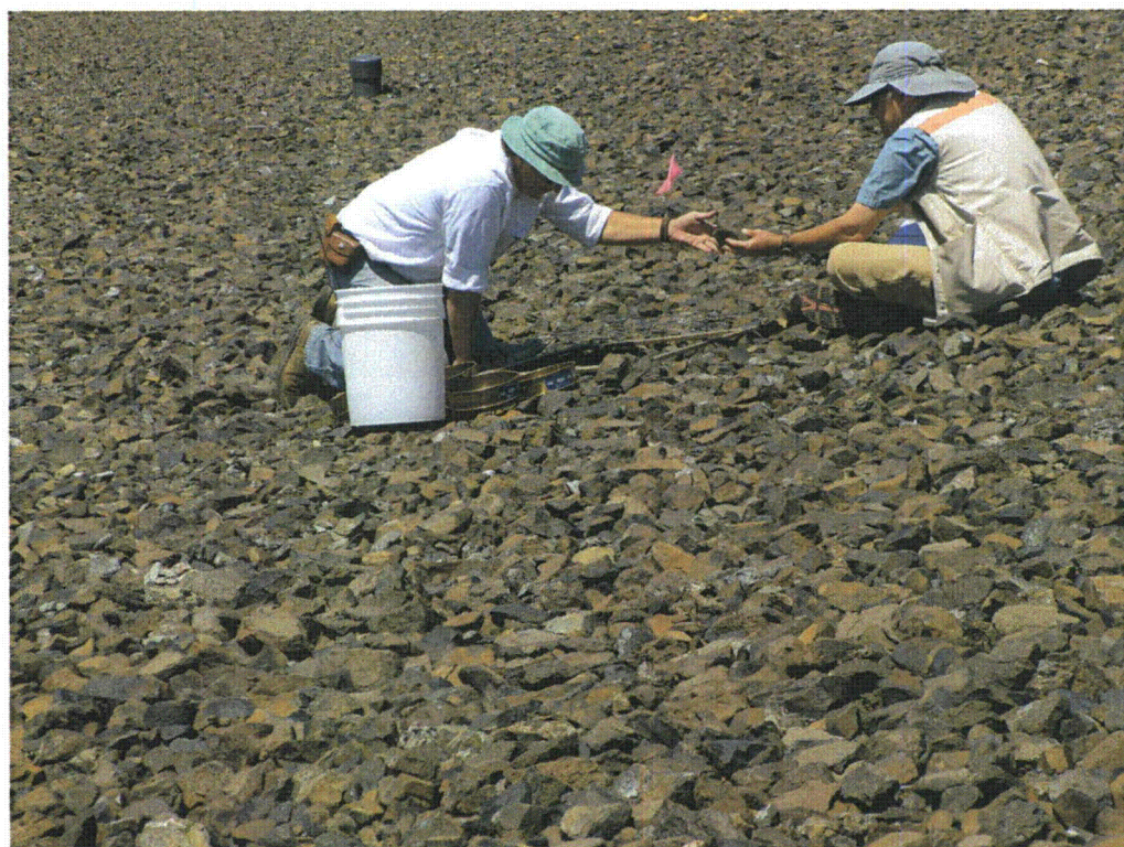
LKV 7/2009. PL-4. Inspectors conducting rock gradation and durability monitoring.
