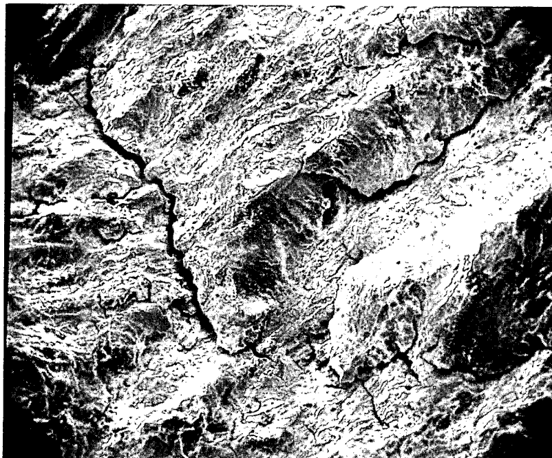
FIGURE 2. SEM of primary fracture surface after some ultrasonic cleaning. Note the secondary cracks.
