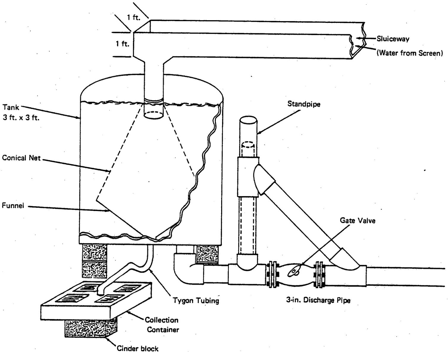
Figure 4-1. Collection device used for fine mesh traveling screen studies at Indian Point.
