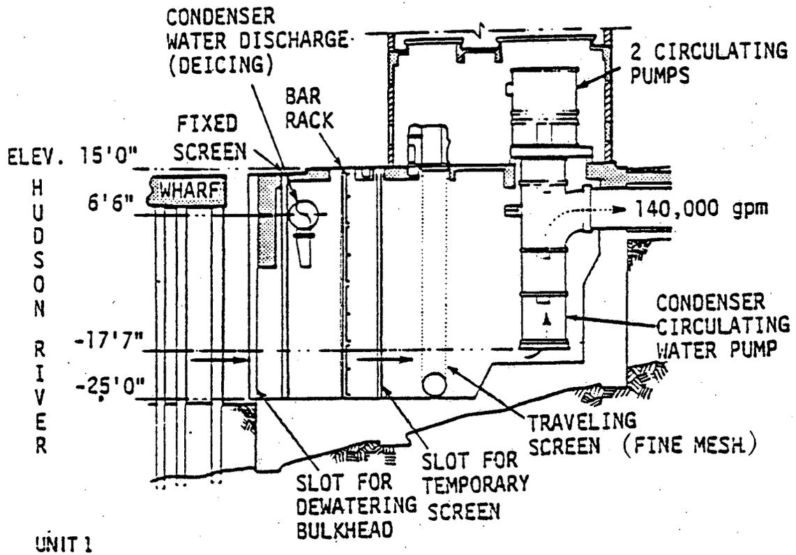
Figure 3-1. Cross-sectional view of Indian Point Generating Station Unit 1 showing location of fine mesh traveling screen. (Source: Con Edison 1977b)
