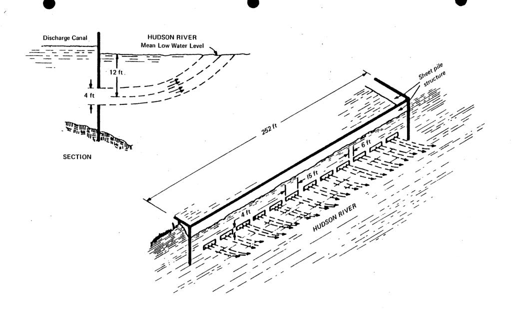
Figure 3-3. Diagrammatic sketch of Indian Point Generating Station discharge structure (from Con Edison 1974).
