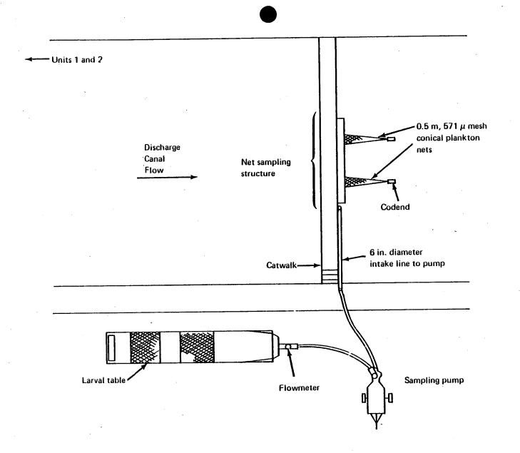
Figure 5-1. Schematic of sampling gear used during the pump-net comparison study (Station D 1), Indian Point Generating Station, 1978.
