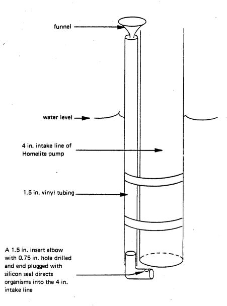
Figure A-1. Vinyl tubing injection system for direct release control experiments conducted at the Indian Point Generating Station, 1978.
