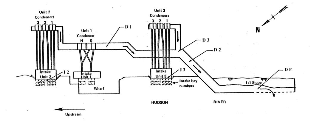
Figure 3-2. Diagram of the Indian Point Generating Station circulating water system showing location of sampling stations (from Con Edison 1977b).
