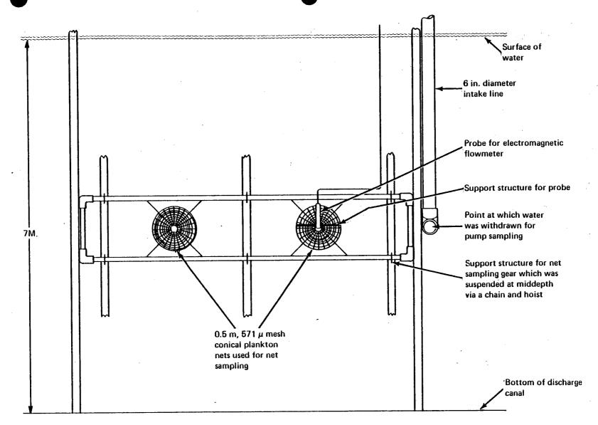
Figure 5-2. Location of net and pump intake pipe used during the pump-net comparison study (Station D 1), Indian Point Generating Station, 1978.
