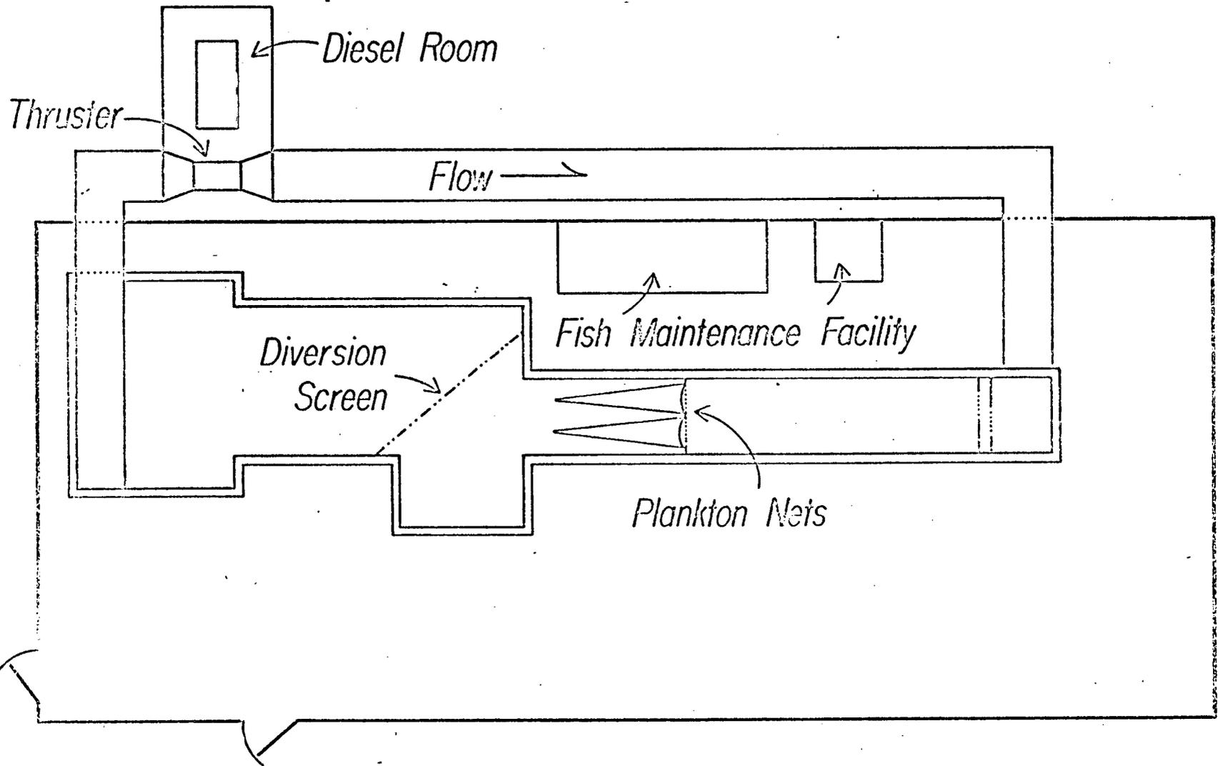
Figure 1. Plan view of the Consolidated Edison experimental flume located at Alden Research Laboratories, Holden, Massachusetts.
