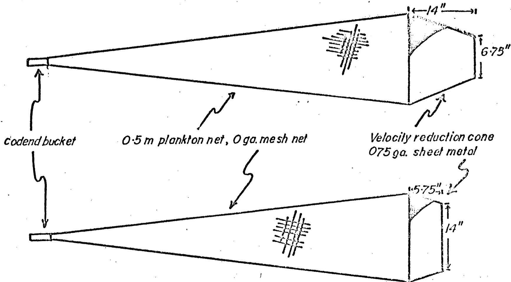
Figure 2. Schematic diagram of plankton nets equipped with velocity reduction cones of 14" and 6.75" mouth openings.
