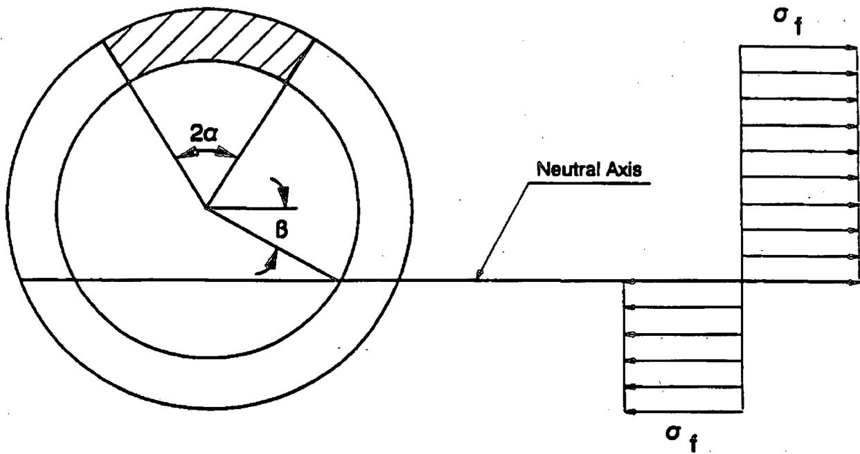
Figure 5-1 Fully Plastic Stress Distribution
