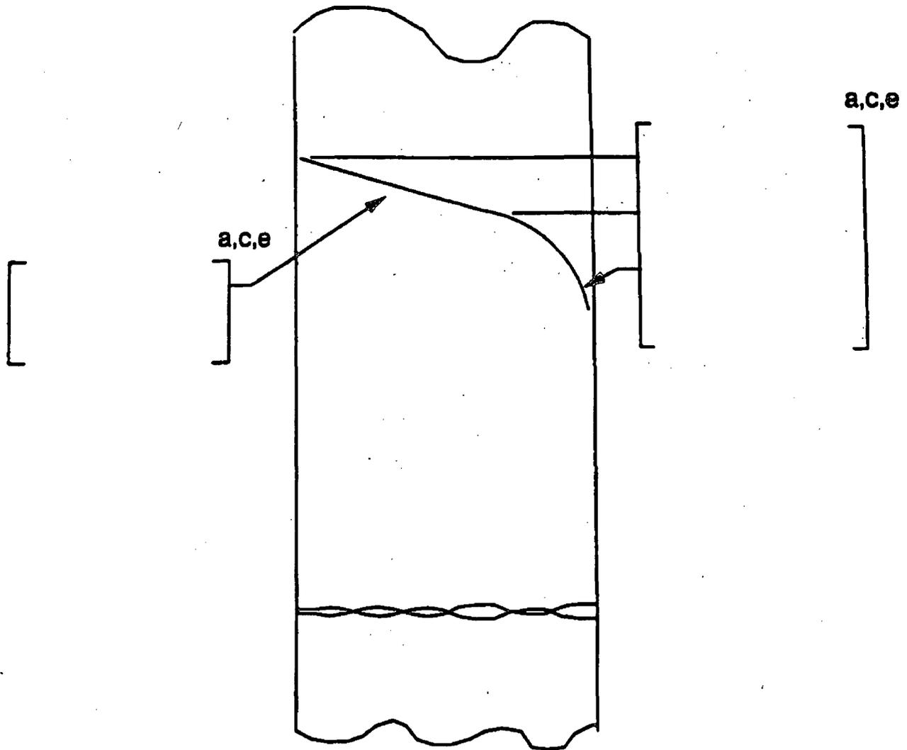
**Figure 5-4 Idealized Pressure Drop Profile Through a Postulated Crack**
