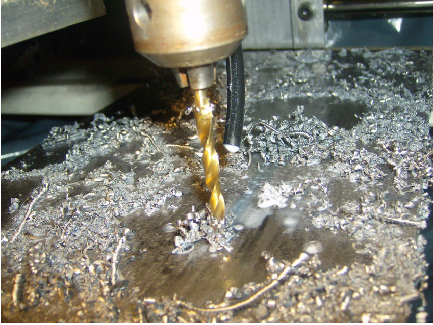
Swarf produced by drilling
