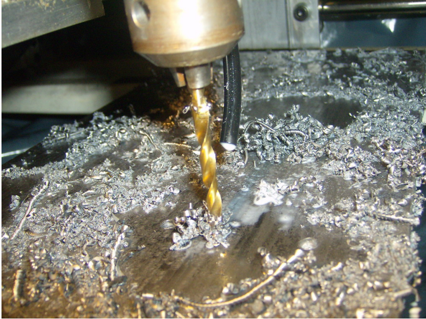
Swarf produced by drilling
