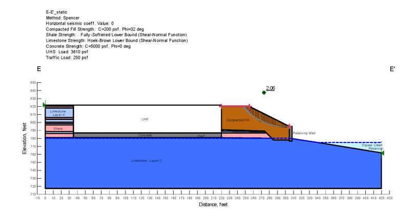
Figure 2.5.5-210 Static Stability Analysis- Cross Section E-E'
