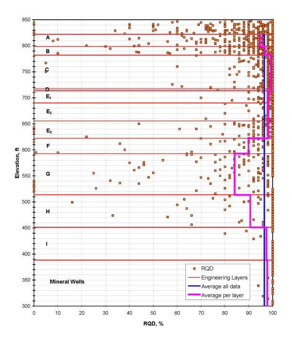
Figure 2.5.4-240 Rock Quality Designation vs. Elevation
