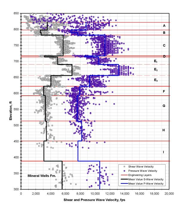
Figure 2.5.4-239 In-Situ S- and P-Wave Velocity vs. Elevation
