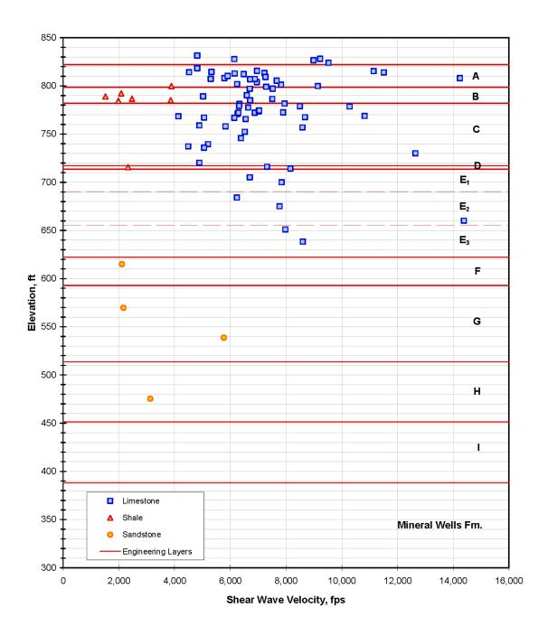
Figure 2.5.4-238 Laboratory-Based Shear Wave Velocity vs. Elevation
