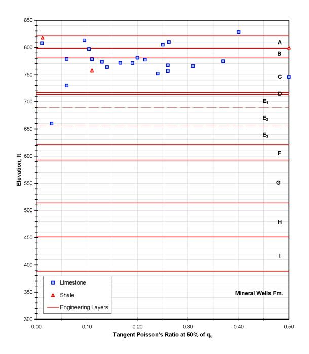
Figure 2.5.4-230 Tangent Poisson's Ratio from Unconfined Compression Tests vs. Elevation
