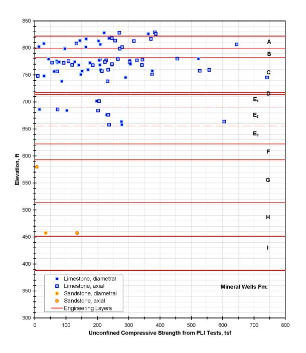
Figure 2.5.4-229 Estimated Unconfined Compressive Strength from Point Load Index Tests vs. Elevation
