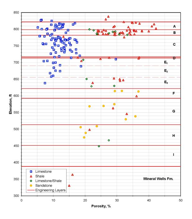
Figure 2.5.4-221 Calculated Porosity vs. Elevation
