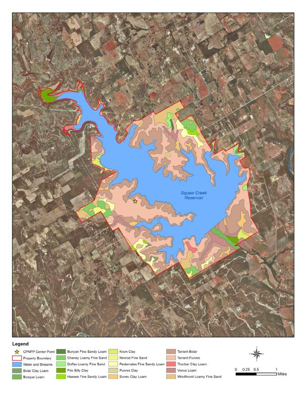
Figure 2.4.12-211 Soil Types at CPNPP Site
