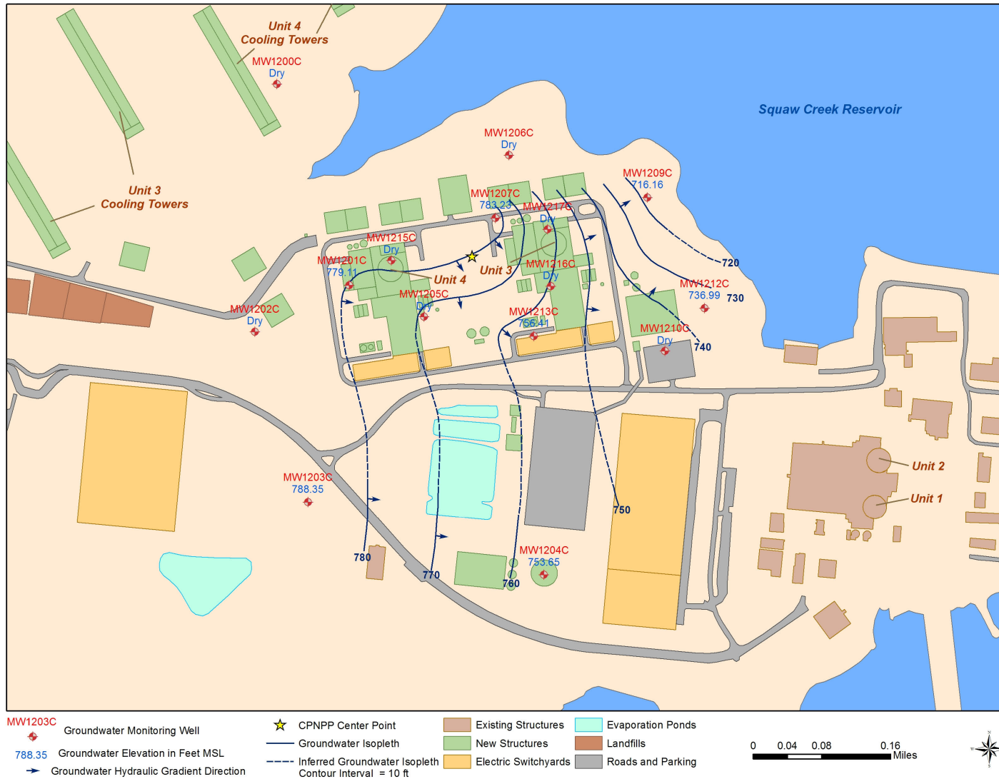
Figure 2.4.12-210 Potentiometric Surface Maps (Sheet 10 of 12)
