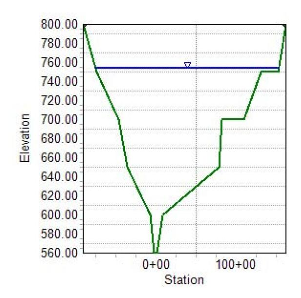
Figure 2.4.4-203 Water Surface Elevation at Brazos River - Paluxy River Confluence Cross Section for Hydrologic Domino Type Dam Failures Coincident with PMF
