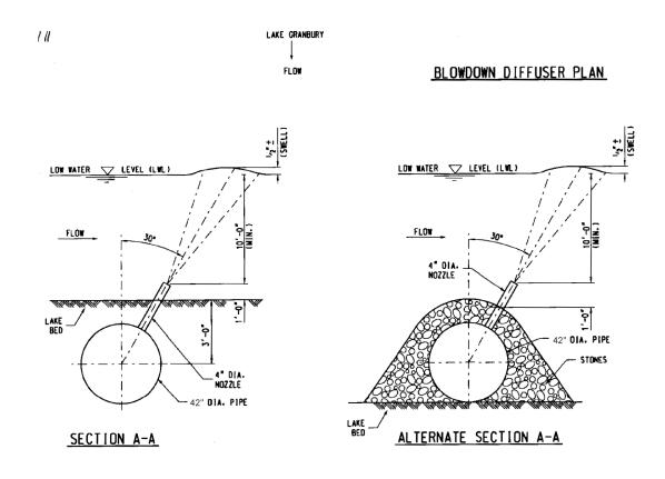
Figure 9.4-4 Proposed Multi-Fort Diffuser Discharge System
