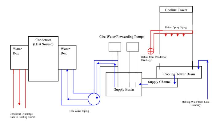
Figure 9.4-3 Proposed Cooling Water System, Closed Cycle Mechanical Draft (Wet) Cooling Tower
