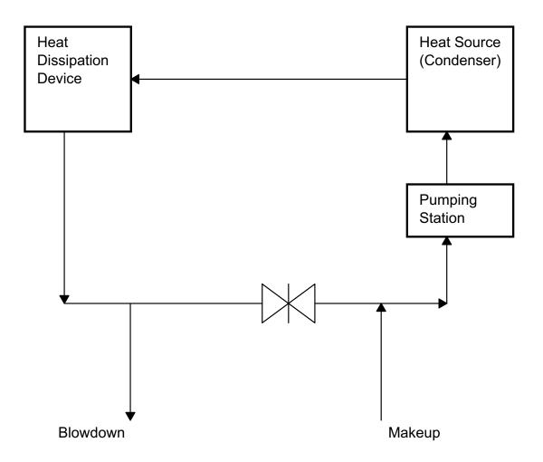
Figure 9.4-1 Alternative Cooling System, Typical Closed Cycle System
