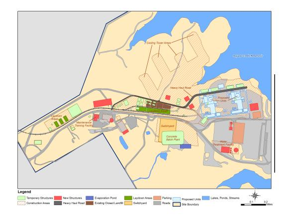
Figure 4.1-1 Detailed Site Plot plan with Construction Laydown Areas
