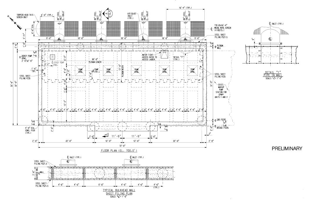
Figure 3.4-4 Makeup Water Intake Structure
