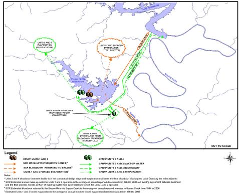
Figure 2.3-30 CPNPP Units 1 and 2 and 3 and 4 Simplified Water Use Diagram
