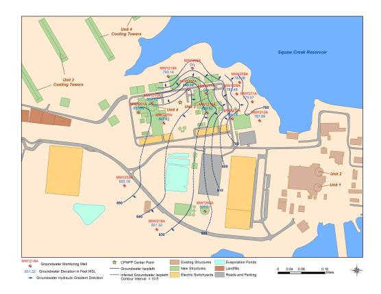
Figure 2.3-27 June 2007 Potentiometric Surface Map (A-Wells)(Sheet 3 of 12)
