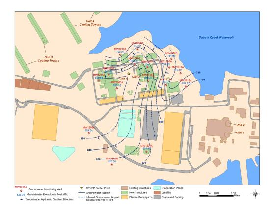
Figure 2.3-27 September 2007 Potentiometric Surface Map (A-Wells)(Sheet 4 of 12)
