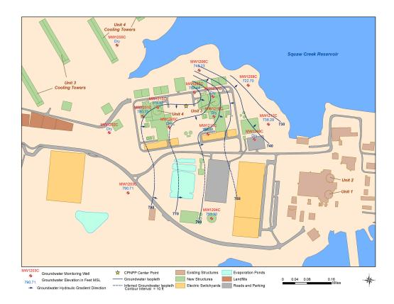
Figure 2.3-27 June 2007 Potentiometric Surface Map (C-Wells)(Sheet 11 of 12)
