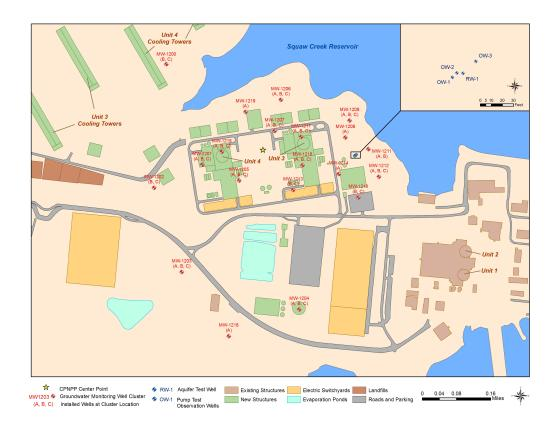
Figure 2.3-26 Groundwater Monitoring Well Location Map
