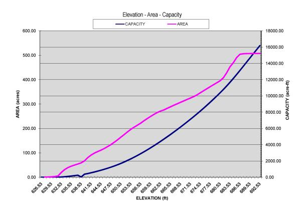
Figure 2.3-14 Lower Lake Granbury Elevation - Area - Capacity Curve
