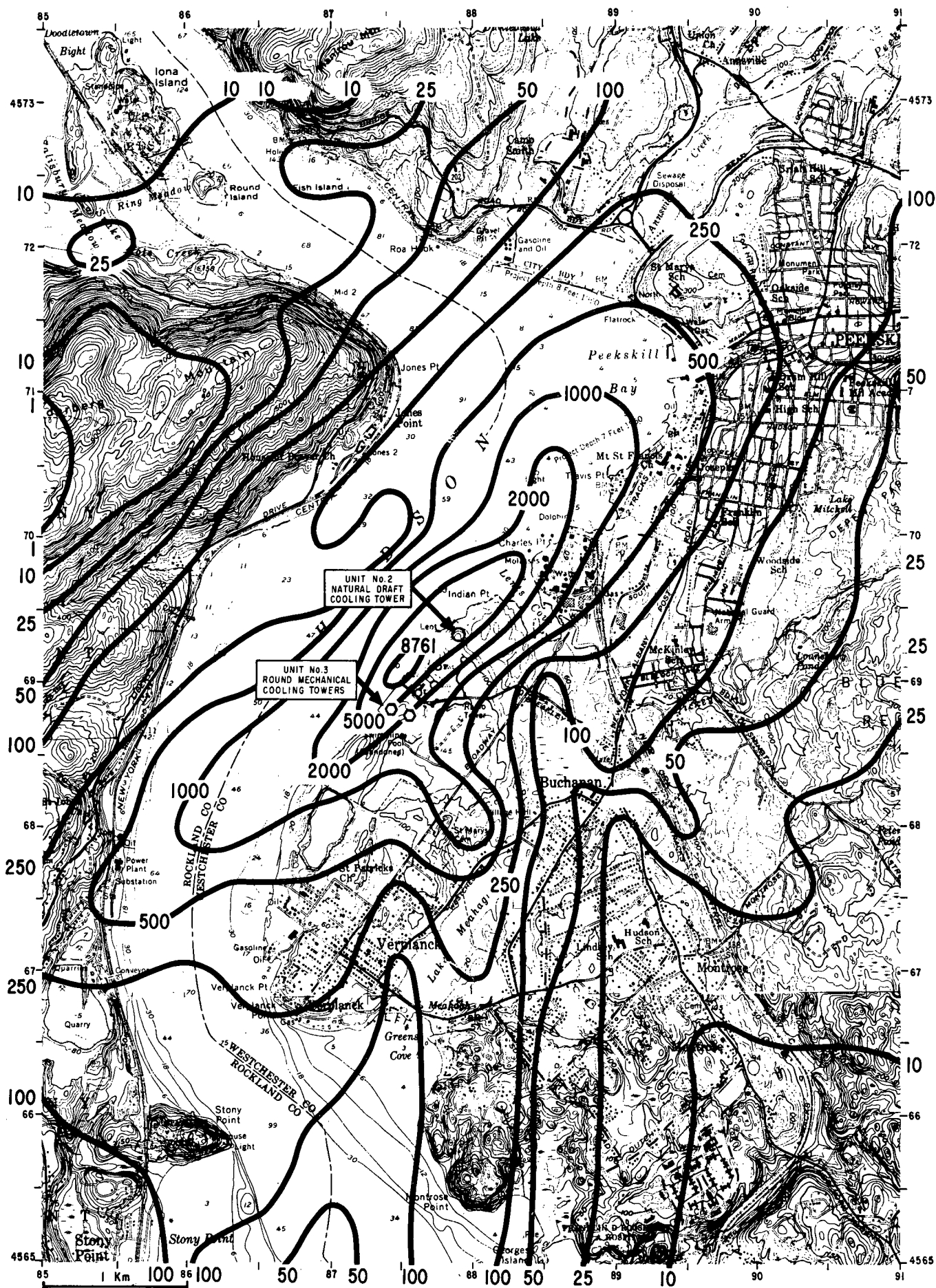
FIGURE 5.1.7 ACCUMULATED SALT DRIFT DEPOSITS \text{Kg/Km}^2/\text{Mo} , AUGUST 1974 ROUND WET MECHANICAL DRAFT COOLING TOWERS
