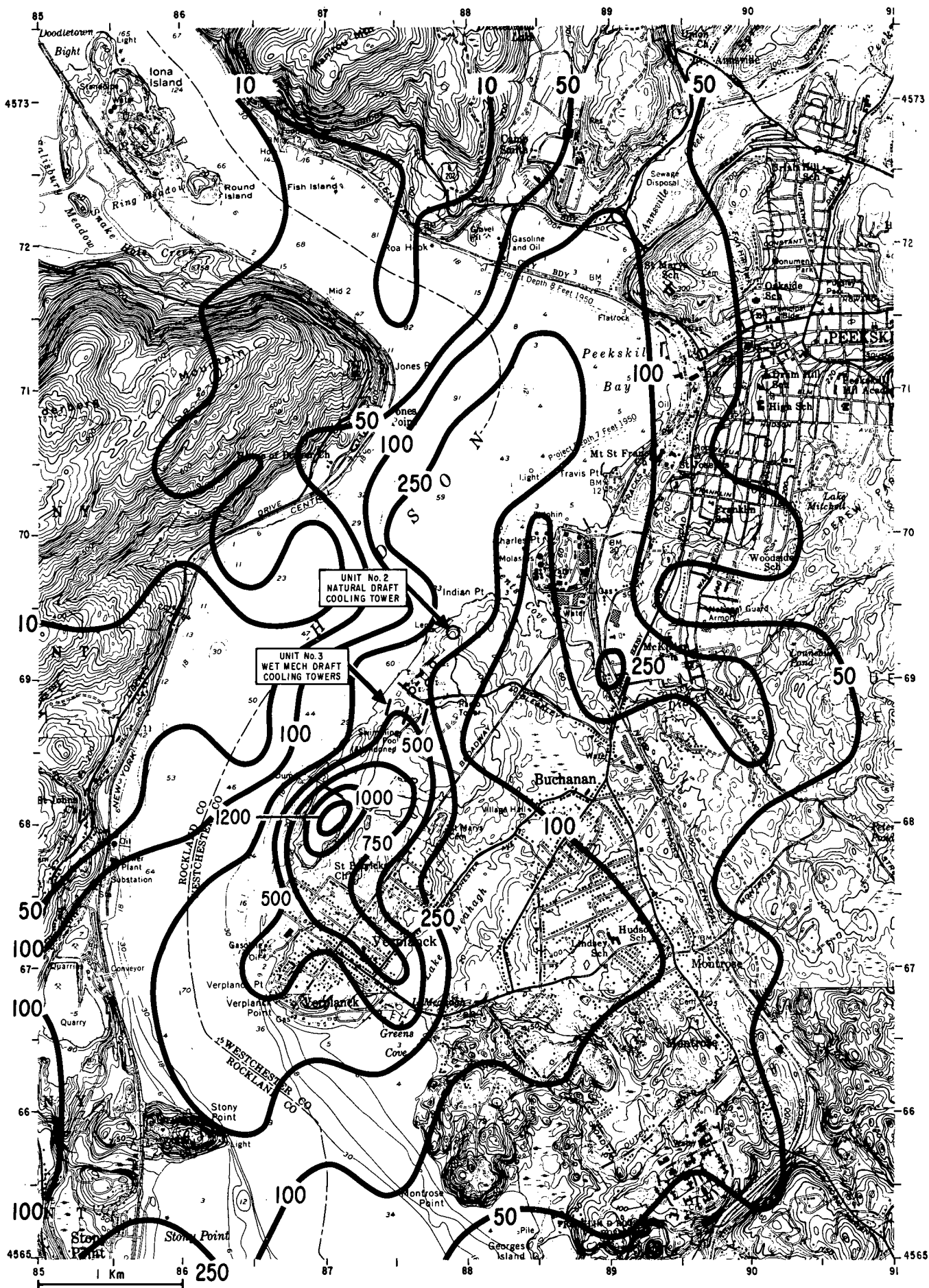
FIGURE 5.1.3 ACCUMULATED SALT DRIFT DEPOSITS \text{Kg/Km}^2/\text{Mo} , FEBRUARY 1974 WET MECHANICAL DRAFT COOLING TOWERS
