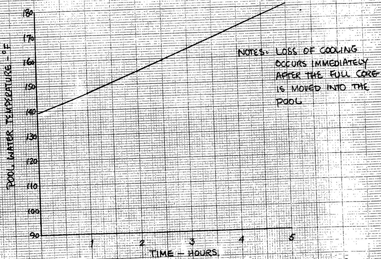
FIG. C-5. TRANSIENT HEAT-UP OF POOL WATER TEMPERATURE WITH NO COOLING FOR THE ABNORMAL CASE.
