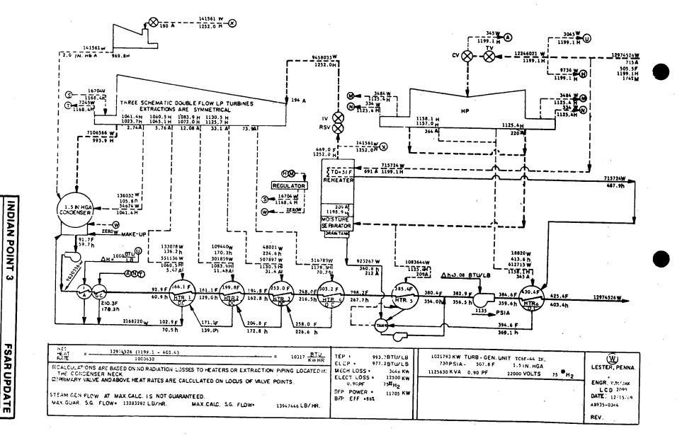
1000630 KW NET LOAD HEAT BALANCE INITIAL GUARANTEE AT 715A INLET
