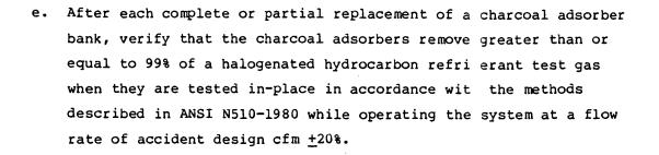
With the efficiencies of the HEPA filters and charcoal adsorbers as specified, further assurance is provided that the resulting doses will be less than the allowable levels stated in Criterion 19 of the General Design Criteria for Nuclear Power Plants, Appendix A to 10CFR Part 50.
