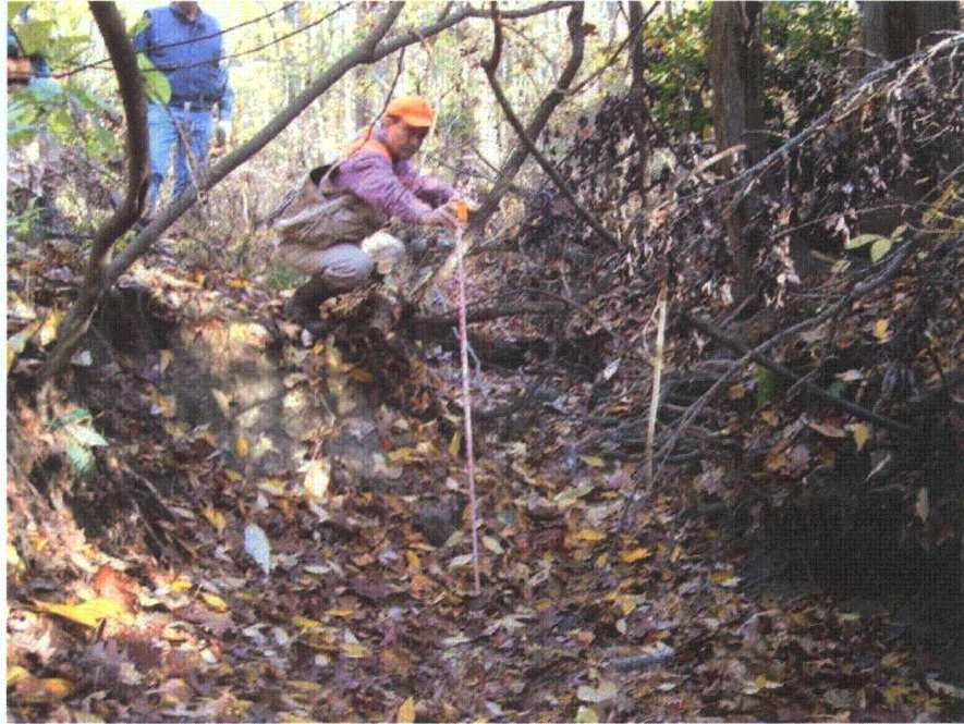
Photo 4-9 Views of Woodland Branch showing degree of incision and a depositional feature below an exposed bank.
