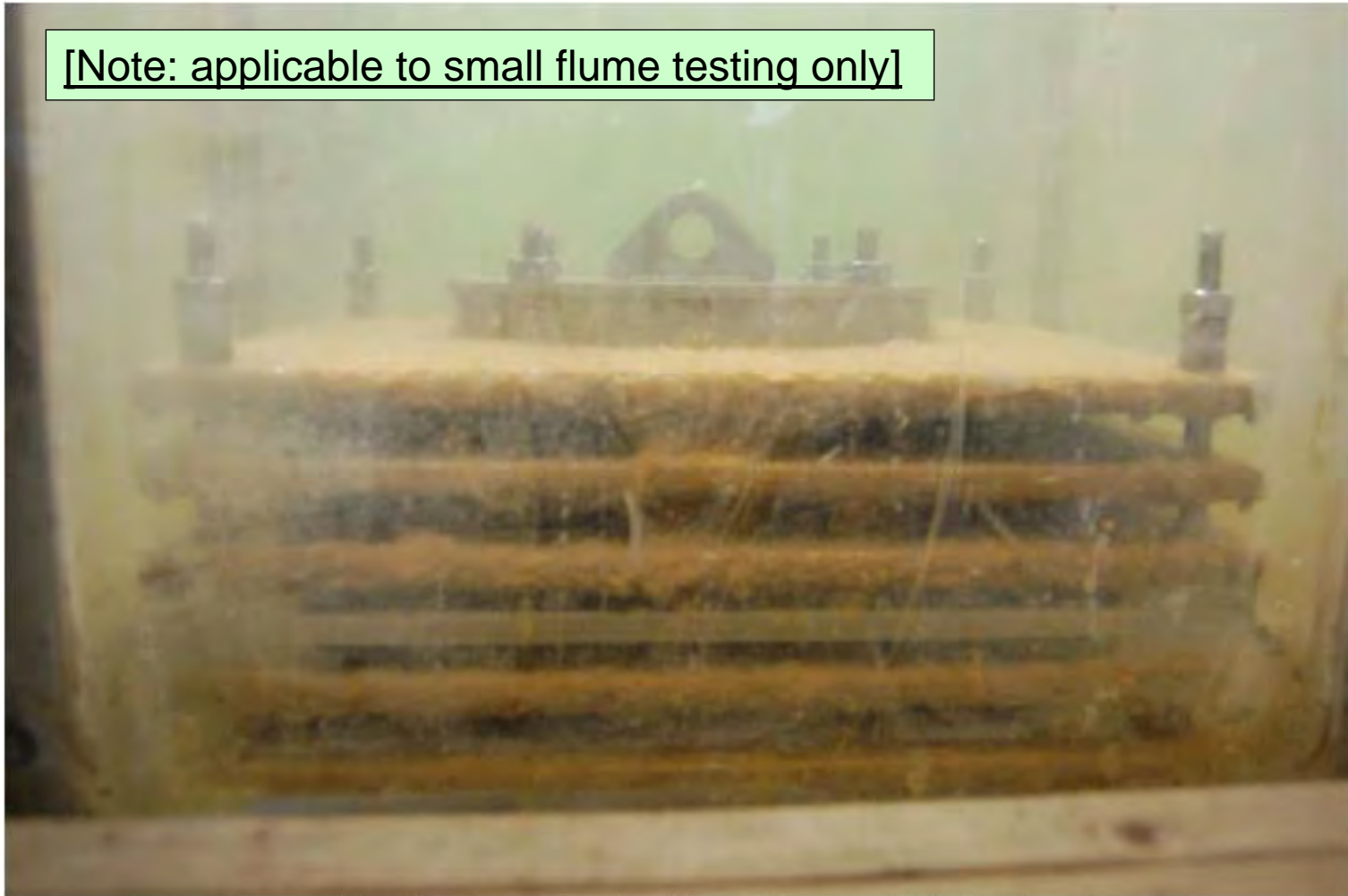
Figure 11. Fine fiber on strainer after smalls introduction
