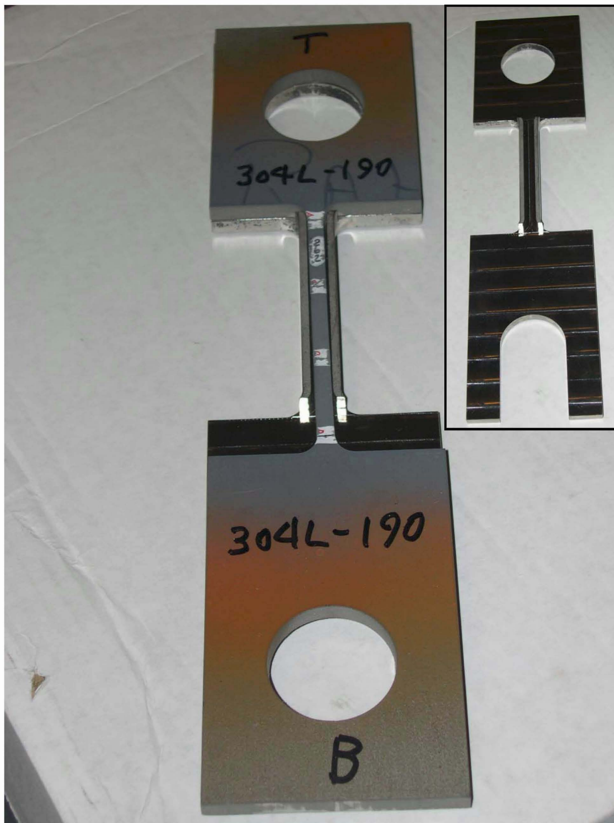
Figure 52. D-2-2 cradle holding an impacted test specimen (upper right insert is of cradle alone).
