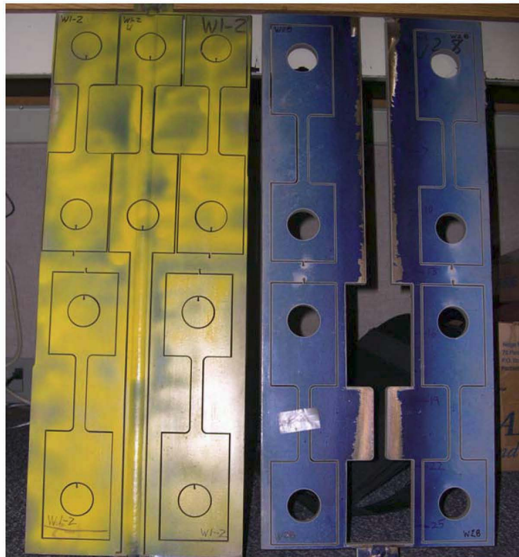
Figure 16. Both 304L and 316L 1/2-inch thick welded plates showing welded material blanks (attached to impact test specimens, which were later removed).
