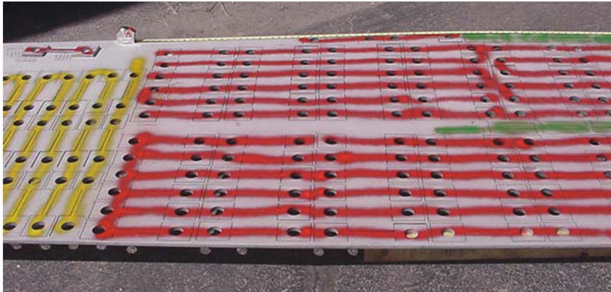
Figure 38. Initial 304L plate water jet cut and test specimens painted.
