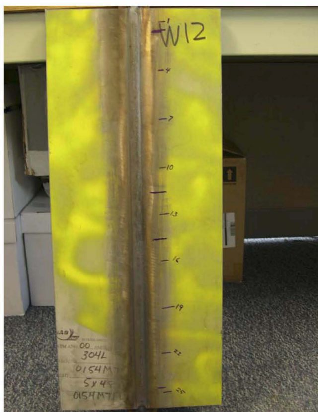
Figure 12. Markings showing where radiographs were taken on the welded plate.
