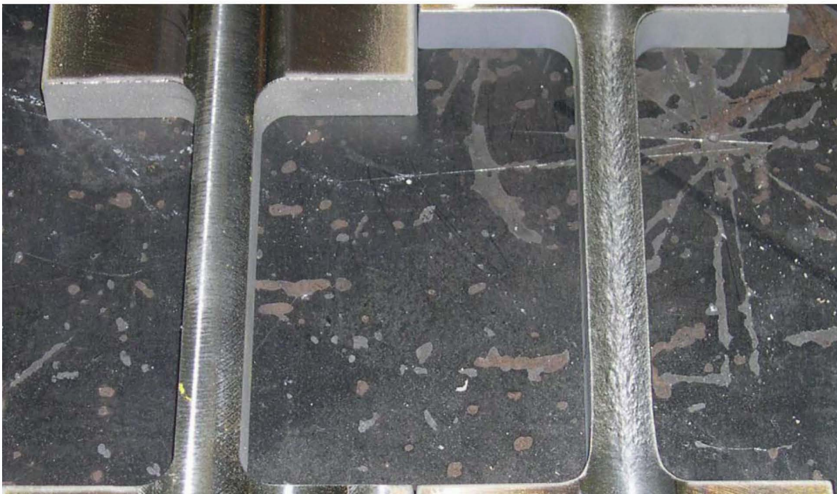
Figure 59. 'Orange peel' effect in welded material impact test specimen (right).
