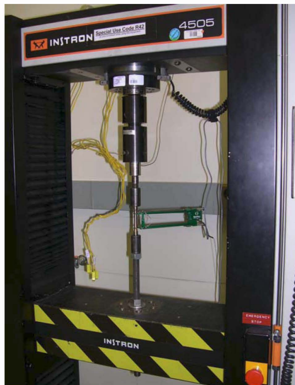
Figure 23. Room temperature tensile testing setup at IRC.
