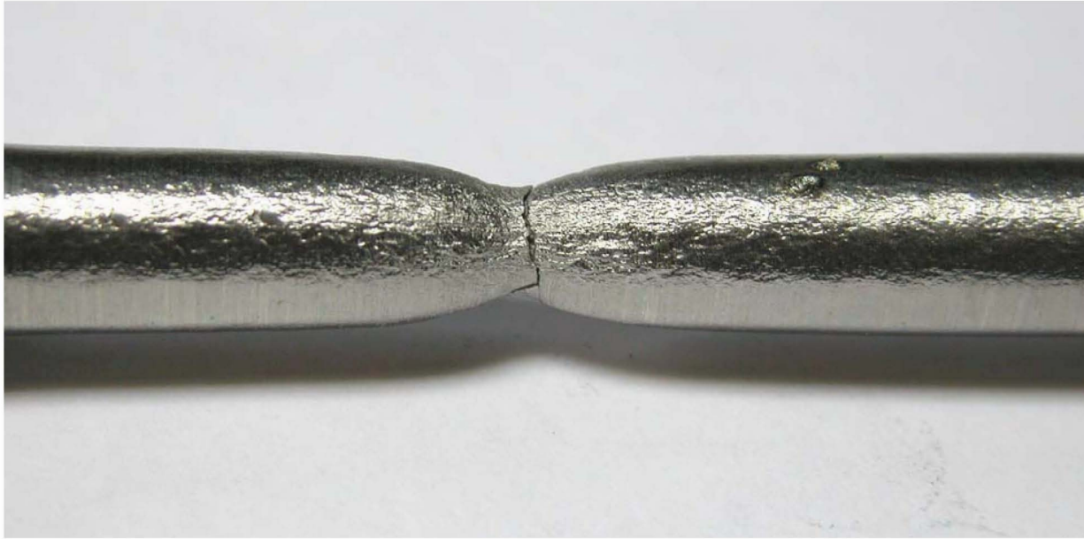
Figure 29. Welded quasi-static tensile test specimen showing 'orange peel' effect.
