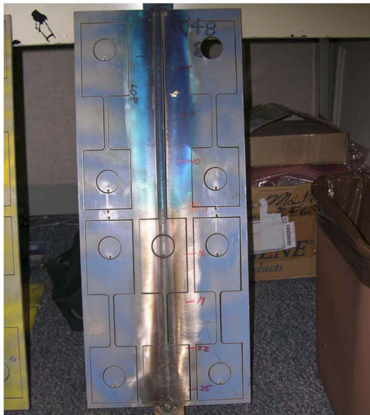
Figure 17. 316L 1/4-inch thick plate showing welded material blank cut from the plate (also attached to impact test specimen, which was later removed).
