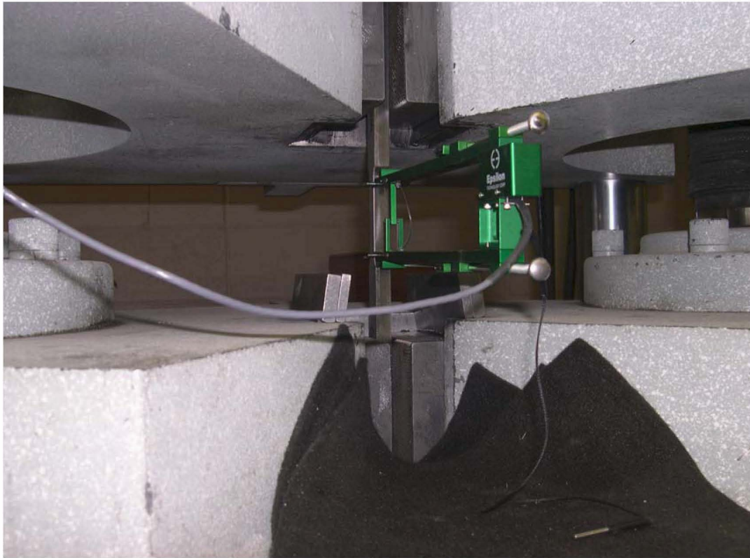
Figure 21. Close-up of inserted test specimen with extensometer attached.
