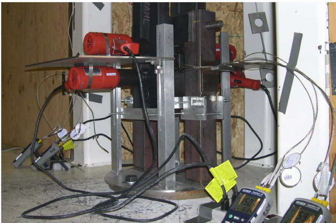
Figure 53. Temperature baseline testing setup showing four heat guns in position.
