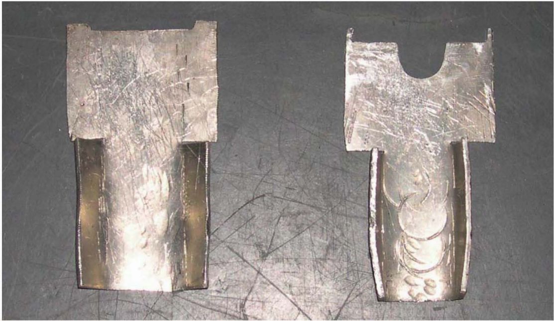
Figure 51. Heat shields for all test specimens (left) except D-2-2 test specimens at 600 °F (right).
