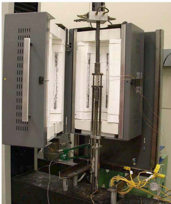
Figure 24. Elevated temperature tensile testing setup with furnace door open.
