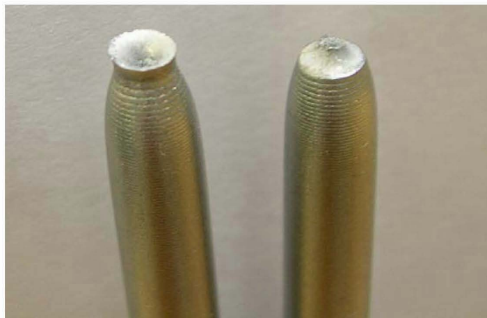
Figure 28. 'Cup and cone' type failure at fracture point.
