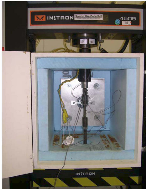
Figure 22. Cold (-20°F) temperature tensile testing setup.
