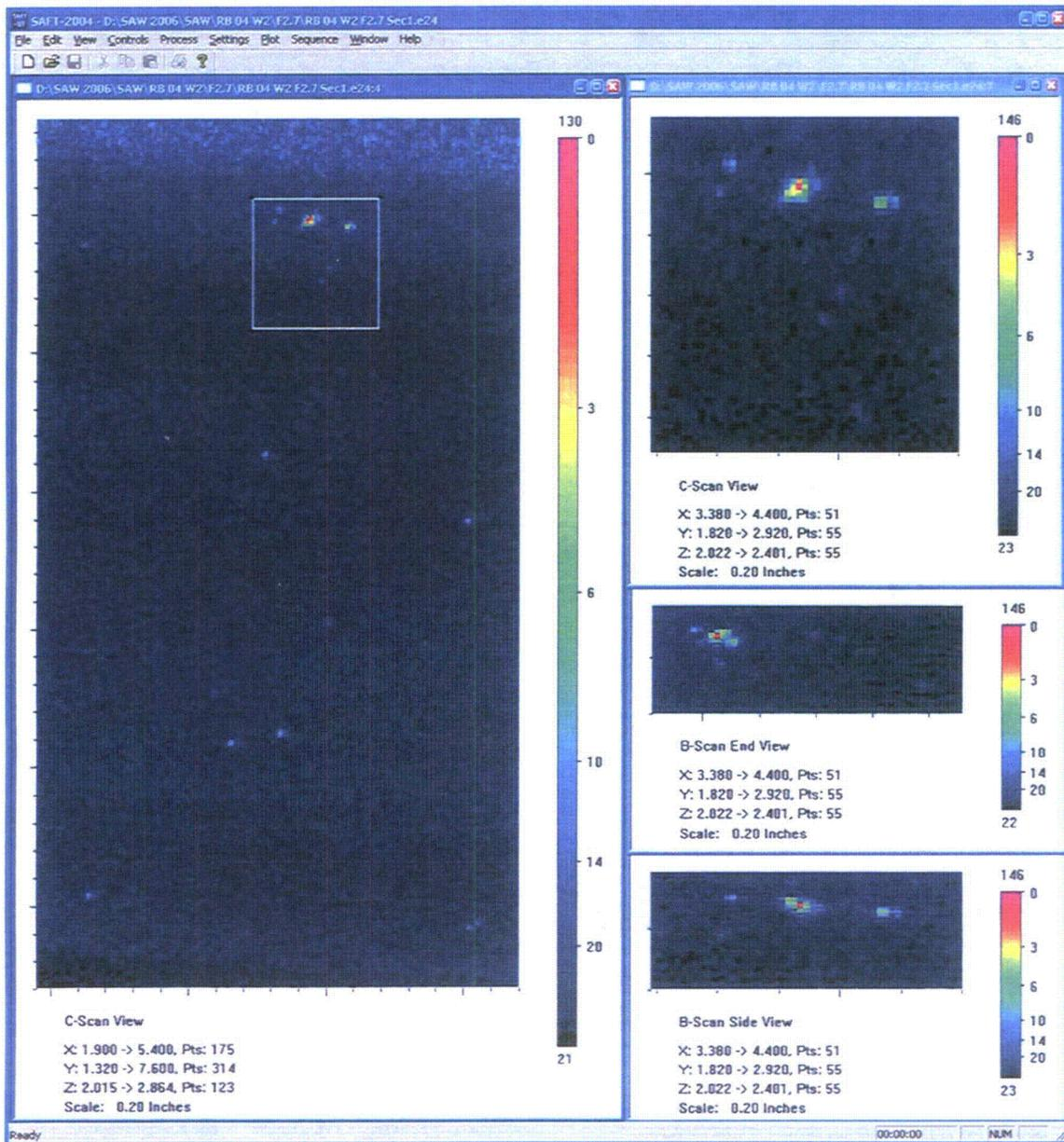
Figure A.3.c F2.7 Immersion Testing Images of Small Fabrication Flaw: *RB3A*. This figure shows the same material and flaw as the previous figures. Here the flaw is resolved to a through-wall size of 1.5 mm.
