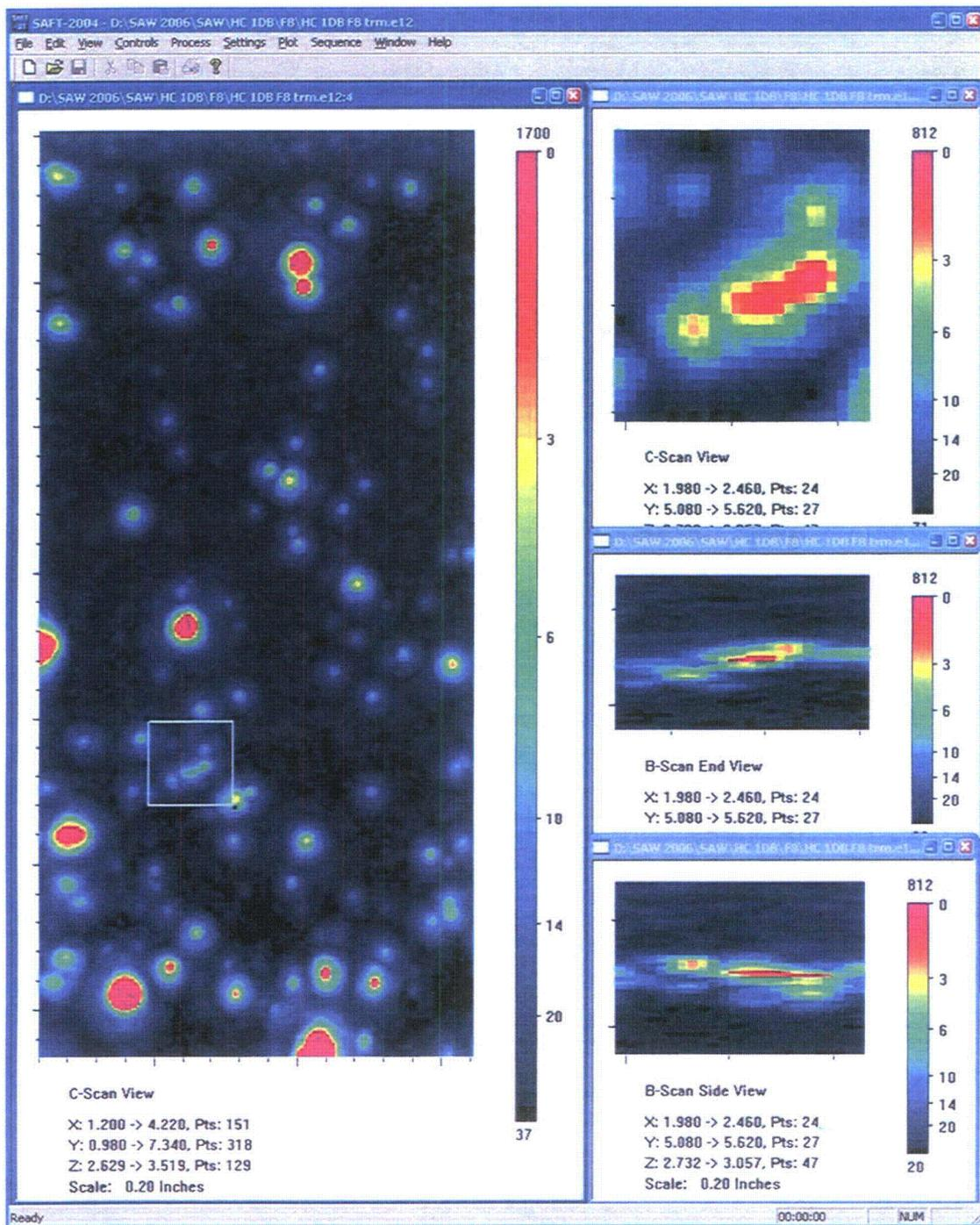
Figure A.12.a 10 MHz F8 Immersion Testing Images of Small Fabrication Flaw: *HC6A*. This figure shows immersion testing data of a 7-mm flaw indication from the weld-normal testing of large weld segments. The flaw indication is identified in the box drawn in the SAFT-UT image on the left in the figure. A close up of the flaw in the C-scan view (top right) shows 4 unresolved flaws.
