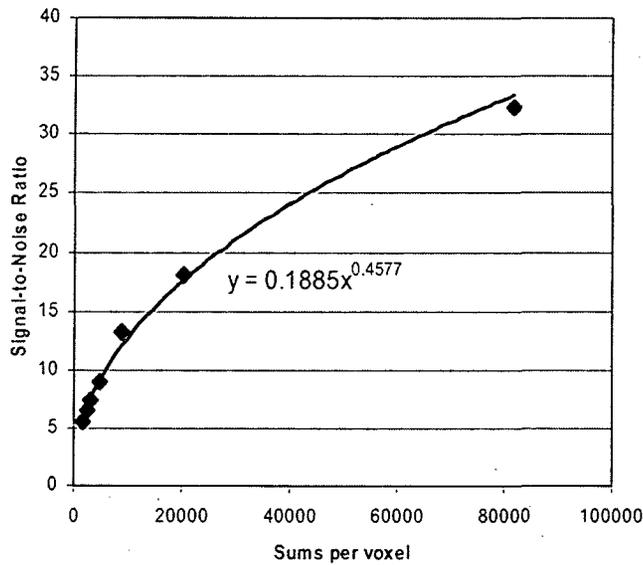
**Figure 3.2 Signal-to-Noise and Sizing Performance for Lens Sampling**
