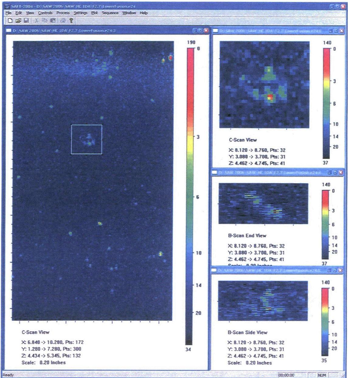
Figure A.11.c F2.7 Immersion Testing Images of Small Fabrication Flaw: *HC5B*. This figure shows the same material and complex flaw as the previous figures. Here the complex flaw is resolved to two flaws with through-wall sizes of 2.5 mm and 2.5 mm.
