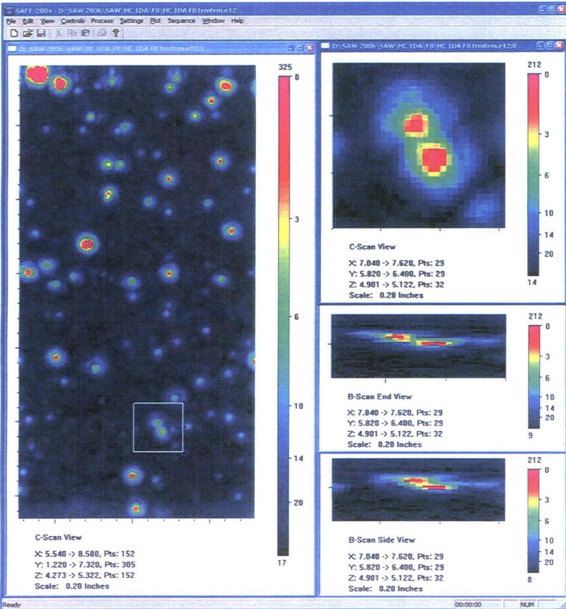
Figure A.10.a 10 MHz F8 Immersion Testing Images of Small Fabrication Flaw: *HC5A*. This figure shows immersion testing data of a 7-mm flaw indication from the weld-normal testing of large weld segments. The flaw indication is identified in the box drawn in the SAFT-UT image on the left in the figure. A close up of the flaw in the C-scan view (top right) shows 2 unresolved flaws.
