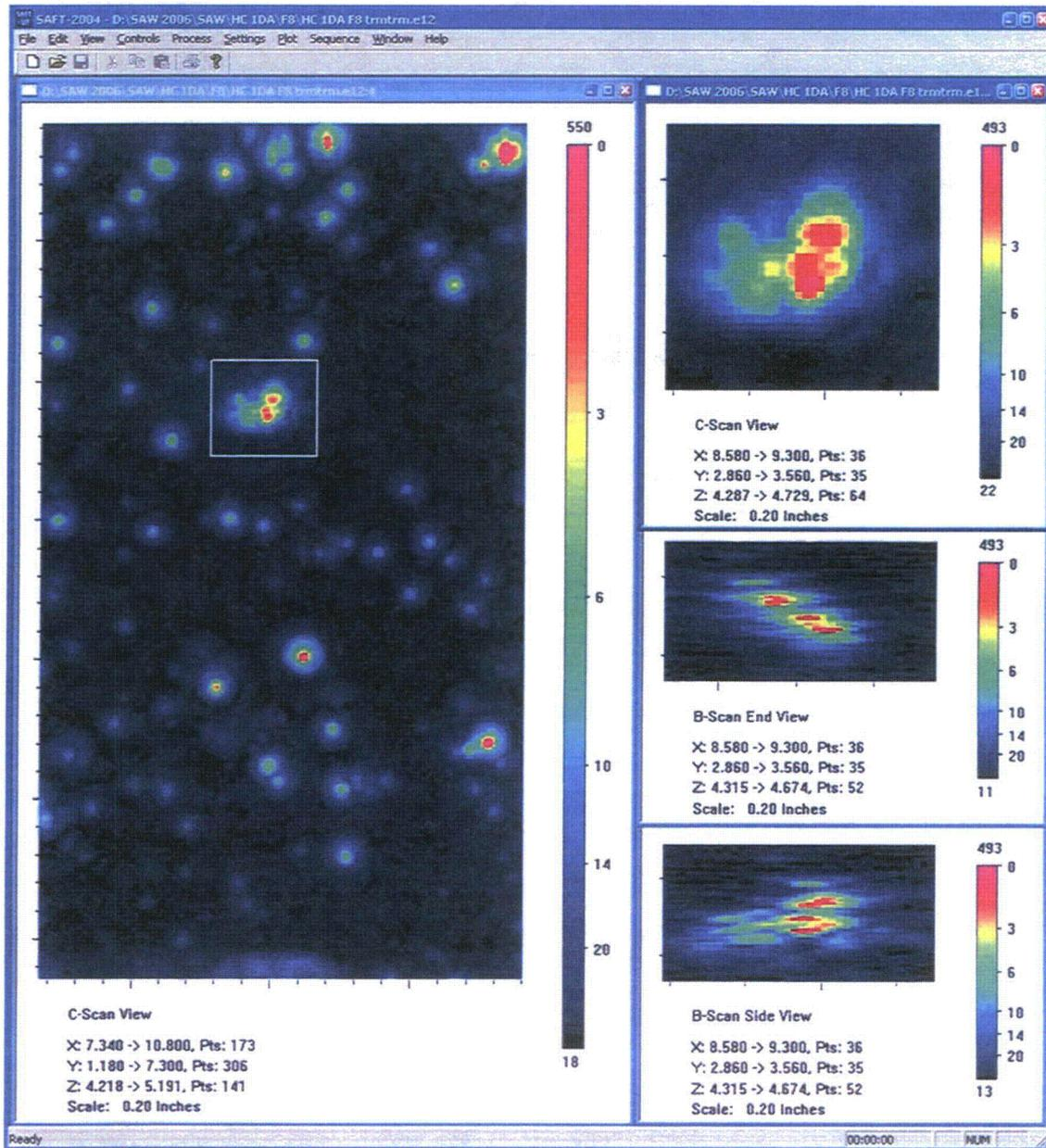
Figure A.11.a 10 MHz F8 Immersion Testing Images of Small Fabrication Flaw: *HC5B*. This figure shows immersion testing data of a complex flaw indication from the weld-normal testing of large weld segments. The flaw indication is identified in the box drawn in the SAFT-UT image on the left in the figure.
