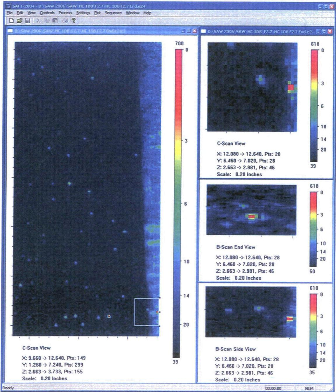
Figure A.9.c F2.7 Immersion Testing Images of Small Fabrication Flaw: *HC4A*. This figure shows the same material and flaw as the previous figures. Here the flaw is resolved to a through-wall size of 2.0 mm.
