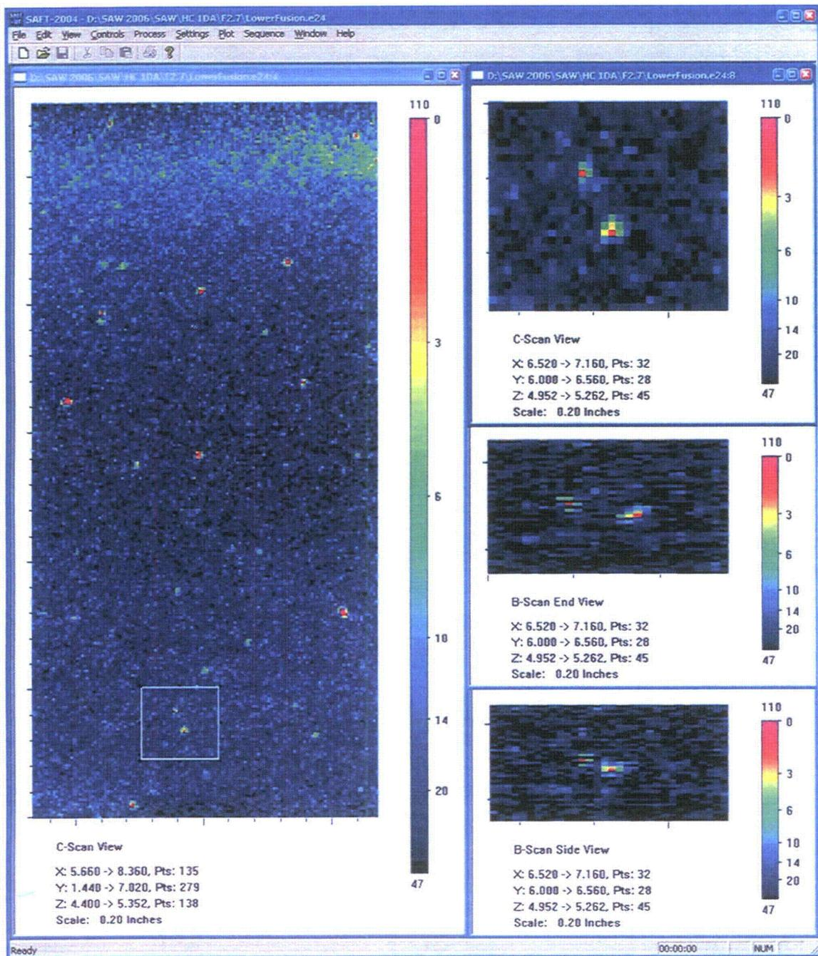
Figure A.10.c F2.7 Immersion Testing Images of Small Fabrication Flaw: *HC5A*. This figure shows the same material and flaw(s) as the previous figures. Here the two flaws are resolved to through-wall sizes of 1.0 mm and 1.5 mm.
