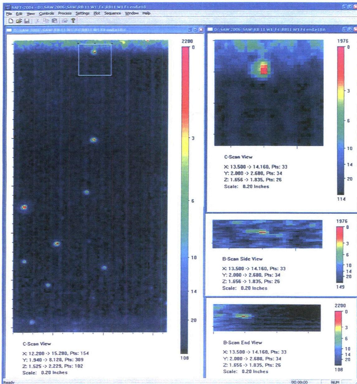
Figure A.4.b F4 Immersion Testing Images of Small Fabrication Flaw: *RB4A*. This figure shows the same material and flaw(s) as the previous figure but with twice the resolving power. The ultrasonic immersion probe was a 10 MHz F4 and as such has a lateral resolution of 1.2 wavelength or 0.7 mm. Here the flaw is resolved both laterally and in depth. The through-wall size is 2.5 mm.
