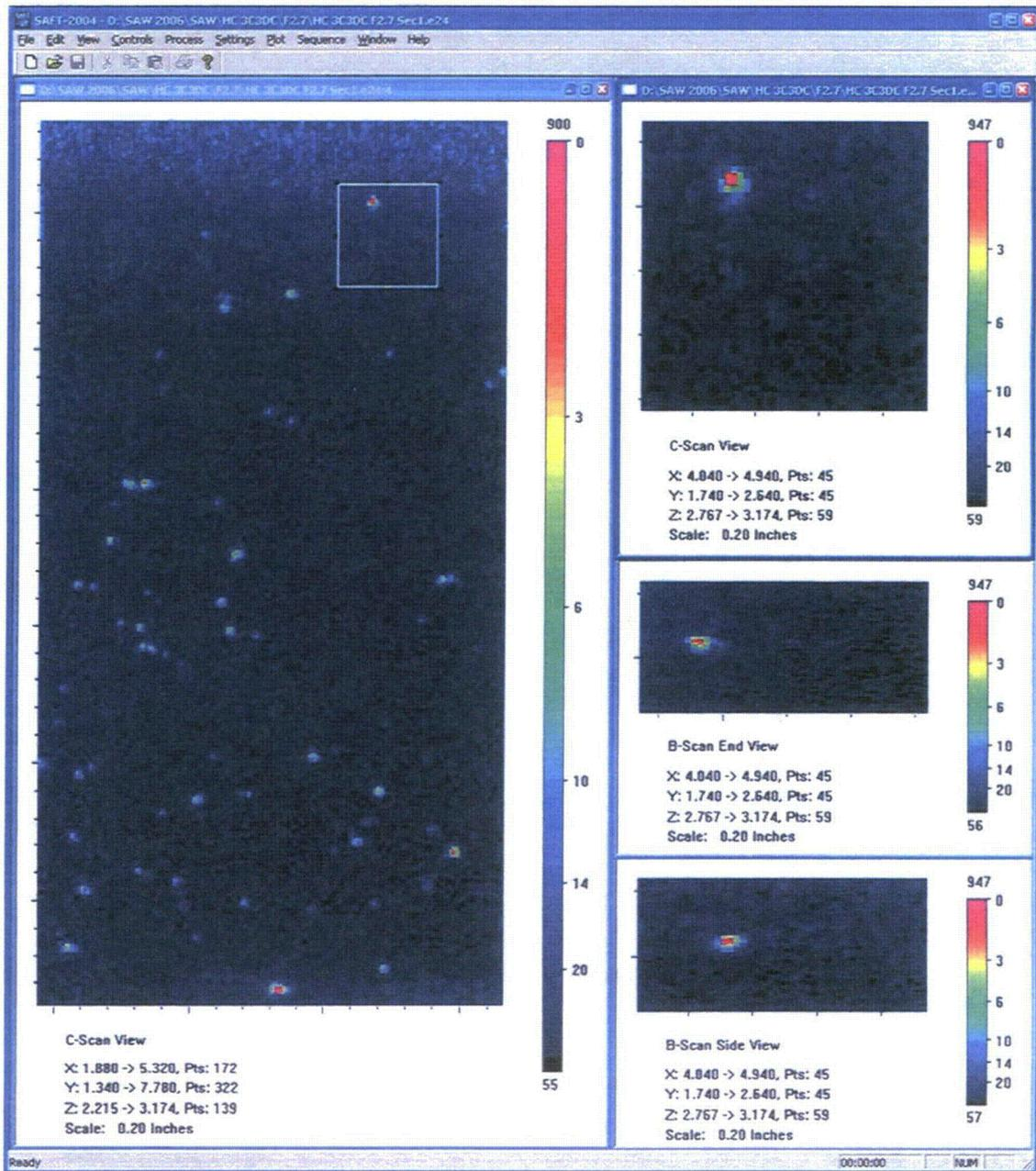
Figure A.6.c F2.7 Immersion Testing Images of Small Fabrication Flaw: *HClA*. This figure shows the same material and flaw as the previous figures. Here the flaw is resolved to a through-wall size of 1.5 mm.
