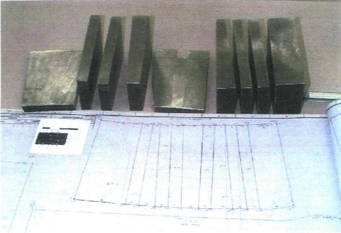
**Figure 2.9 Photo of Weld Cross Section Plates from the PVRUF Vessel**
