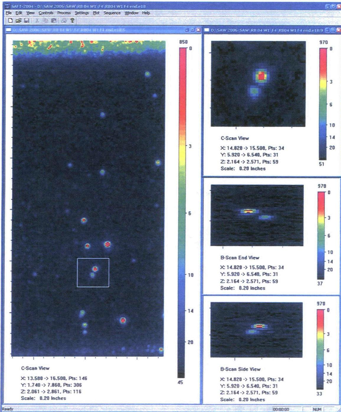
Figure A.1.b F4 Immersion Testing Images of Small Fabrication Flaw: *RBIA*. This figure shows the same material and flaw(s) as the previous figure but with twice the resolving power. The ultrasonic immersion probe was a 10 MHz F4 and as such has a lateral resolution of 1.2 wavelength or 0.7 mm. Here the two flaws are resolved both laterally and in depth. The through-wall sizes are 2.0 mm and 1.0 mm.
