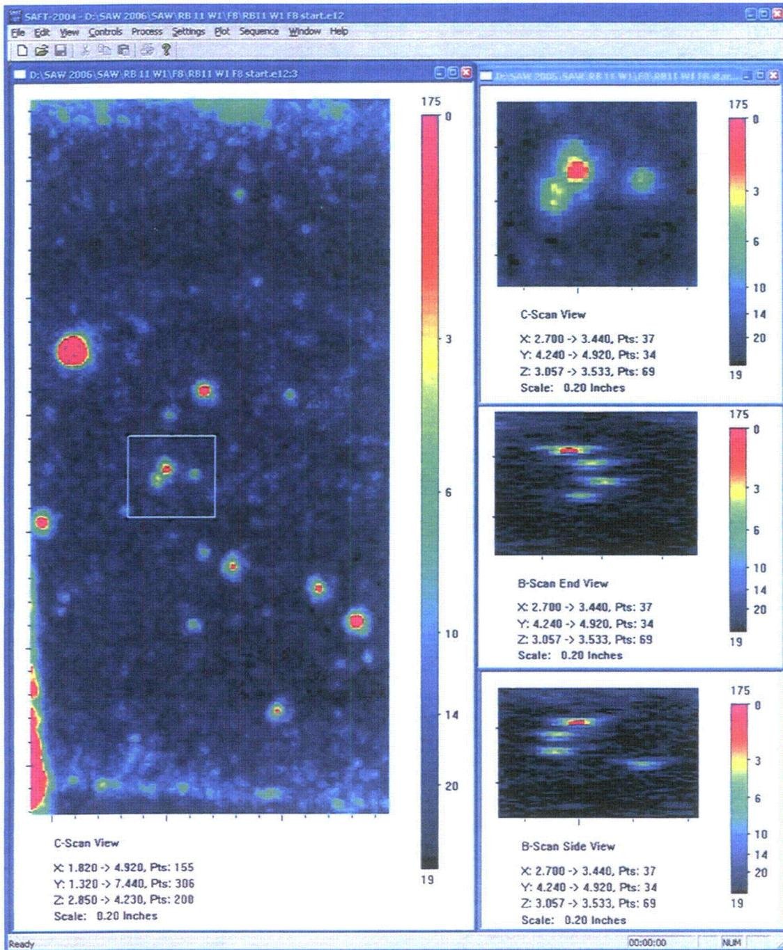
Figure A.5.a 10 MHz F8 Immersion Testing Images of Small Fabrication Flaw: *RB5A*. This figure shows immersion testing data of a 5.5-mm flaw indication from the weld-normal testing of large weld segments. The flaw indication is identified in the box drawn in the SAFT-UT image on the left in the figure. A close up of the flaw in the C-scan view (top right) shows 2 unresolved flaws.
