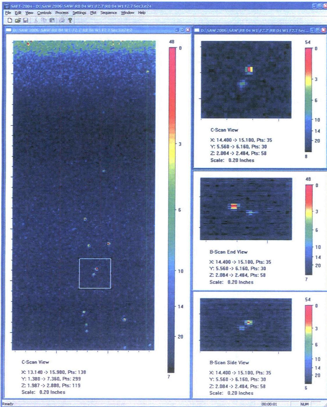
Figure A.1.c F2.7 Immersion Testing Images of Small Fabrication Flaw: *RBIA*. This figure shows the same material and flaw(s) as the previous figures. Here the two flaws are resolved to through-wall sizes of 1.0 mm and 0.5 mm.
