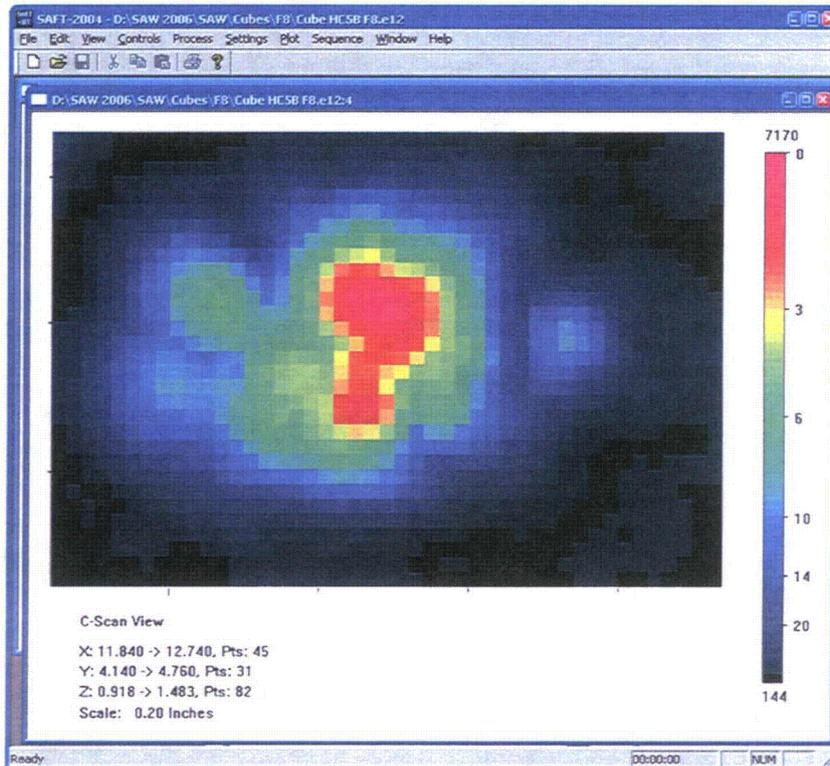
Figure 2.12 F8 Immersion UT of Fabrication Flaw in Cube: *HC5B*
