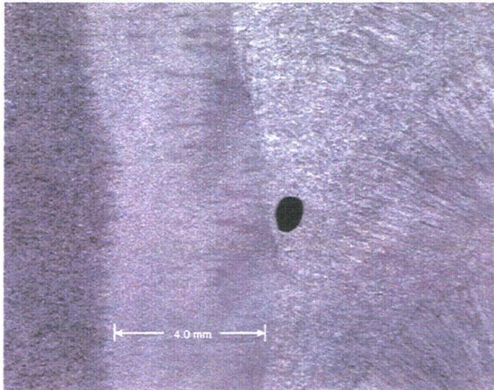
Figure B.1 Metallograph of Flaw RB2A at 10x
