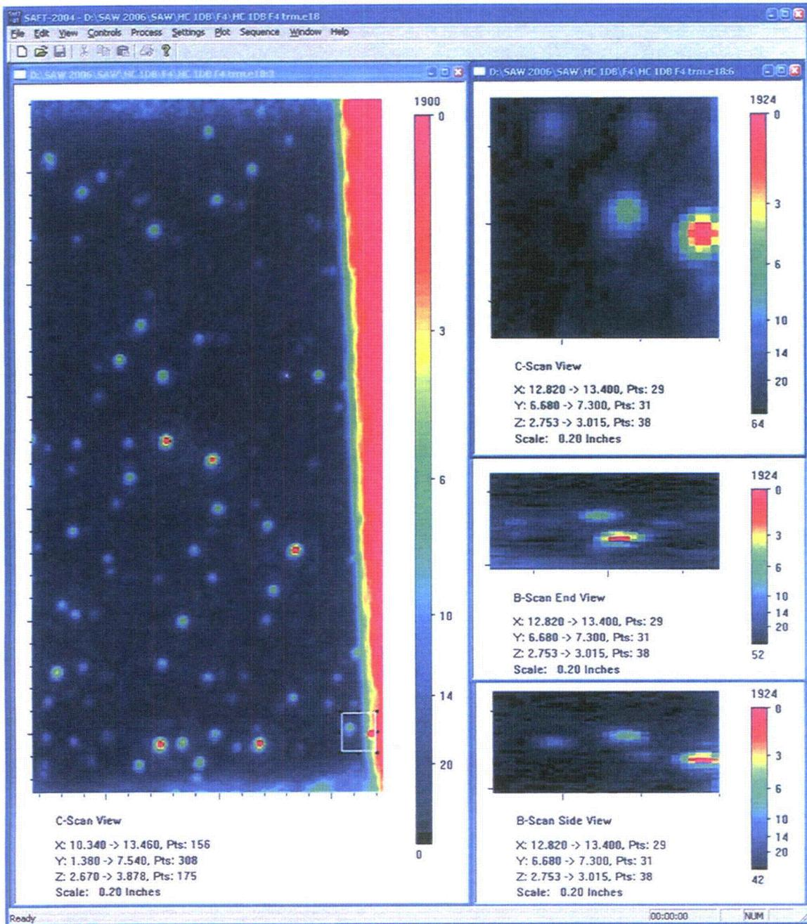
Figure A.9.b F4 Immersion Testing Images of Small Fabrication Flaw: *HC4A*. This figure shows the same material and flaw(s) as the previous figure but with twice the resolving power. The ultrasonic immersion probe was a 10 MHz F4 and as such has a lateral resolution of 1.2 wavelength or 0.7 mm. Here the flaw is resolved both laterally and in depth with a through-wall size of 2.5 mm.
