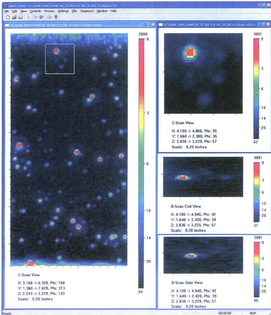
Figure A.6.b F4 Immersion Testing Images of Small Fabrication Flaw: *HClA*. This figure shows the same material and flaw(s) as the previous figure but with twice the resolving power. The ultrasonic immersion probe was a 10 MHz F4 and as such has a lateral resolution of 1.2 wavelength or 0.7 mm. Here the flaw is resolved both laterally and in depth with a through-wall size of 2.5 mm.
