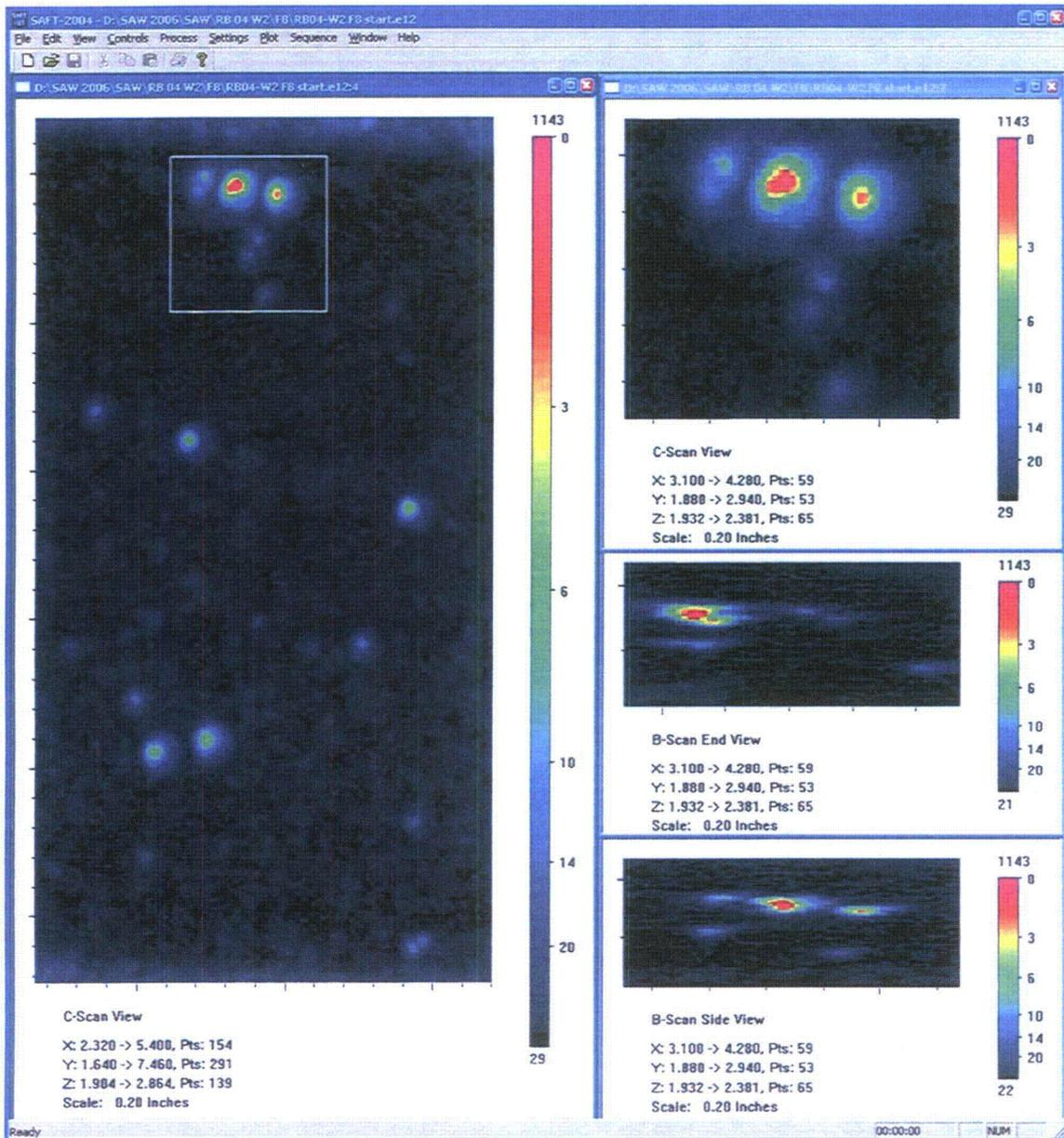
Figure A.3.a 10 MHz F8 Immersion Testing Images of Small Fabrication Flaw: *RB3A*. This figure shows immersion testing data of a 6-mm flaw indication from the weld-normal testing of large weld segments. The flaw indication is identified in the box drawn in the SAFT-UT image on the left in the figure.
