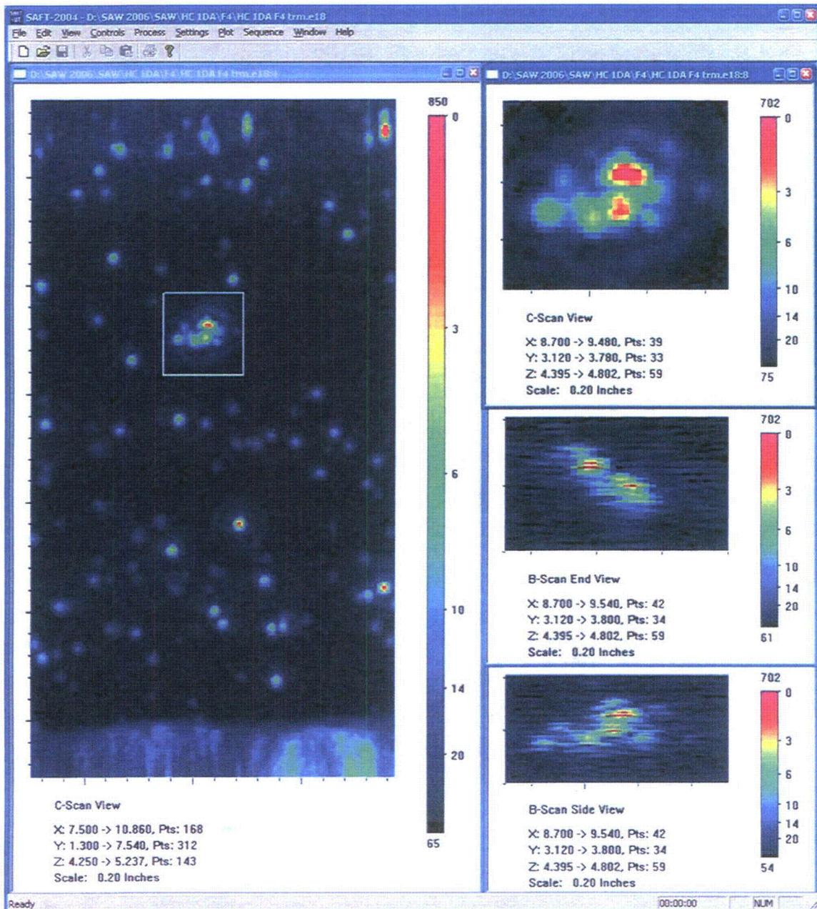
Figure A.11.b F4 Immersion Testing Images of Small Fabrication Flaw: *HC5B*. This figure shows the same material and complex flaw as the previous figure but with twice the resolving power. The ultrasonic immersion probe was a 10 MHz F4 and as such has a lateral resolution of 1.2 wavelength or 0.7 mm.
