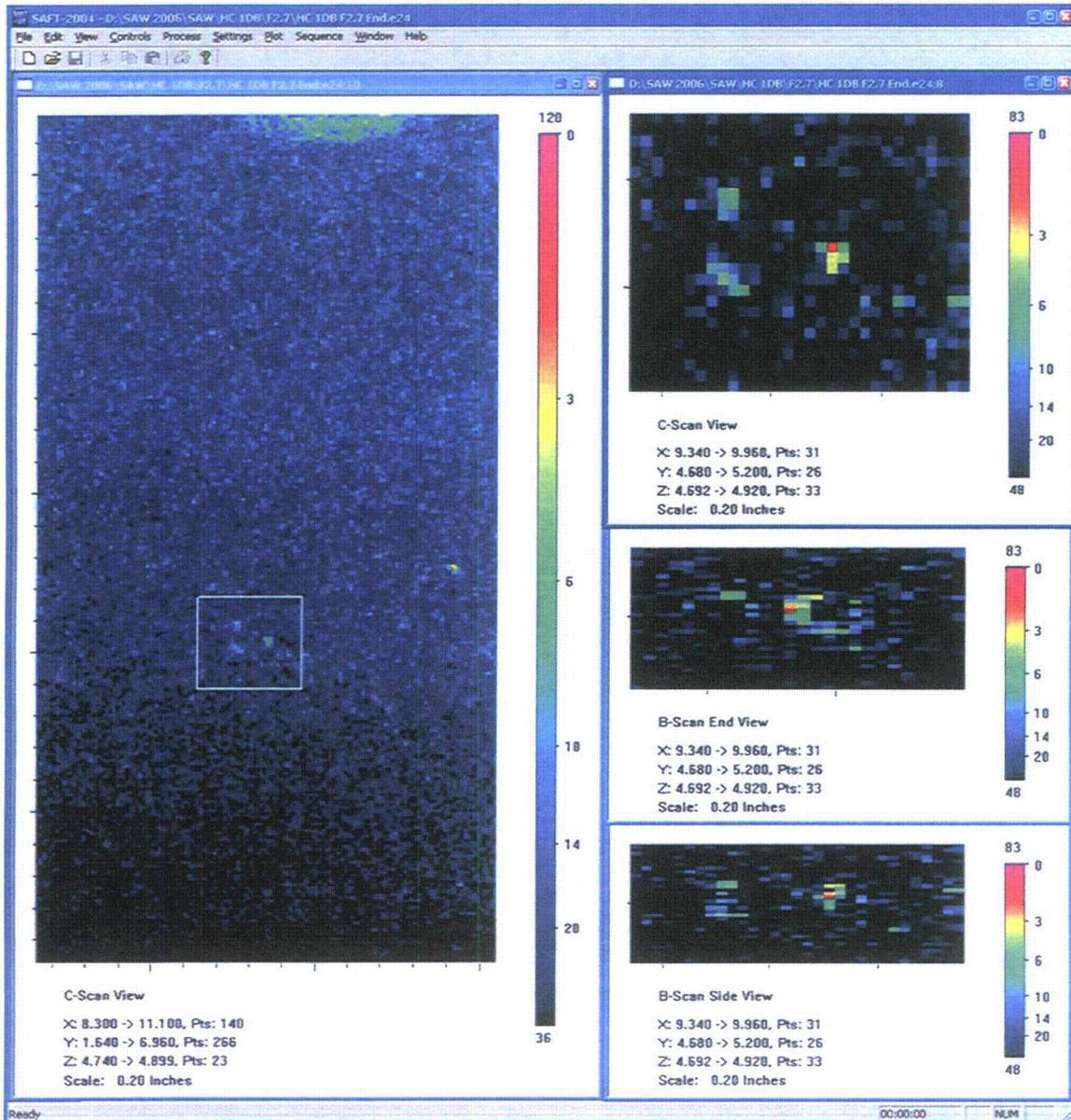
Figure A.7.c F2.7 Immersion Testing Images of Small Fabrication Flaw: *HC3A*. This figure shows the same material and flaw(s) as the previous figures. Here the flaws are resolved to through-wall sizes of 2.0 mm, 1.5 mm, and 1.5 mm.
