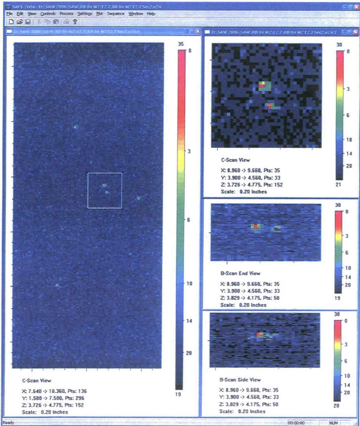
Figure A.2.c F2.7 Immersion Testing Images of Small Fabrication Flaw: *RB2A*. This figure shows the same material and flaw(s) as the previous figures. Here the two flaws are resolved to through-wall sizes of 1.5 mm and 1.0 mm.
