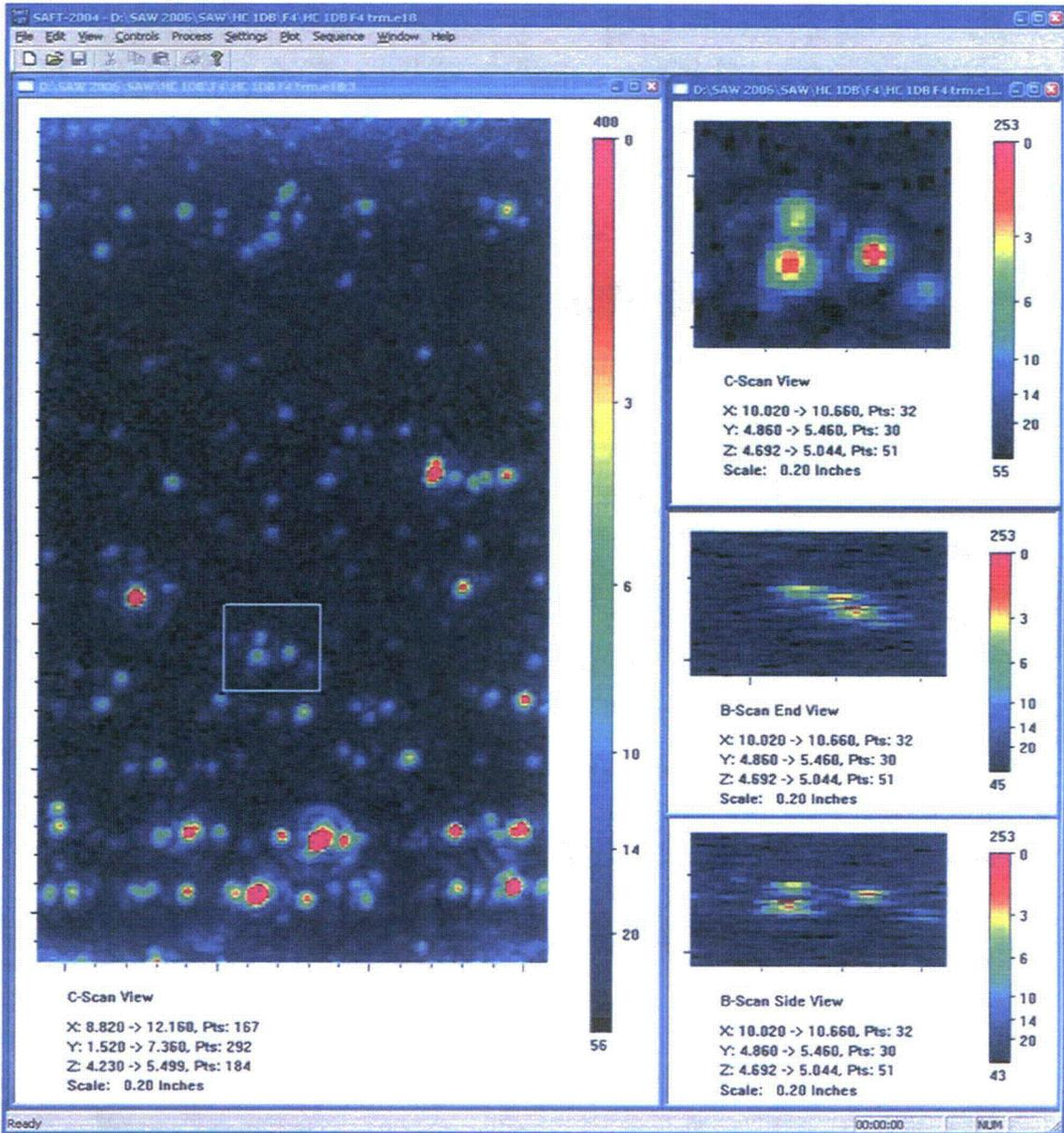
Figure A.7.b F4 Immersion Testing Images of Small Fabrication Flaw: *HC3A*. This figure shows the same material and flaw(s) as the previous figure but with twice the resolving power. The ultrasonic immersion probe was a 10 MHz F4 and as such has a lateral resolution of 1.2 wavelength or 0.7 mm. Here the 2 flaws are resolved to 3 flaws both laterally and in depth. Through-wall sizes are 3.0 mm, 2.5 mm and 2.5 mm.
