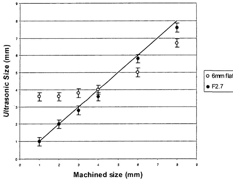
**Figure 3.3 Sizing Performance for Immersion F2.7 Transducer versus a 6-mm Flat Transducer in Contact with Test Specimen Containing Flat-Bottom Holes**
