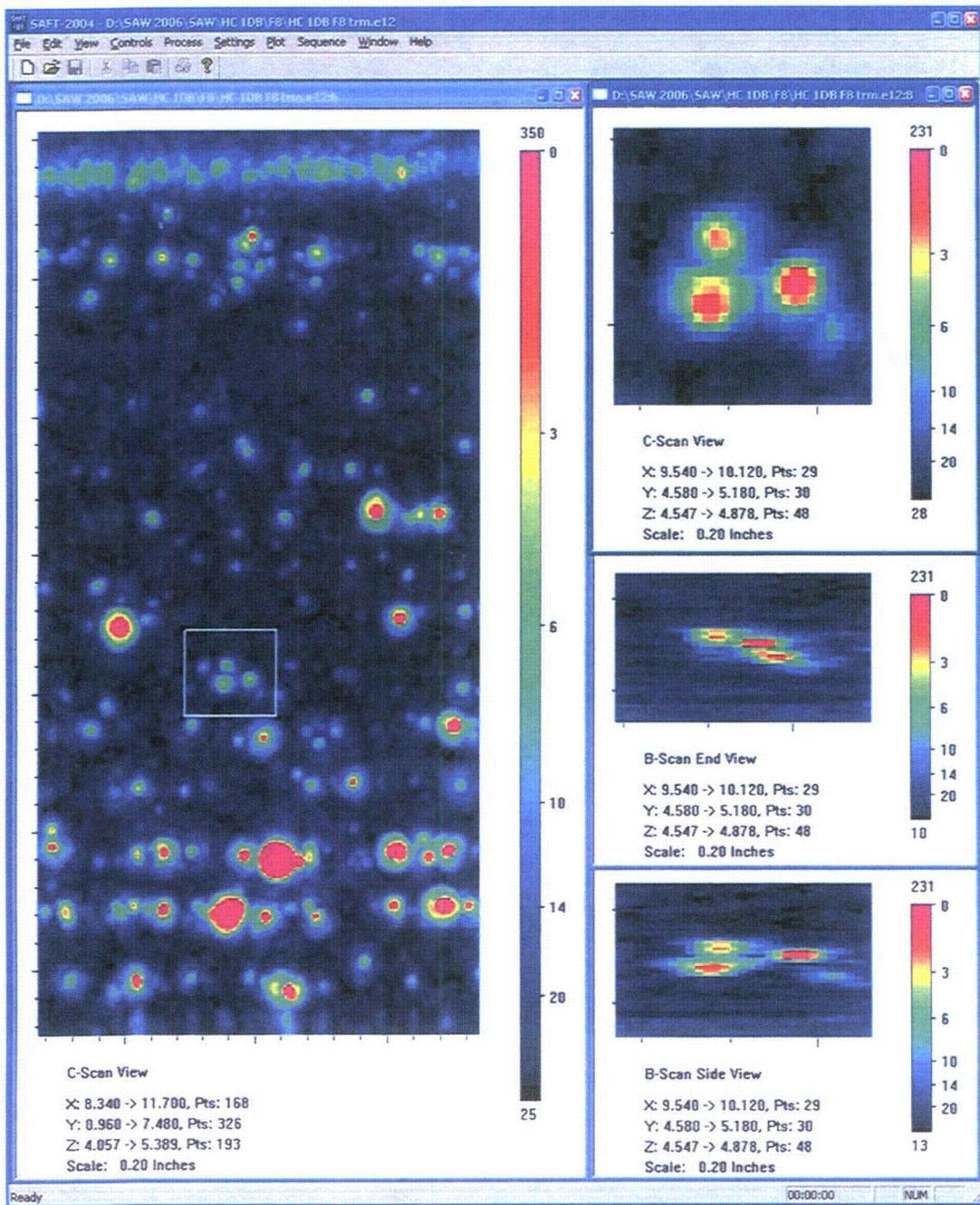
Figure A.7.a 10 MHz F8 Immersion Testing Images of Small Fabrication Flaw: *HC3A*. This figure shows immersion testing data of a 7-mm flaw indication from the weld-normal testing of large weld segments. The flaw indication is identified in the box drawn in the SAFT-UT image on the left in the figure. A close up of the flaw in the C-scan view (top right) shows 3 unresolved flaws.
