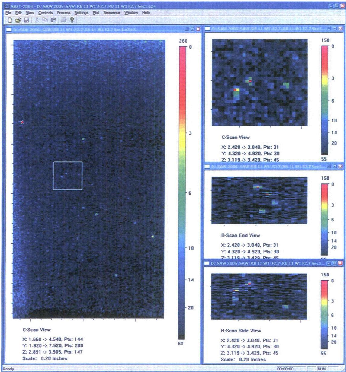
Figure A.5.c F2.7 Immersion Testing Images of Small Fabrication Flaw: *RB5A*. This figure shows the same material and flaw(s) as the previous figures. Here the two flaws are resolved to through-wall sizes of 1.0 mm and 1.5 mm.
