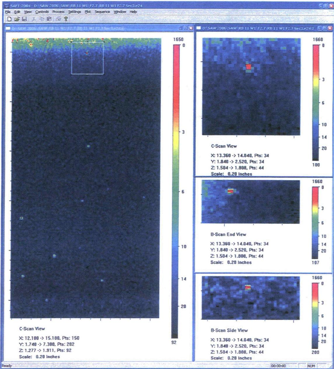
Figure A.4.c F2.7 Immersion Testing Images of Small Fabrication Flaw: *RB4A*. This figure shows the same material and flaw as the previous figures. Here the flaw is resolved to a through-wall size of 1.0 mm.
