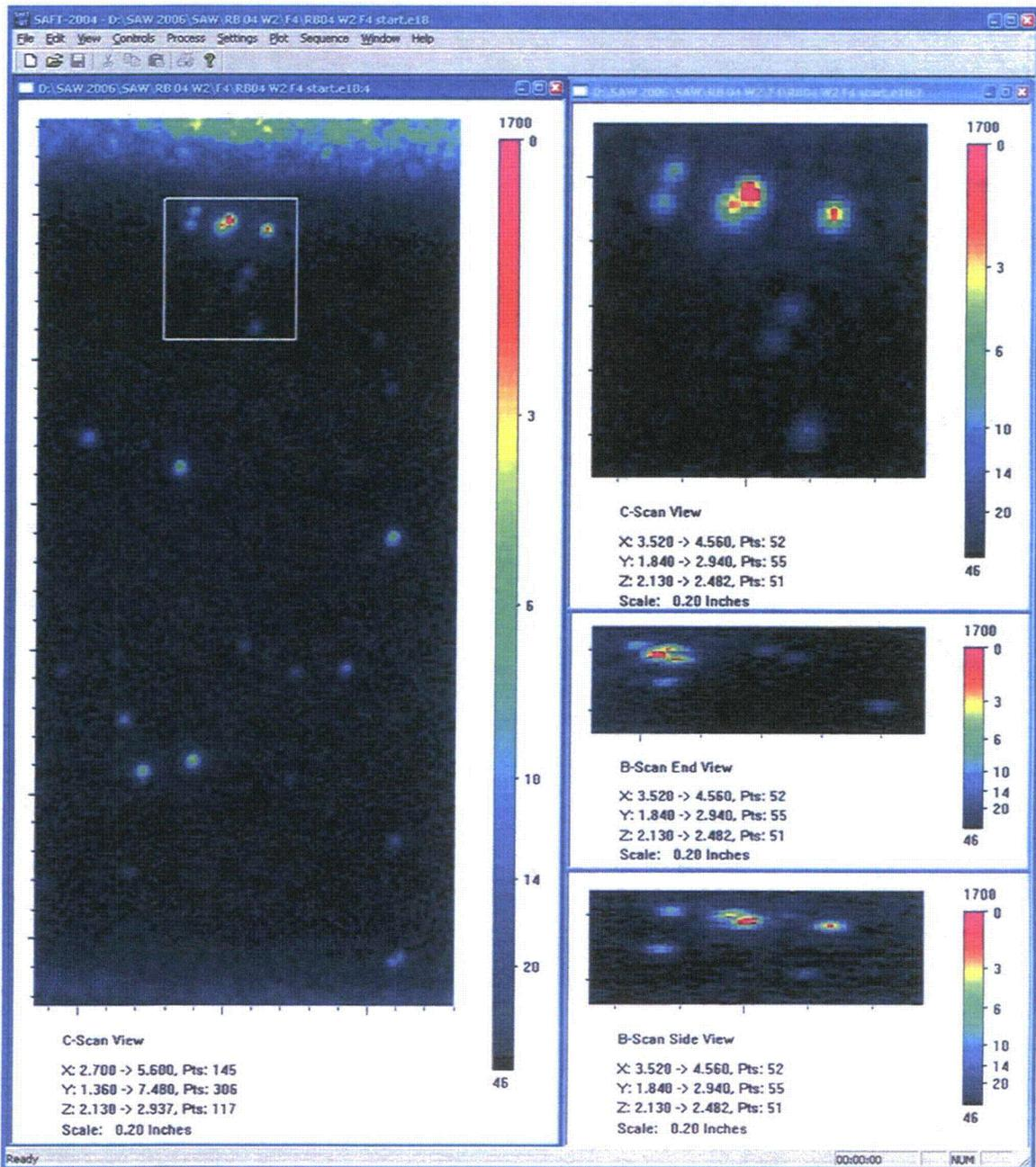
Figure A.3.b F4 Immersion Testing Images of Small Fabrication Flaw: *RB3A*. This figure shows the same material and flaw(s) as the previous figure but with twice the resolving power. The ultrasonic immersion probe was a 10 MHz F4 and as such has a lateral resolution of 1.2 wavelength or 0.7 mm. Here the flaw is resolved both laterally and in depth. The through-wall size is 2.5 mm.
