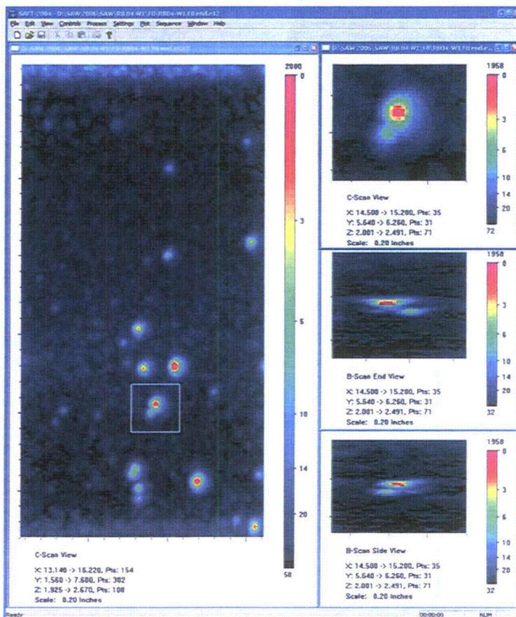
Figure A.1.a 10 MHz F8 Immersion Testing Images of Small Fabrication Flaw: *RB1A*. This figure shows immersion testing data of a 5.5-mm flaw indication from the weld-normal testing of large weld segments. The flaw indication is identified in the box drawn in the SAFT-UT image on the left in the figure. A close up of the flaw in the C-scan view (top right) shows 2 unresolved flaws.
