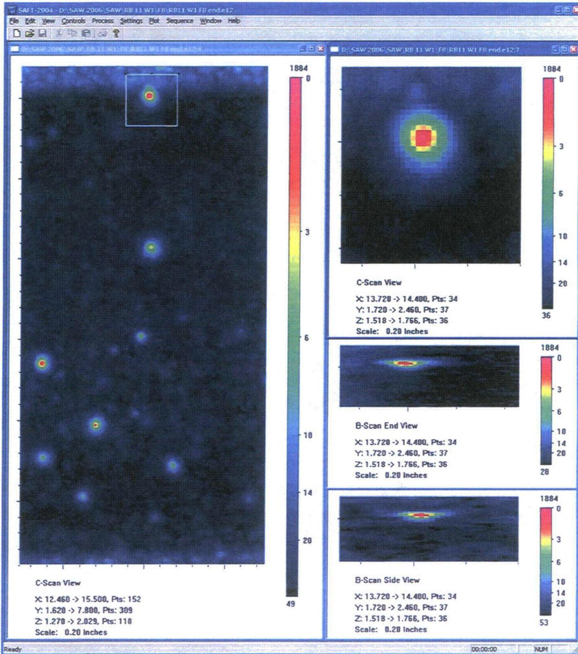
Figure A.4.a 10 MHz F8 Immersion Testing Images of Small Fabrication Flaw: *RB4A*. This figure shows immersion testing data of a 6-mm flaw indication from the weld-normal testing of large weld segments. The flaw indication is identified in the box drawn in the SAFT-UT image on the left in the figure.
