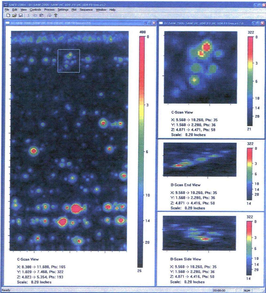
Figure A.8.a 10 MHz F8 Immersion Testing Images of Small Fabrication Flaw: *HC3B (HC 1DB-3 / 1DIE 14.0 mm)*. This figure shows immersion testing data of a 14-mm flaw indication from the weld-normal testing of large weld segments. The flaw indication is identified in the box drawn in the SAFT-UT image on the left in the figure.
