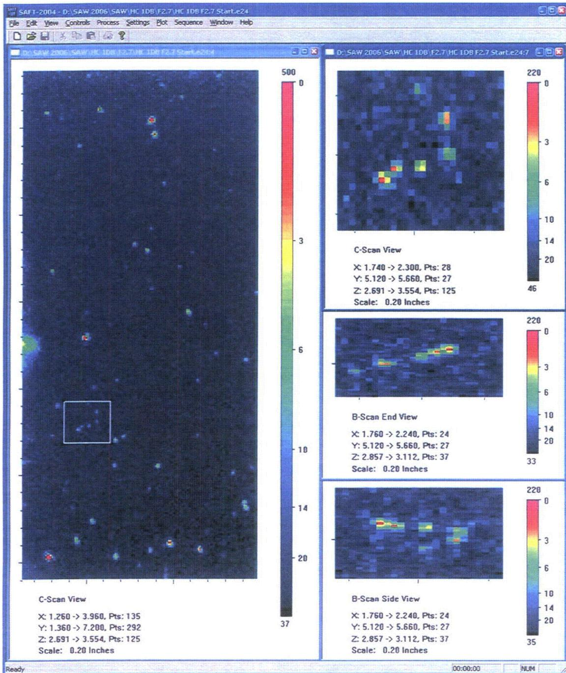
Figure A.12.c F2.7 Immersion Testing Images of Small Fabrication Flaw: *HC6A*. This figure shows the same material and flaw(s) as the previous figures. Here the four flaws are resolved to through-wall sizes of 1.5 mm, 2.0 mm, 2.0 mm and 1.5 mm.
