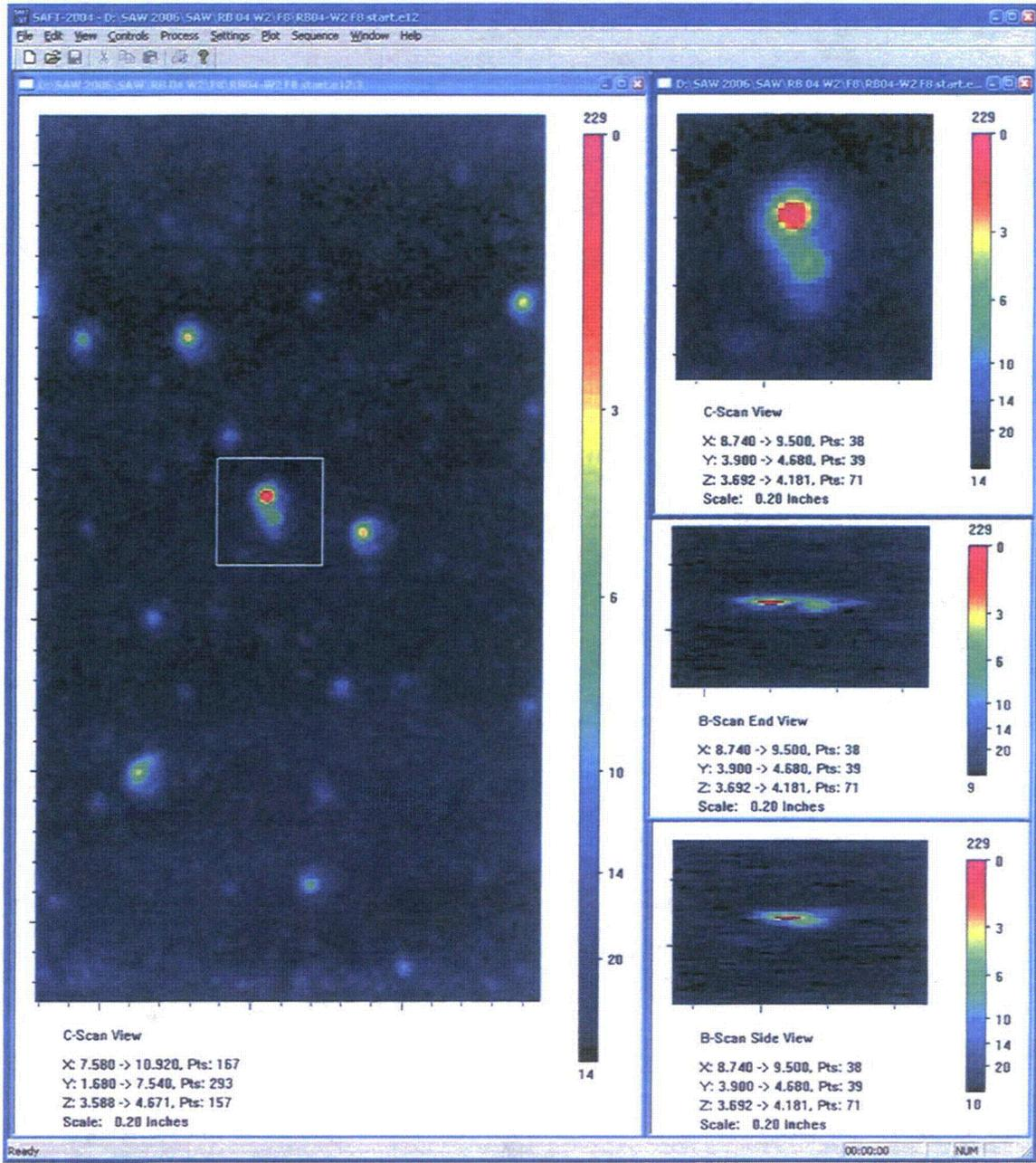
Figure A.2.a 10 MHz F8 Immersion Testing Images of Small Fabrication Flaw: *RB2A*. This figure shows immersion testing data of a 5.5-mm flaw indication from the weld-normal testing of large weld segments. The flaw indication is identified in the box drawn in the SAFT-UT image on the left in the figure. A close up of the flaw in the C-scan view (top right) shows 2 unresolved flaws.
