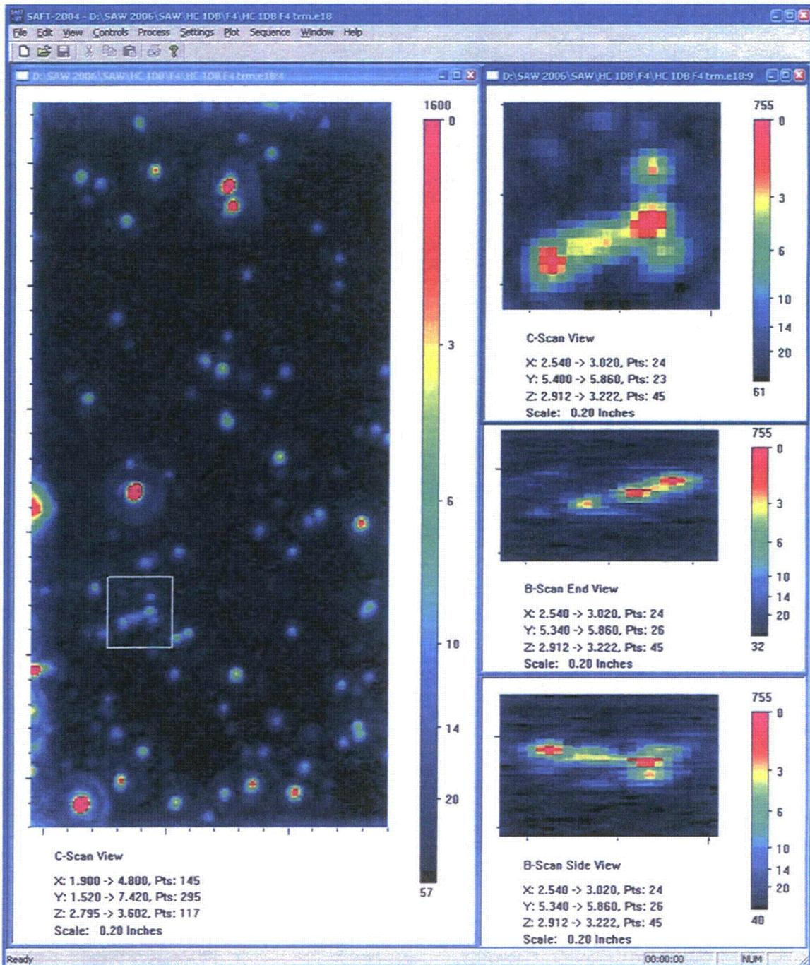
Figure A.12.b F4 Immersion Testing Images of Small Fabrication Flaw: *HC6A*. This figure shows the same material and flaw(s) as the previous figure but with twice the resolving power. The ultrasonic immersion probe was a 10 MHz F4 and as such has a lateral resolution of 1.2 wavelength or 0.7 mm. Here the four flaws are resolved both laterally and in depth to 2 flaws. The through-wall sizes are 1.5 mm and 4.5 mm.
