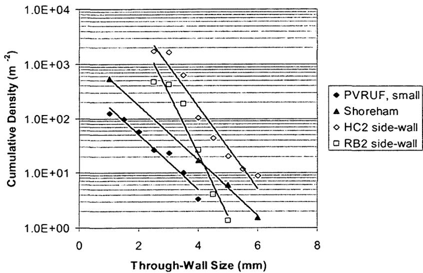
**Figure 5.5 Comparison of Through-Wall Size Distribution of Cumulative Flow Densities for Side-Wall Fusion Zones in SAW**
