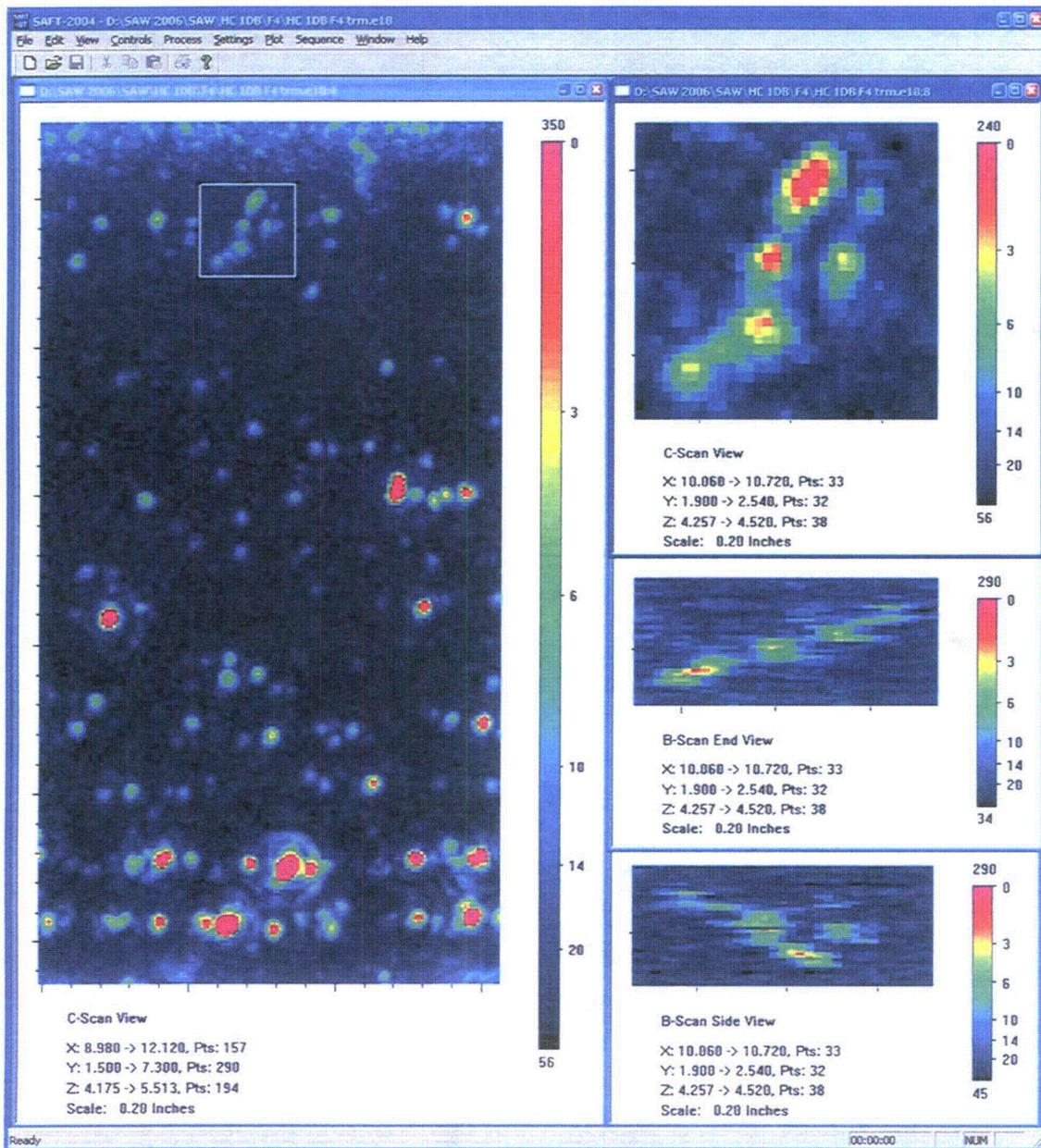
Figure A.8.b F4 Immersion Testing Images of Small Fabrication Flaw: *HC3B (HC 1DB-3 / 1DIE 14.0mm)*. This figure shows the same material and flaw(s) as the previous figure but with twice the resolving power. The ultrasonic immersion probe was a 10 MHz F4 and as such has a lateral resolution of 1.2 wavelength or 0.7 mm.
