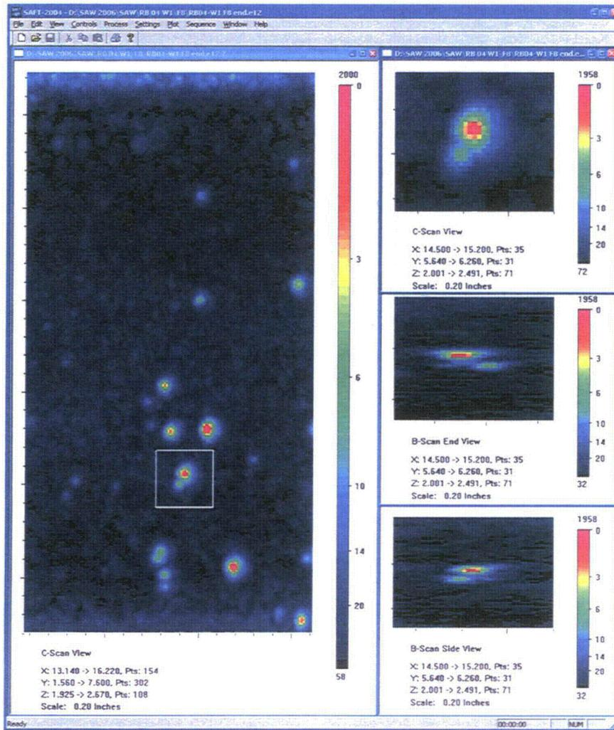
Figure 2.6 F8 Immersion Testing Images of Small Fabrication Flaw: *RB04-5.5*
