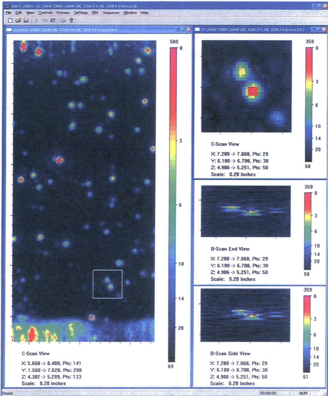
Figure A.10.b F4 Immersion Testing Images of Small Fabrication Flaw: *HC5A*. This figure shows the same material and flaw(s) as the previous figure but with twice the resolving power. The ultrasonic immersion probe was a 10 MHz F4 and as such has a lateral resolution of 1.2 wavelength or 0.7 mm. Here the two flaws are resolved both laterally and in depth. The through-wall sizes are 2.0 mm and 2.5 mm.
