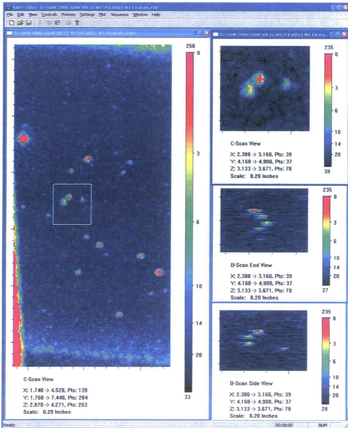
Figure A.5.b F4 Immersion Testing Images of Small Fabrication Flaw: *RB5A*. This figure shows the same material and flaw(s) as the previous figure but with twice the resolving power. The ultrasonic immersion probe was a 10 MHz F4 and as such has a lateral resolution of 1.2 wavelength or 0.7 mm. Here the two flaws are resolved both laterally and in depth. The through-wall sizes are 2.5 mm and 3.0 mm.
