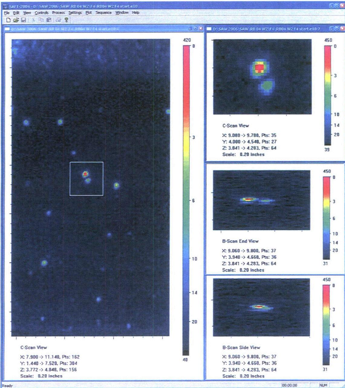
Figure A.2.b F4 Immersion Testing Images of Small Fabrication Flaw: *RB2A*. This figure shows the same material and flaw(s) as the previous figure but with twice the resolving power. The ultrasonic immersion probe was a 10 MHz F4 and as such has a lateral resolution of 1.2 wavelength or 0.7 mm. Here the two flaws are resolved both laterally and in depth. The through-wall sizes are 2.5 mm and 1.5 mm.
