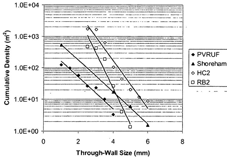
**Figure ES.1 Comparison of Through-Wall Size Distribution of Cumulative Flaw Densities for Side-Wall Fusion Zones in SAW. HC2 stands for the Hope Creek Unit 2 vessel; RB2 stands for the River Bend Unit 2 vessel.**
