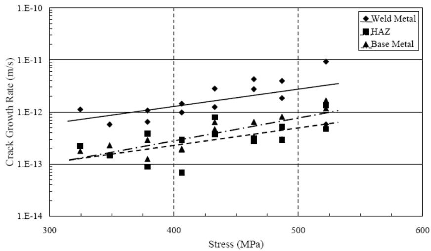
FIGURE 18 - Relationship between Stress and the Crack Growth Rate of PWSCC Microcracks of a Welded Specimen by Alloy 132 in 325 °C
