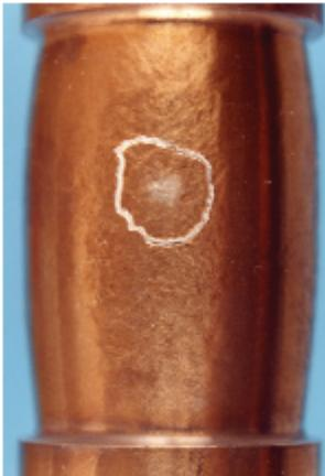
Figure 5. Macroscopic view of a failed capsule
