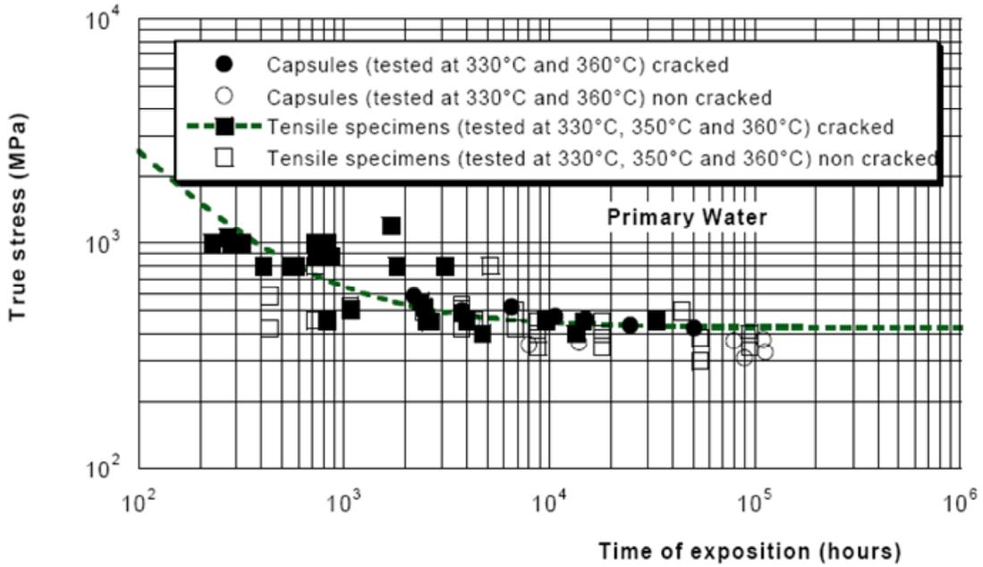
Figure 1. Time to Failure of Alloy 182 in Primary Water as a Function of Stress [4]
