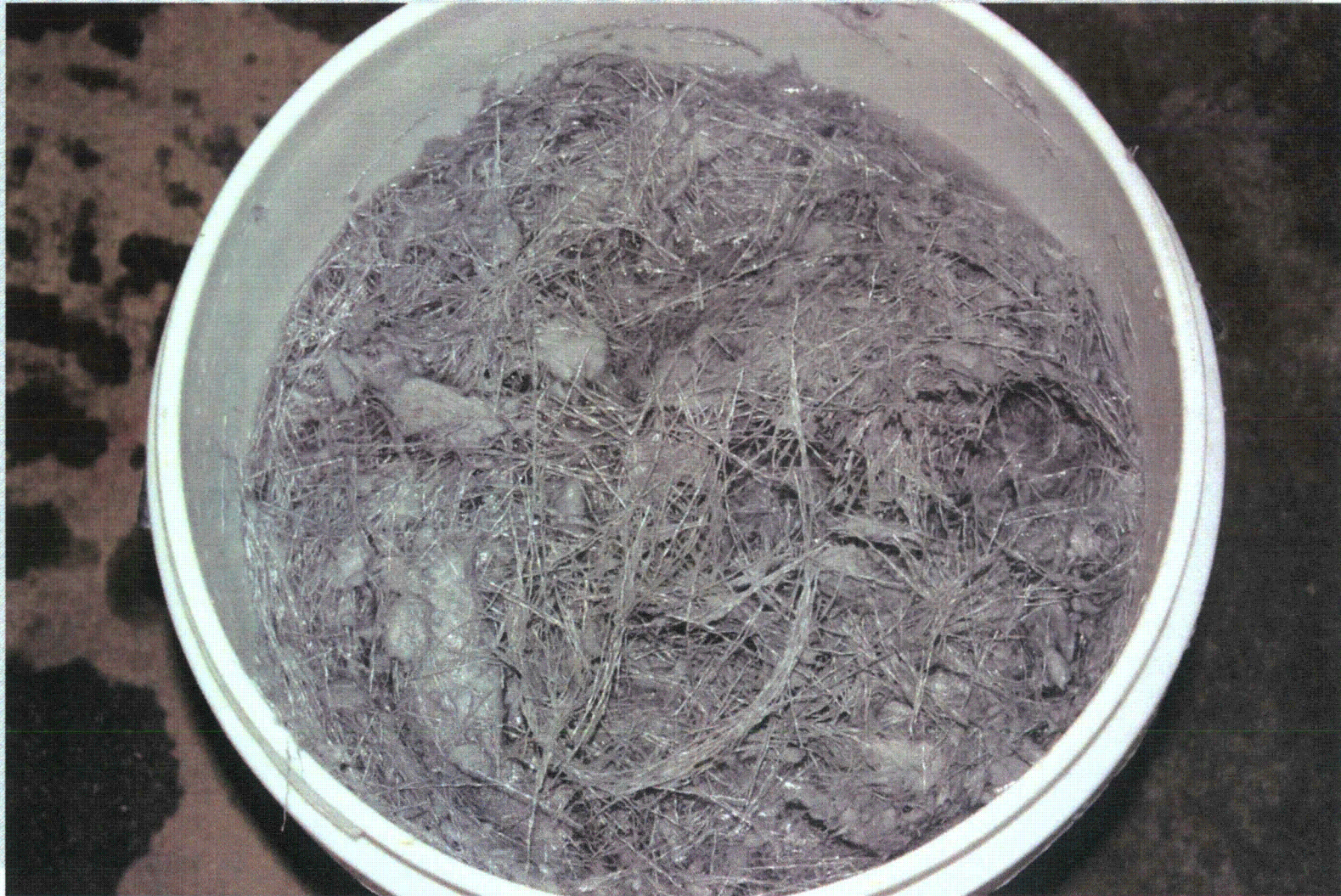
Figure 3.b-13 Blanket debris prep for head loss testing
