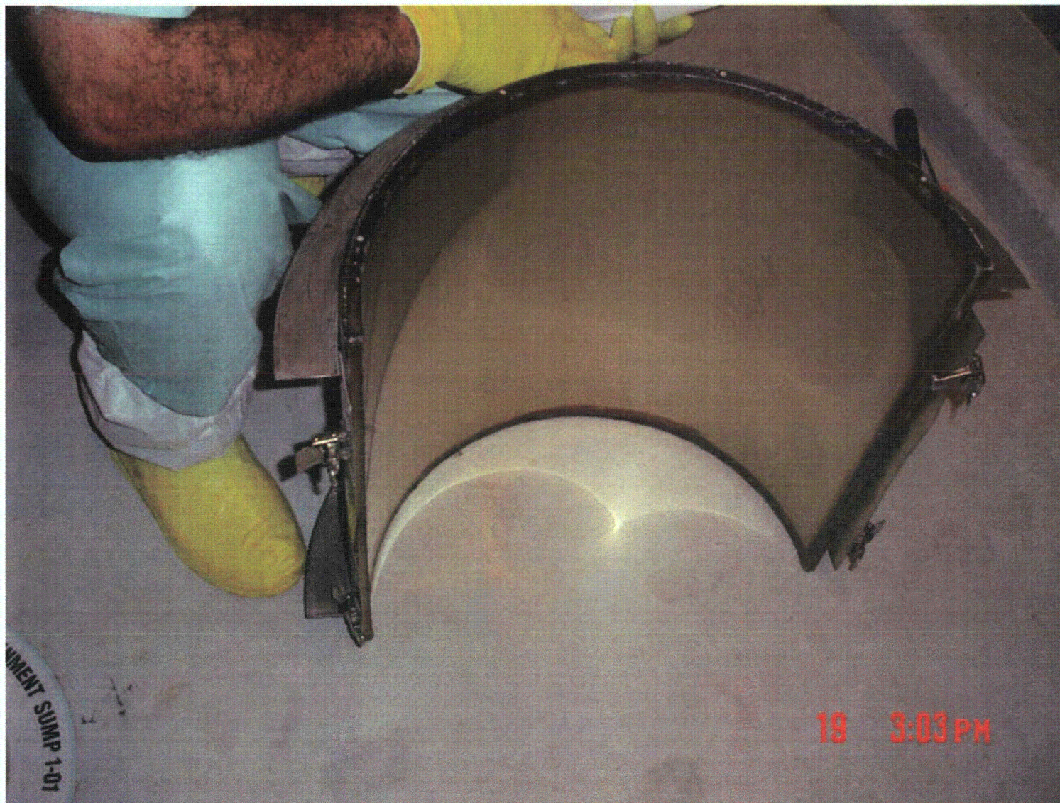
Figure 3.b-15 Min-K Cassette (solid ends, continuous welds)
