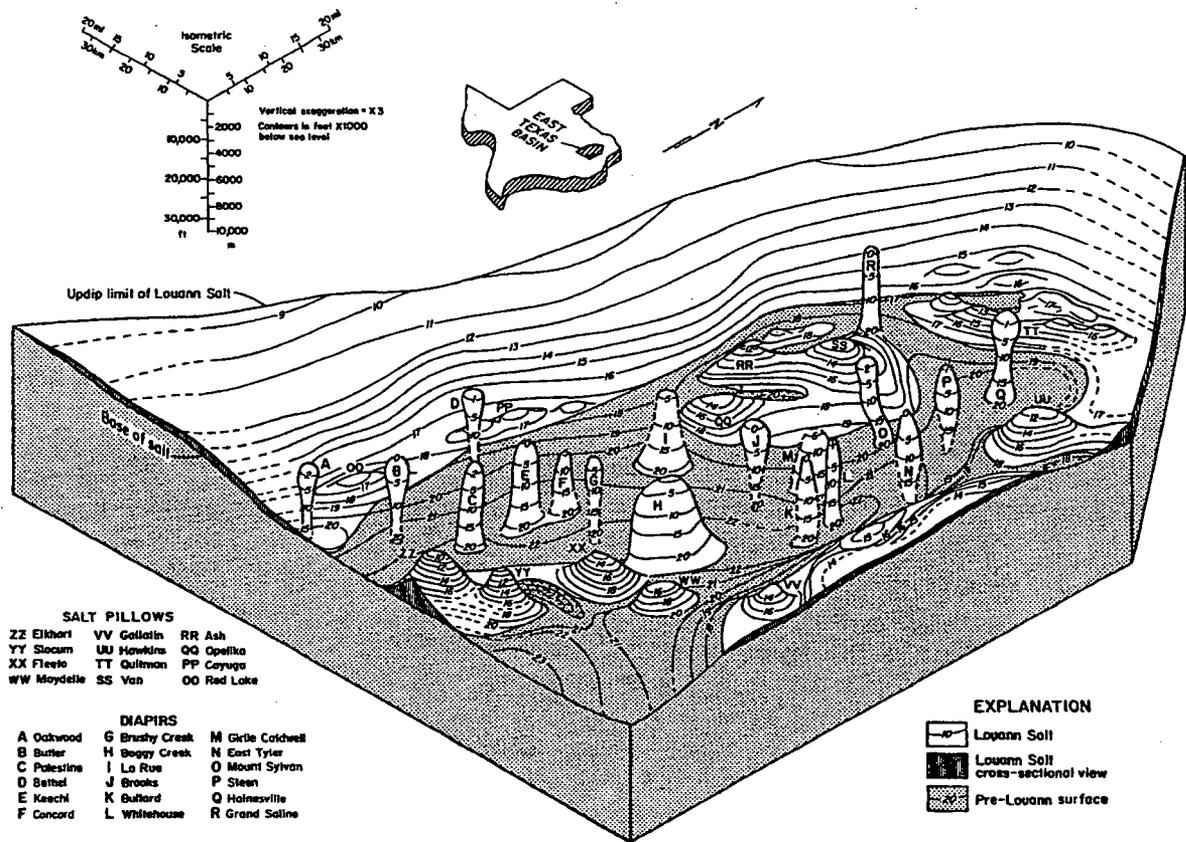
Figure PH.1 Block diagram of salt domes and diapirs in the East Texas Basin showing the three-dimensional configuration of structural contours on top of the Louann Salt or, where the salt is absent, on top of pre-Louann basement. From Seni and Jackson (1984, figure 6A). Permission to use this copyrighted material is granted by the Bureau of Economic Geology, University of Texas.
