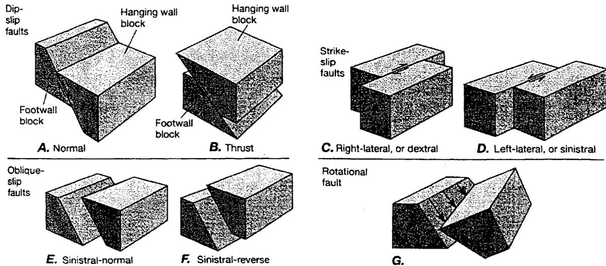
Figure 2.1 Faulted blocks showing the characteristic displacement for the different classes of faults
