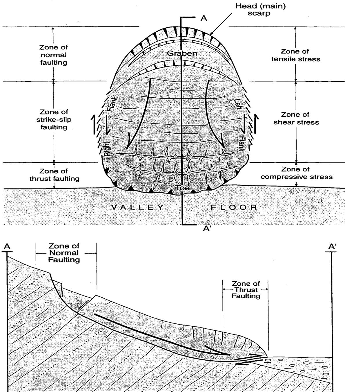
**Figure WC.3** Map and cross section views of a typical landslide showing main landslide features, types of stresses and boundary faulting.
