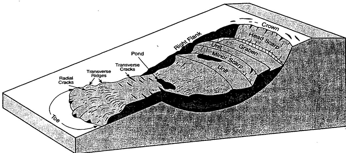
**Figure WC.2** Diagrammatic landslide block diagram showing the main identifying geomorphic features produced by sliding. Geomorphic features such as arcuate head scarps, grabens, linear flanks, bulging toes, closed ponded depressions, hummocky topography and flat bench-like unit surfaces are characteristics of most landslides, and appear in marked contrast to the neighboring intact mountainside. In all three areas, the origin of surface ruptures remains unresolved.
