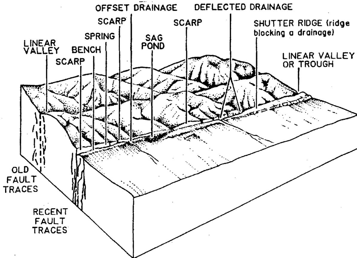
Figure 2.2 Block diagram of geomorphic structures associated with strike-slip faults (from Wesson et al., 1975).
