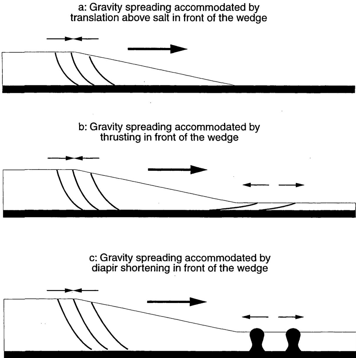
Figure BV.5 Three main types of progradational settings in which gravity spreading of the sediment wedge triggers extension in the shelf and the upper slope.
