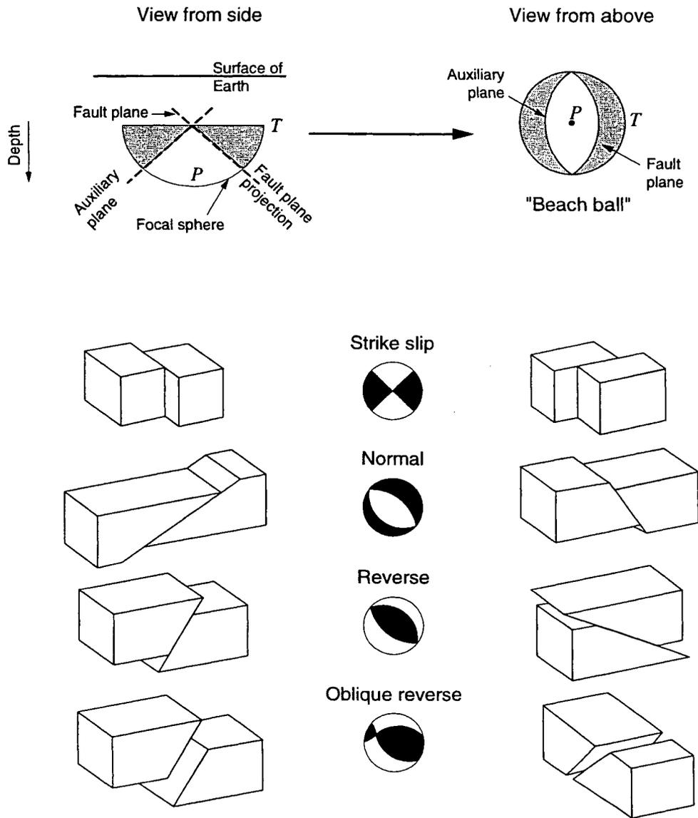
Figure 2.4 Schematic diagram of a focal mechanism. Reprinted from Walter et al., 1996.
