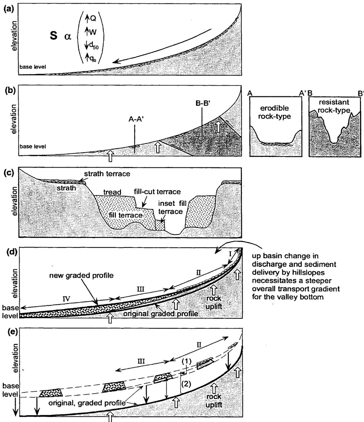
Figure FP.3 Concepts of bedrock channel graded profiles and terrace genesis. a) A graded profile for an alluvial stream develops the familiar concave-up longitudinal profile because discharge and slope are inversely proportional downstream. b) A similar graded profile shape can and does develop for bedrock streams; however, the reach slopes in this profile are delicately adjusted
