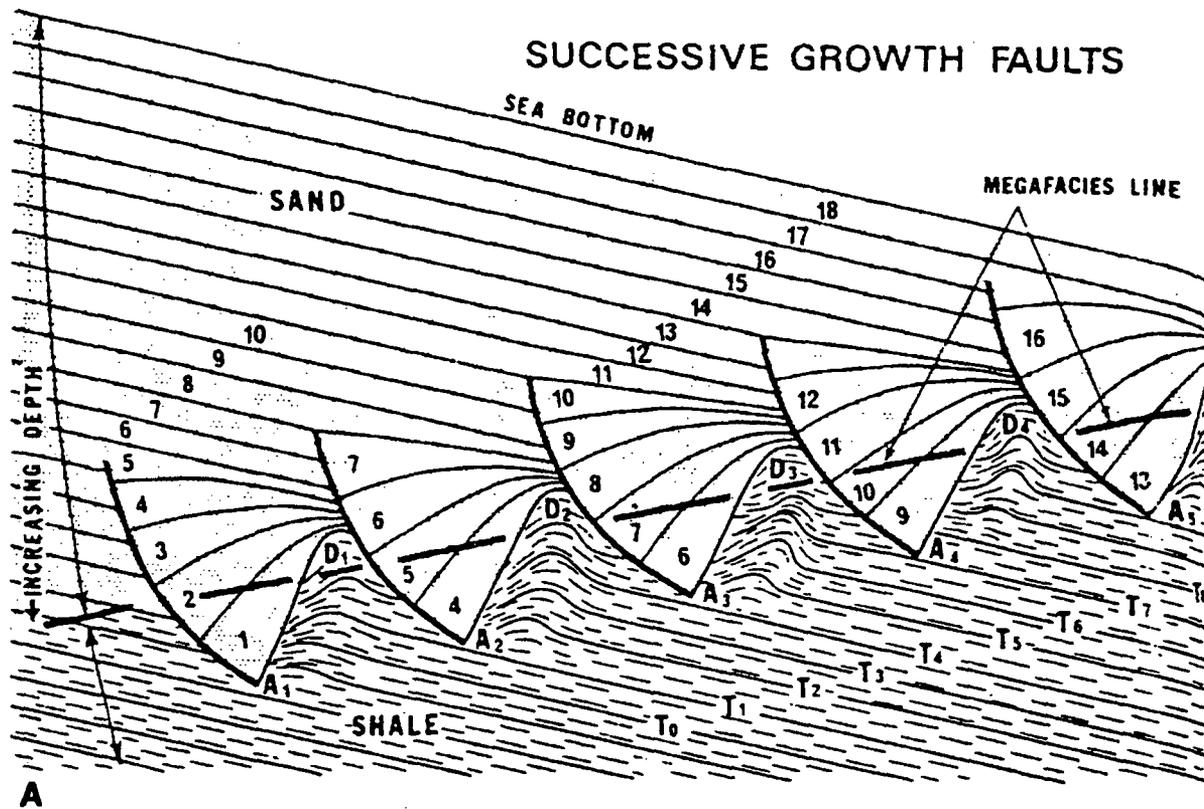
Figure BV.14 Conceptual model for the sequential formation of growth faults during seaward sediment progradation. (H.O. Woodbury, I.B. Murray, Jr., P.J. Pickford, and W.H. Akers, AAPG Bulletin v. 57-12, AAPG © 1973, reprinted by permission of the American Association of Petroleum Geologists).
