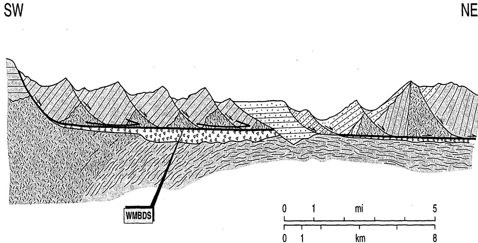
**Figure WC.5** Diagrammatic cross section across the Whipple Mountains of Southeastern California illustrating the Whipple Mountains basal dislocation surface (WMBDS) during middle Miocene. Reprinted with permission from G.A. Davis, *Problems of Intraplate Extensional Tectonics, Western United States, Continental Tectonics, Studies in Geophysics*. Copyright © 1980 by the National Academy of Sciences. Courtesy of the National Academy Press, Washington, D.C.
