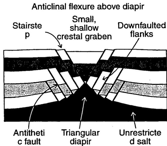
Figure BV.10 Schematic summary of the characteristics of reactive rising diapirs. Reprinted from *Marine and Petroleum Geology*, v. 9, Vendeville and Jackson, *The Fall of Diapirs During Thin-Skinned Extension*, p. 370, © 1992, with permission from Elsevier Science.
