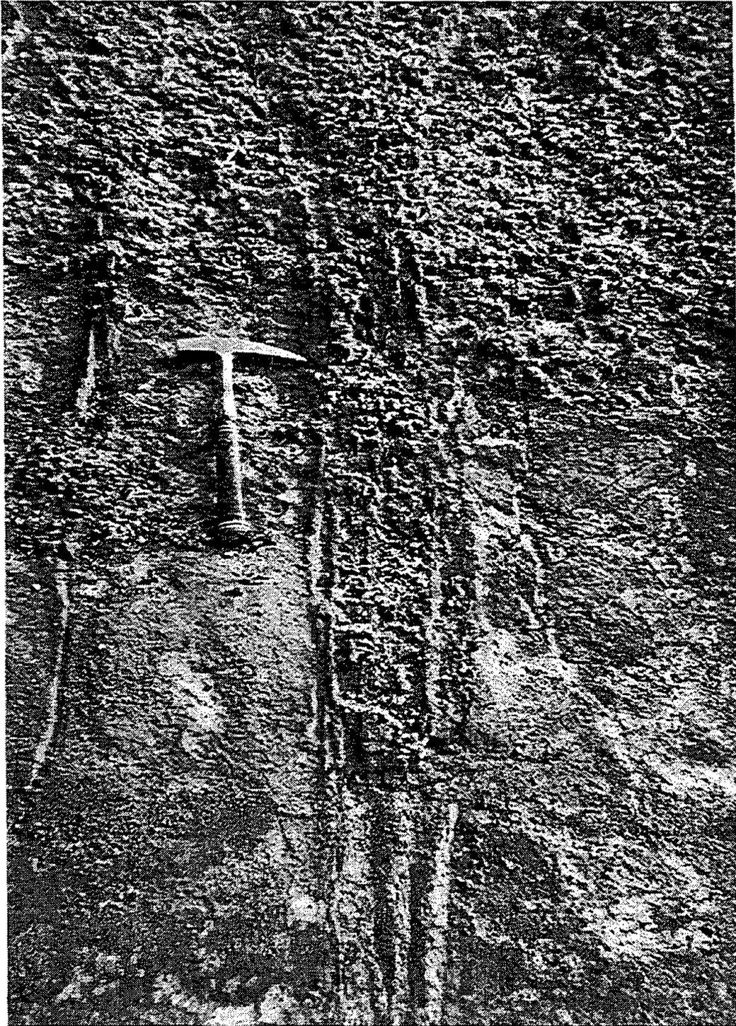
Figure JA.7 Large, structurally controlled cutan, with well developed limonite cemented rinds and vertical internal fabric.
