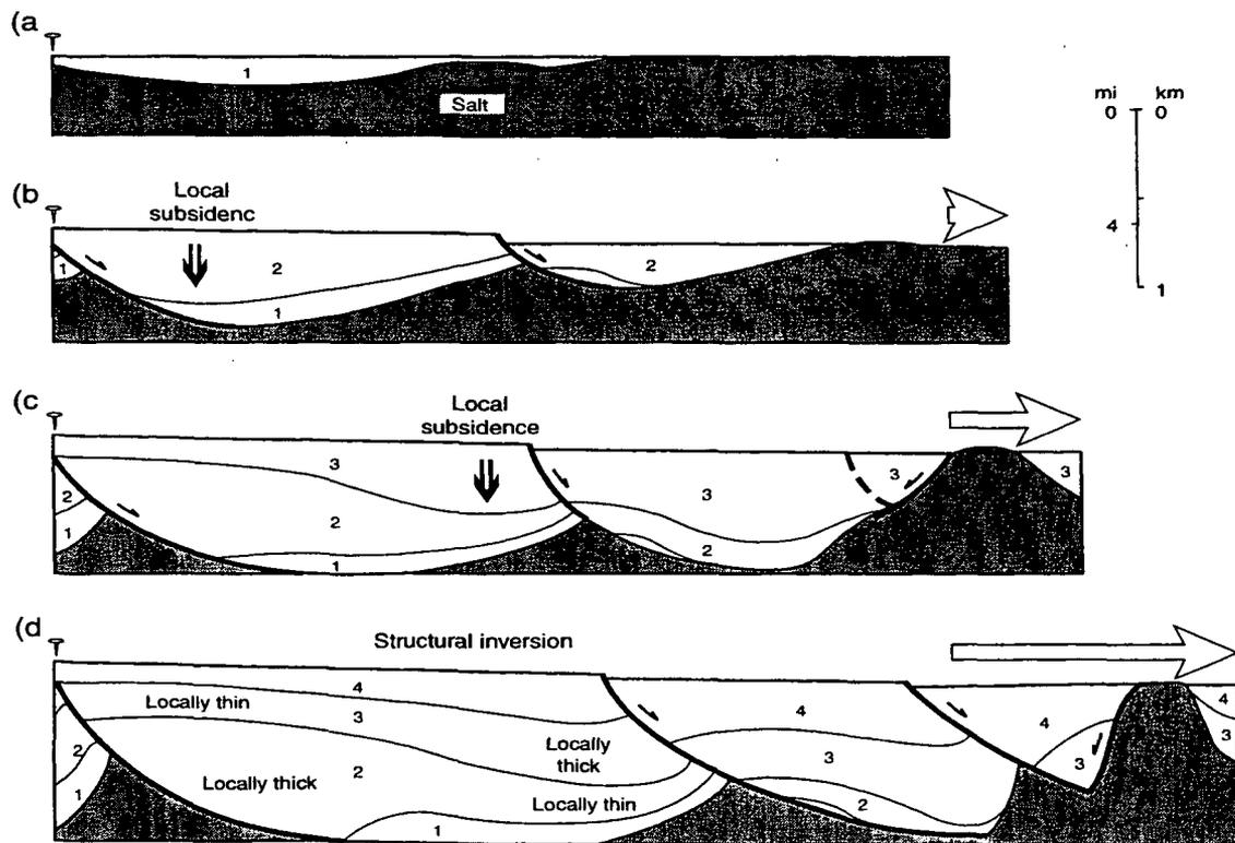
Figure BV.15 Formation of large growth faults above thick salt as a result of thin-skinned extension. Reprinted from Jackson and Talbot (1991), A Glossary of Salt Tectonics, Geological Circular 91-4, with permission from the Bureau of Economic Geology as modified from the Geological Society of America Bulletin, D.M. Worrall, and S. Snelson. Reproduced with permission of the publisher, the Geological Society of America, Boulder, Colorado USA. Copyright © 1989 Geological Society of America.
