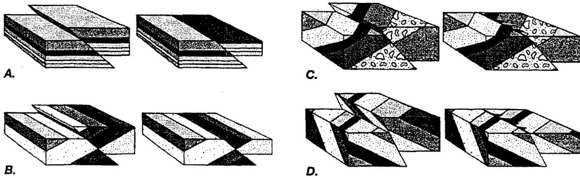
Figure 2.8 The effect of the dip of strata on the separations developed as a result of thrust faulting. The right diagram of each pair shows the hanging wall block eroded down to the same level as the footwall block. On the top surfaces (map views), A. shows a simple discontinuity, B. shows the cutting out of strata, and C. and D. show left and right lateral separations, respectively. faults From: *STRUCTURAL GEOLOGY* by Twiss and Moores © 1992 by W.H. Freeman and Company. Used with permission.
