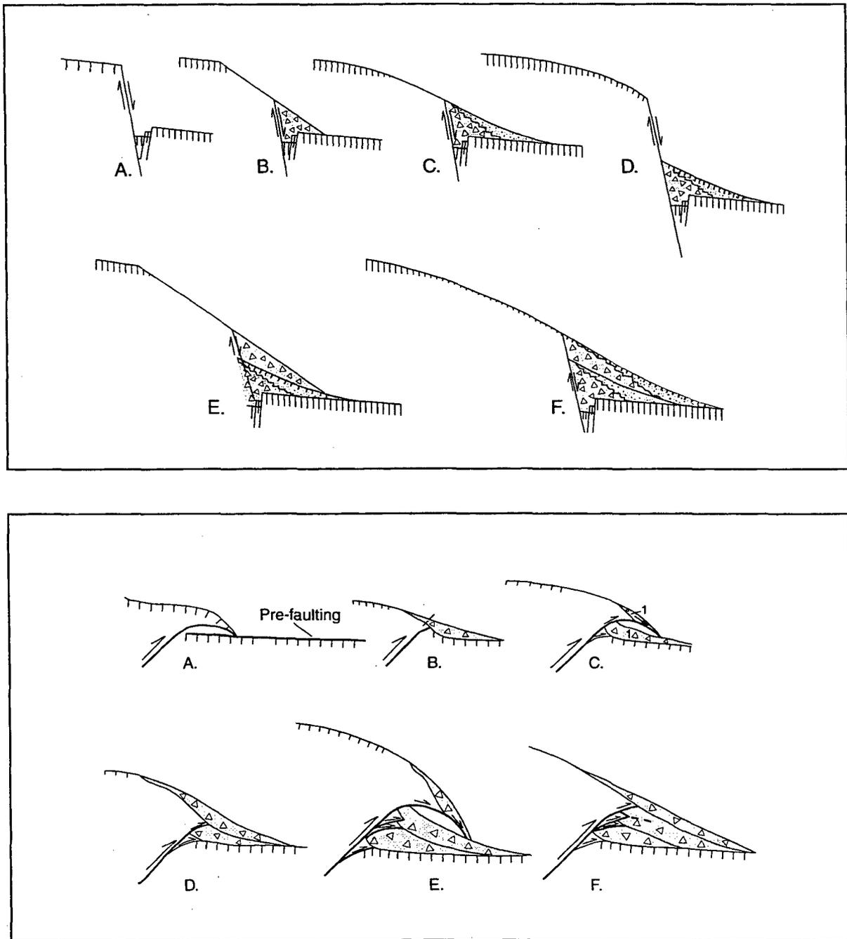
**Figure WC.10** Diagrammatic models of the development of colluvial wedges by repeated ground rupturing of a normal fault (top) and thrust fault (bottom) (Modified from McCalpin, 1987). These same records could be developed by normal faulting along the head of a landslide and thrust faulting at the toe.
