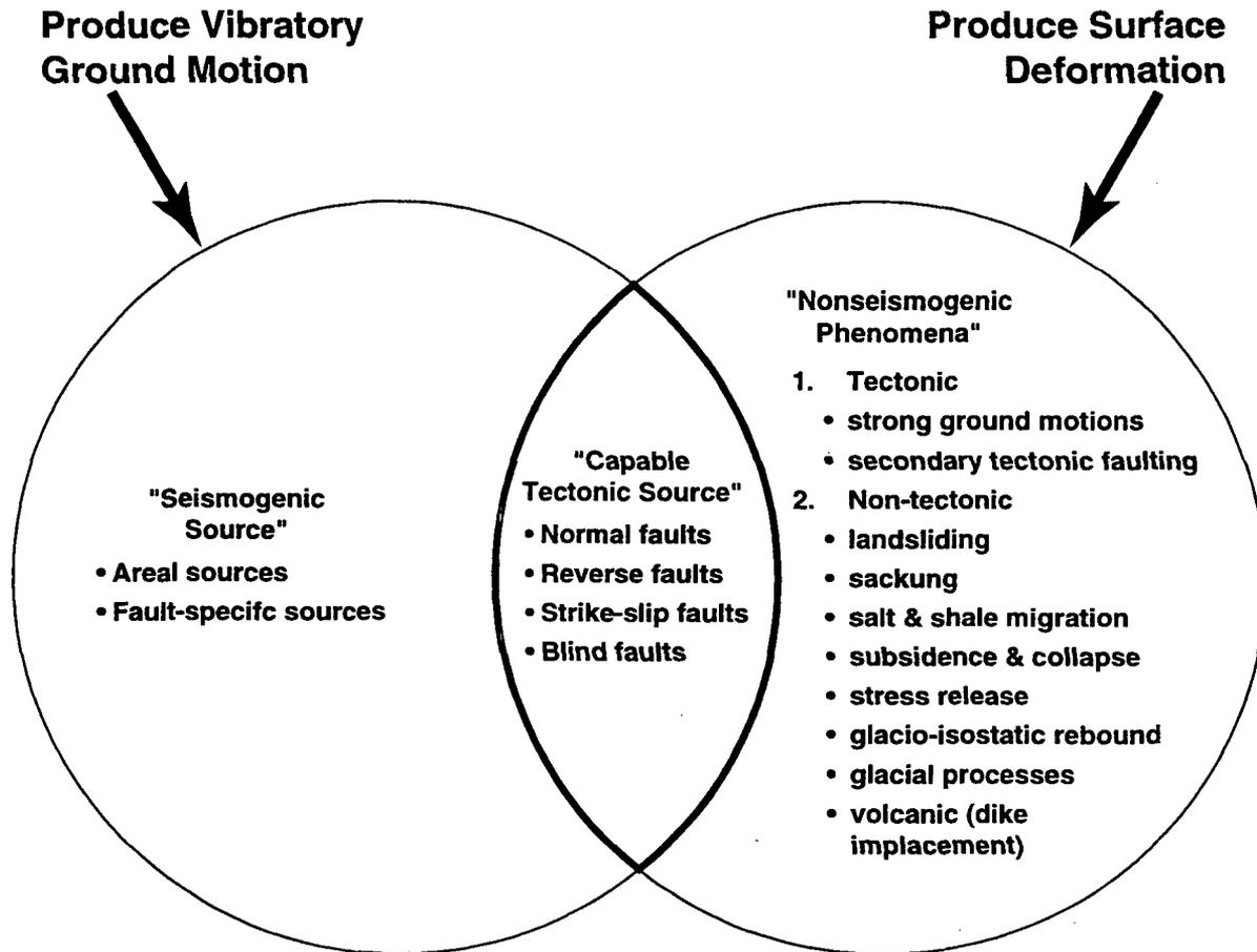
Figure 1.1 Schematic diagram showing the relationship among seismic sources, "seismogenic source," surface deformation, "nonseismogenic phenomena," and "capable tectonic source."
