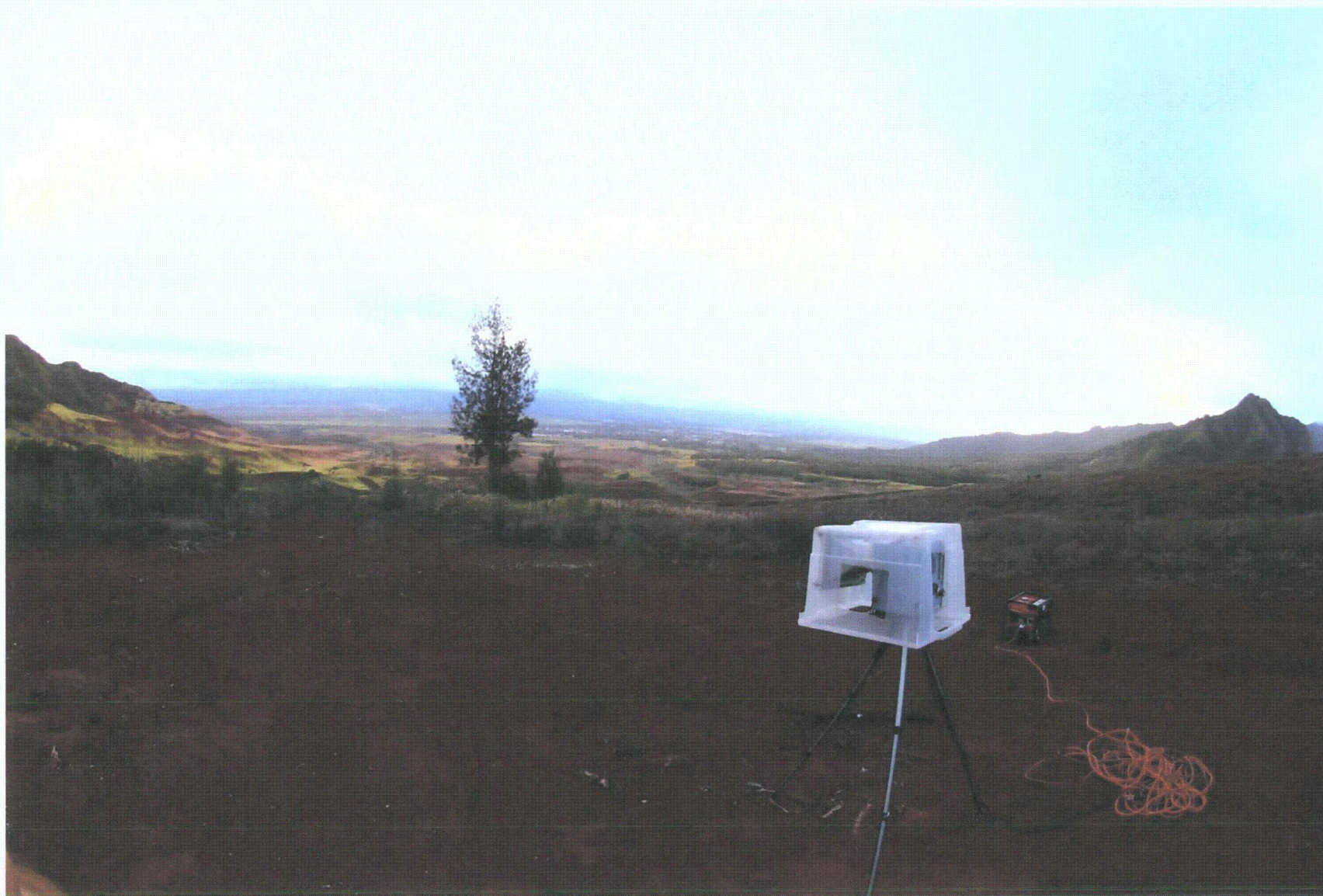
FIGURE 2-2: TYPICAL RANGE BURN AIR SAMPLER SETUP (SAMPLER PT4)
