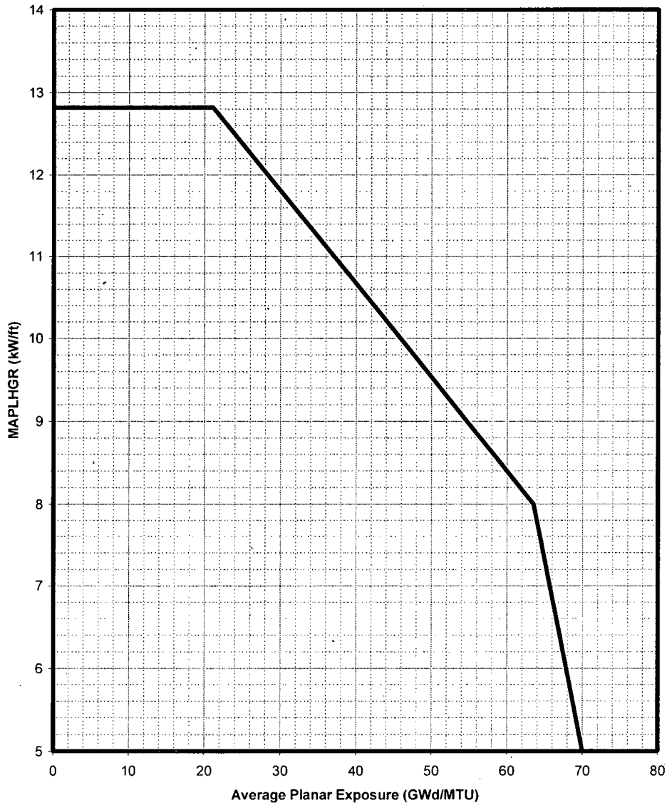
FIGURE 12. MAXIMUM AVERAGE PLANAR LINEAR HEAT GENERATION RATE (MAPLHGR) VERSUS AVERAGE PLANAR EXPOSURE FOR GE14
