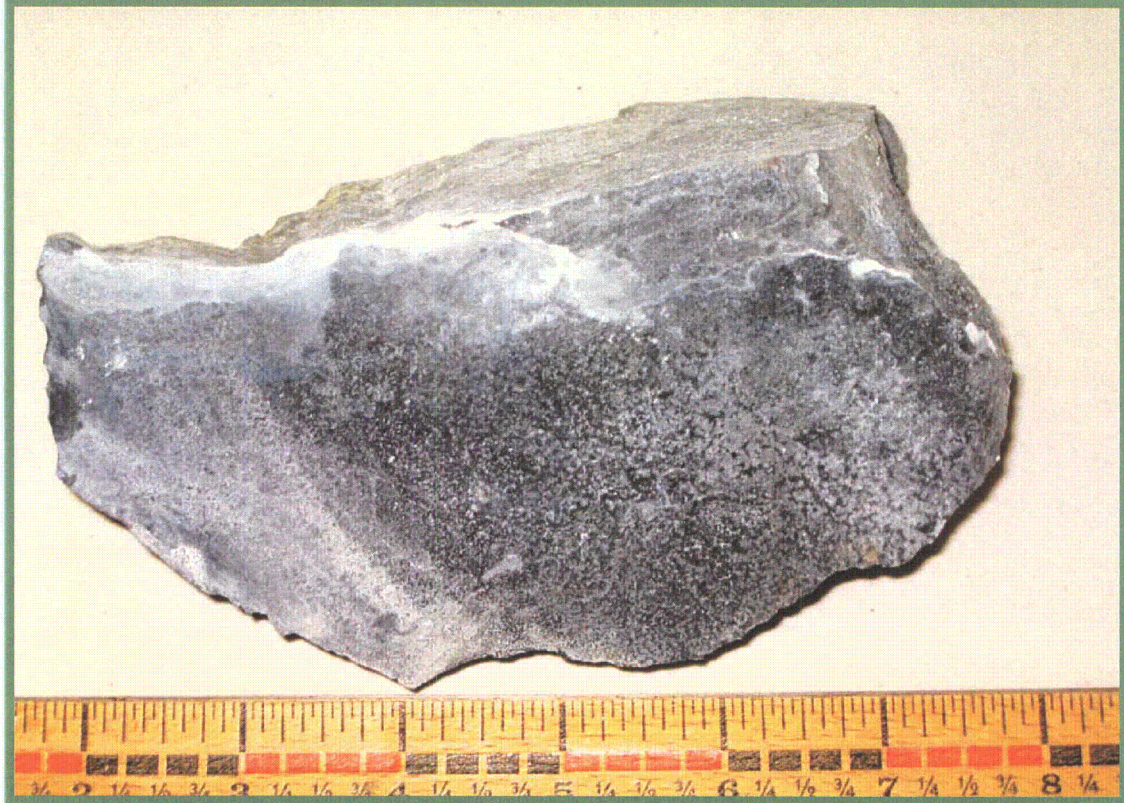
Sample 4-72 Light grey to grey fine-grained slag, trace vesicles to dense/solid, lightly to moderately fractured, slight secondary mineralization along fracture lines.
