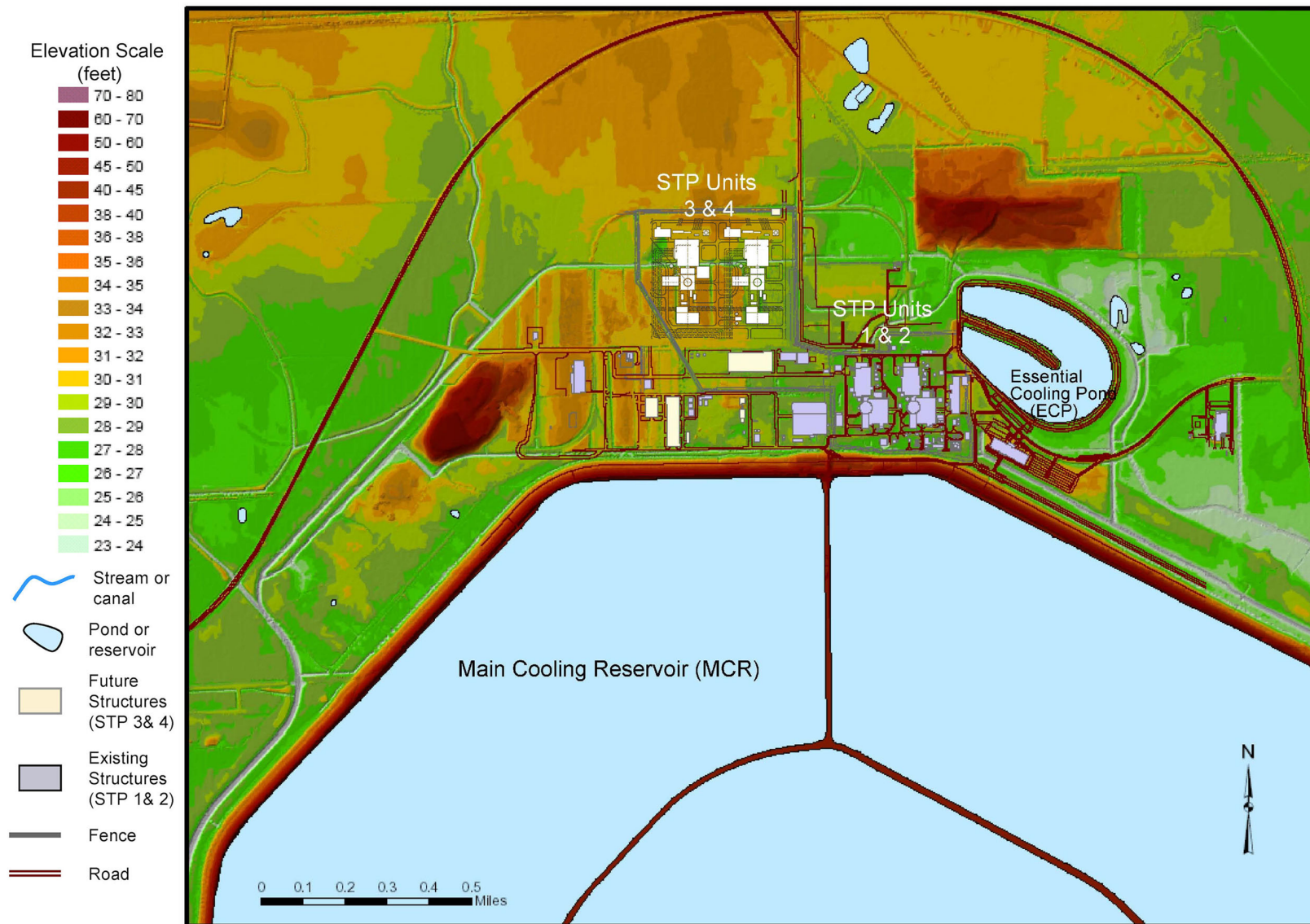
Figure 2.4S.1-3 Existing (Pre-Development) Topography and Major Structures at STP 3 & 4
