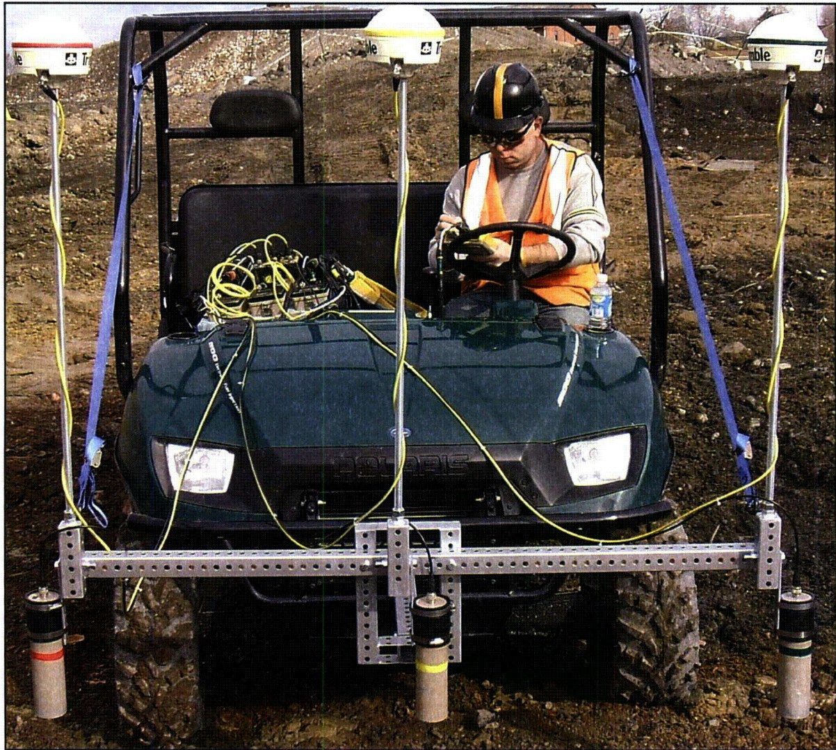
Figure 6.1-1: Example of Best Technology Available Utilized for the Roving Gamma Survey at the Dewey-Burdock Project by ERG.
