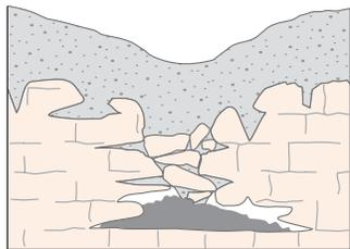
The slow, downward erosion eventually forms small surface depressions 1 inch to several feet in depth and diameter.
