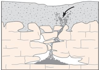
A column of overlying sediments settles into the vacated spaces (a process termed "piping" or "raveling").
