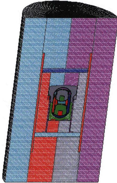
Figure 2-261. Finite Element Mesh for the SC-2, End Impact, 0° Support Structure
